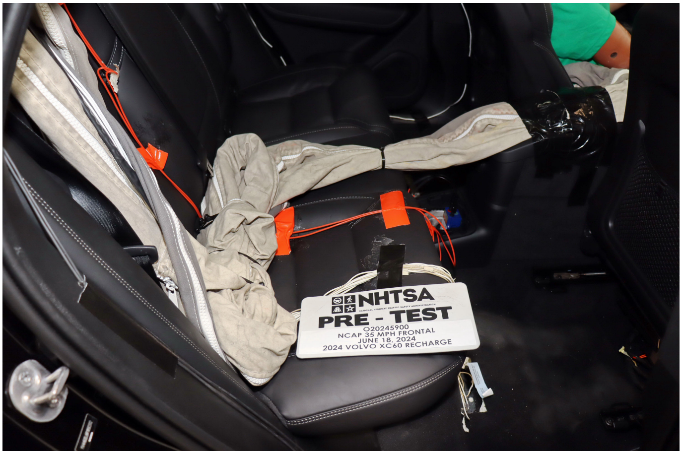
Photo No. 028 - Pre-Test Dummy Cable Routing
