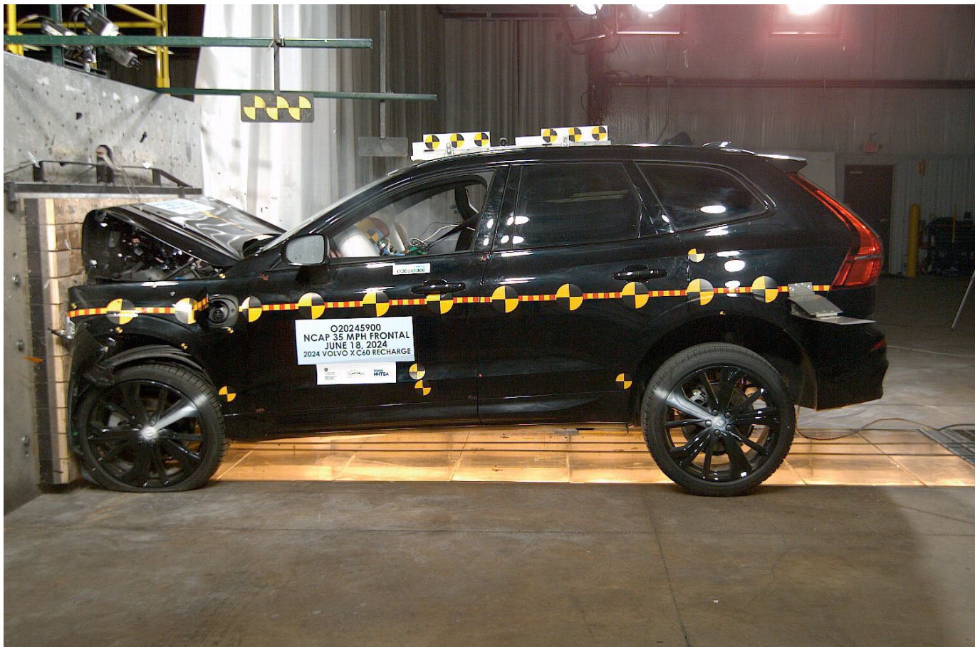
Photo No. 082 - 2024 Volvo XC60 Recharge AWD Ultimate 5-Door SUV Frontal Impact Event
