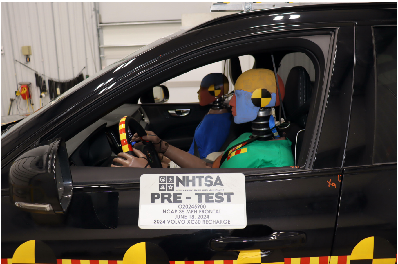
Photo No. 032 - Pre-Test Driver Dummy Window View
