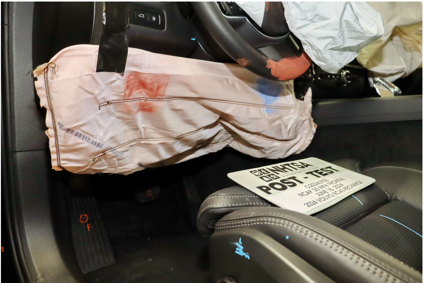
Photo No. 045 - Post-Test Driver's Side Knee Bolster
