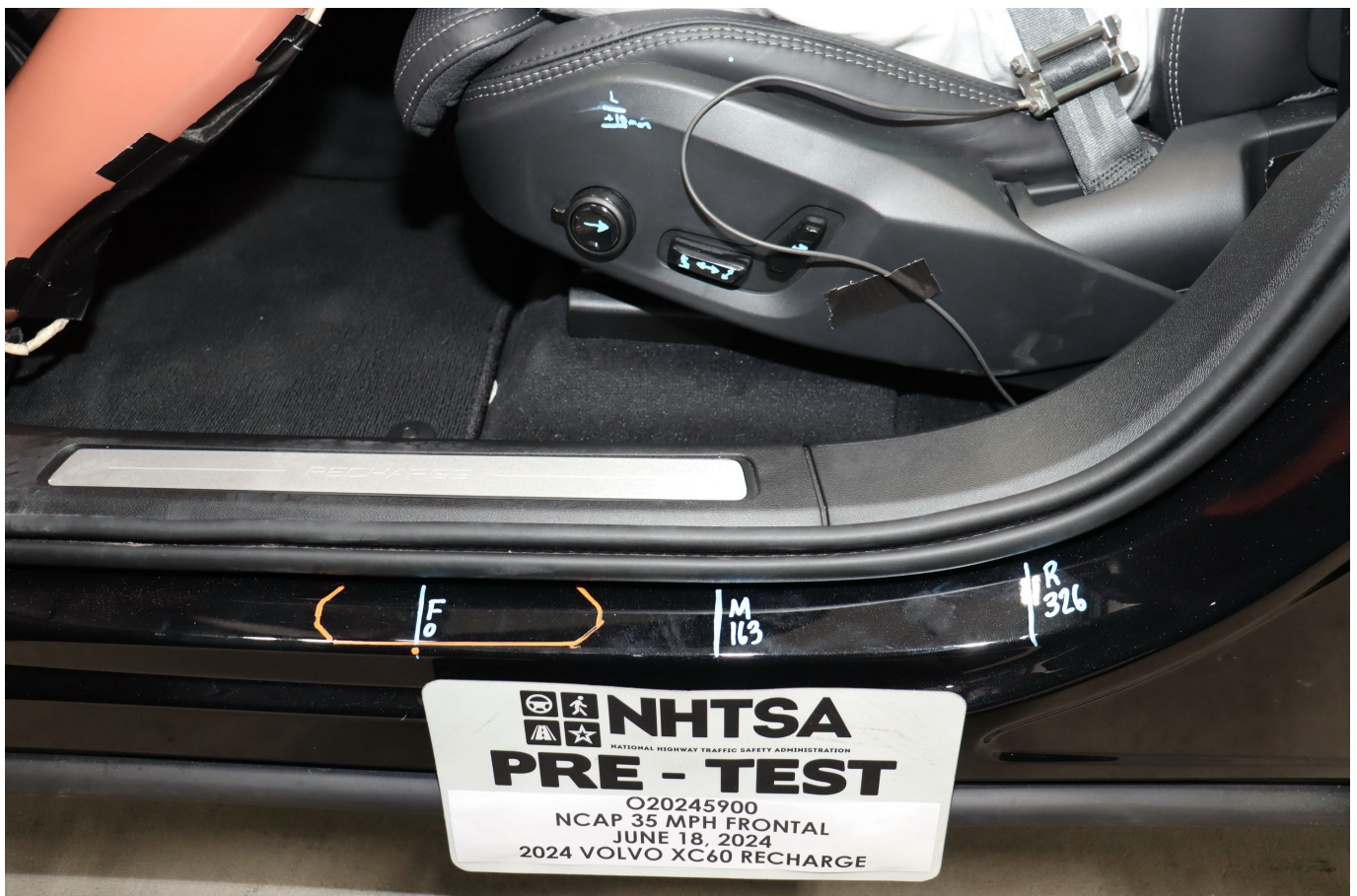
Photo No. 036 - Pre-Test Driver's Seat Fore-Aft Markings
