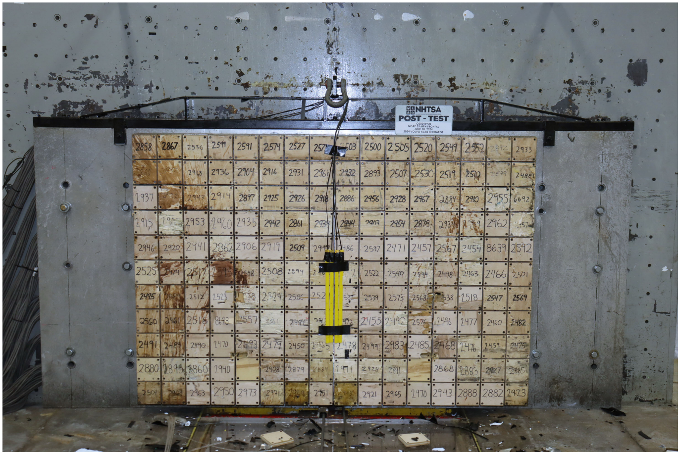
Photo No. 003 - Post-Test Load Cell Wall
