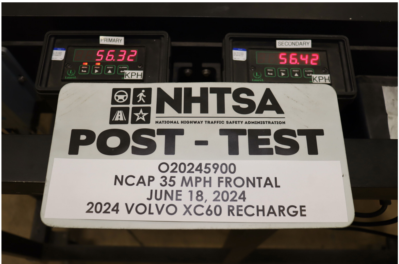
Photo No. 076 - Post-Test Speed Trap Read-Out
