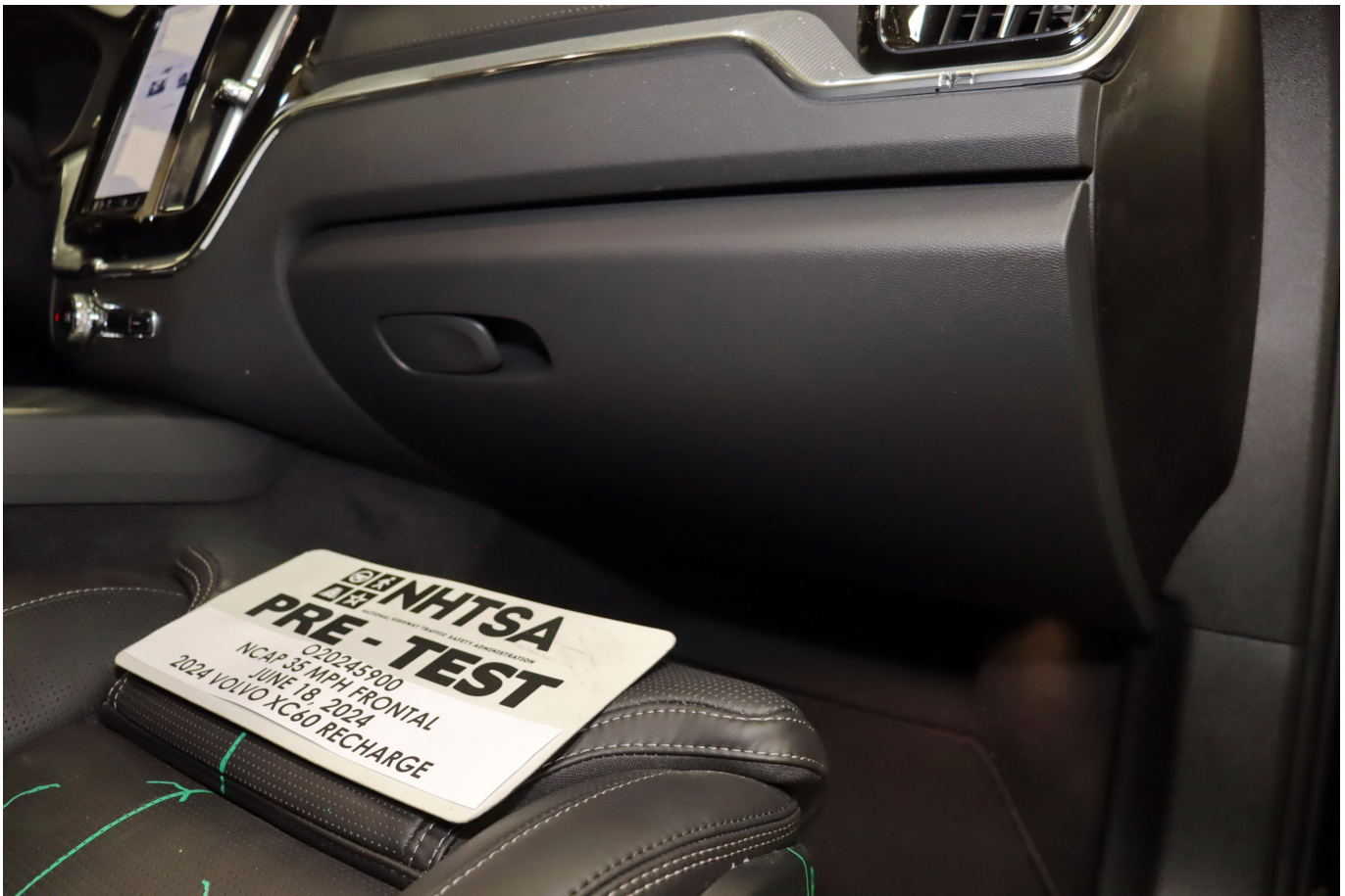
Photo No. 067 - Pre-Test Passenger's Side Knee Bolster
