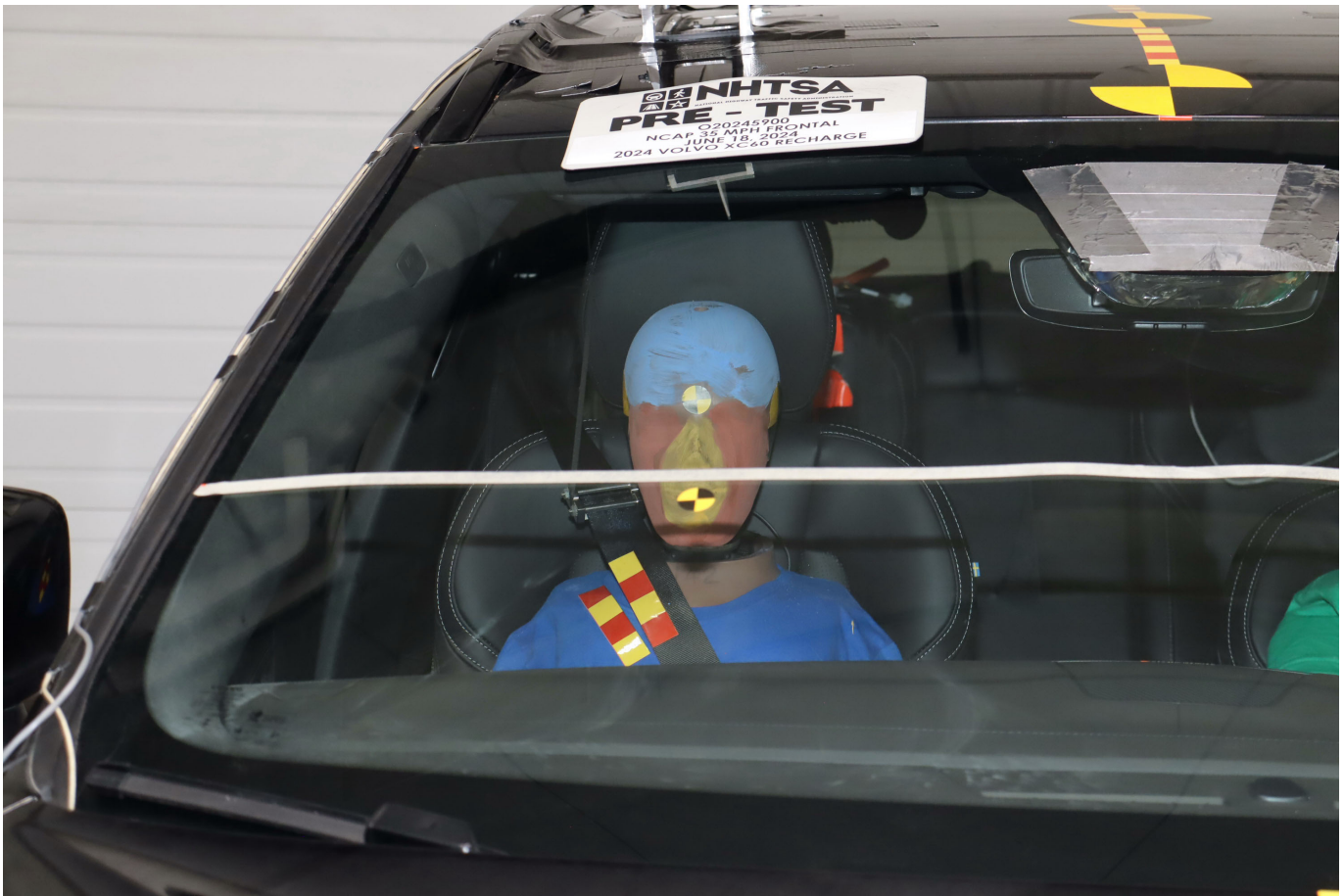
Photo No. 053 - Pre-Test Passenger Dummy Front View
