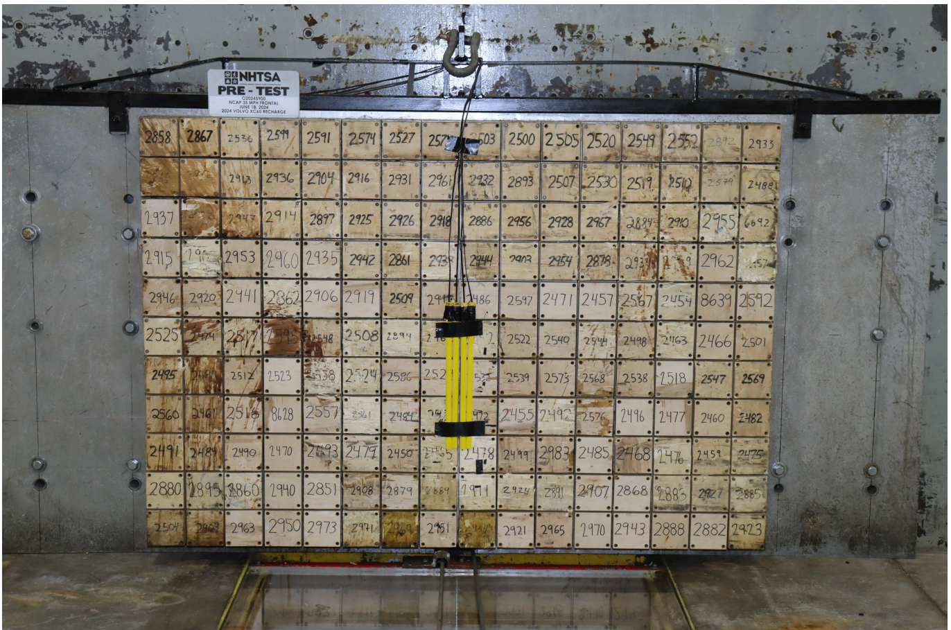
Photo No. 002 - Pre-Test Load Cell Wall
