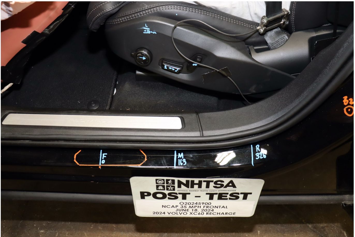
Photo No. 037 - Post-Test Driver's Seat Fore-Aft Markings
