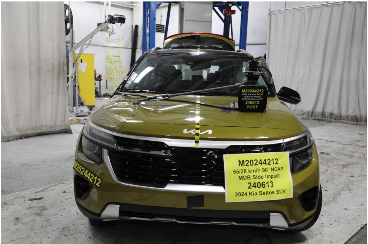
004 Post-Test Frontal View of Test Vehicle
