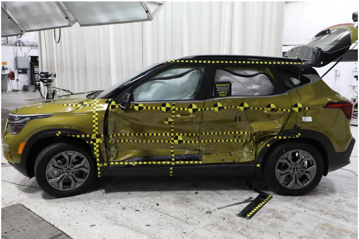
008 Post-Test Left Side View of Test Vehicle
