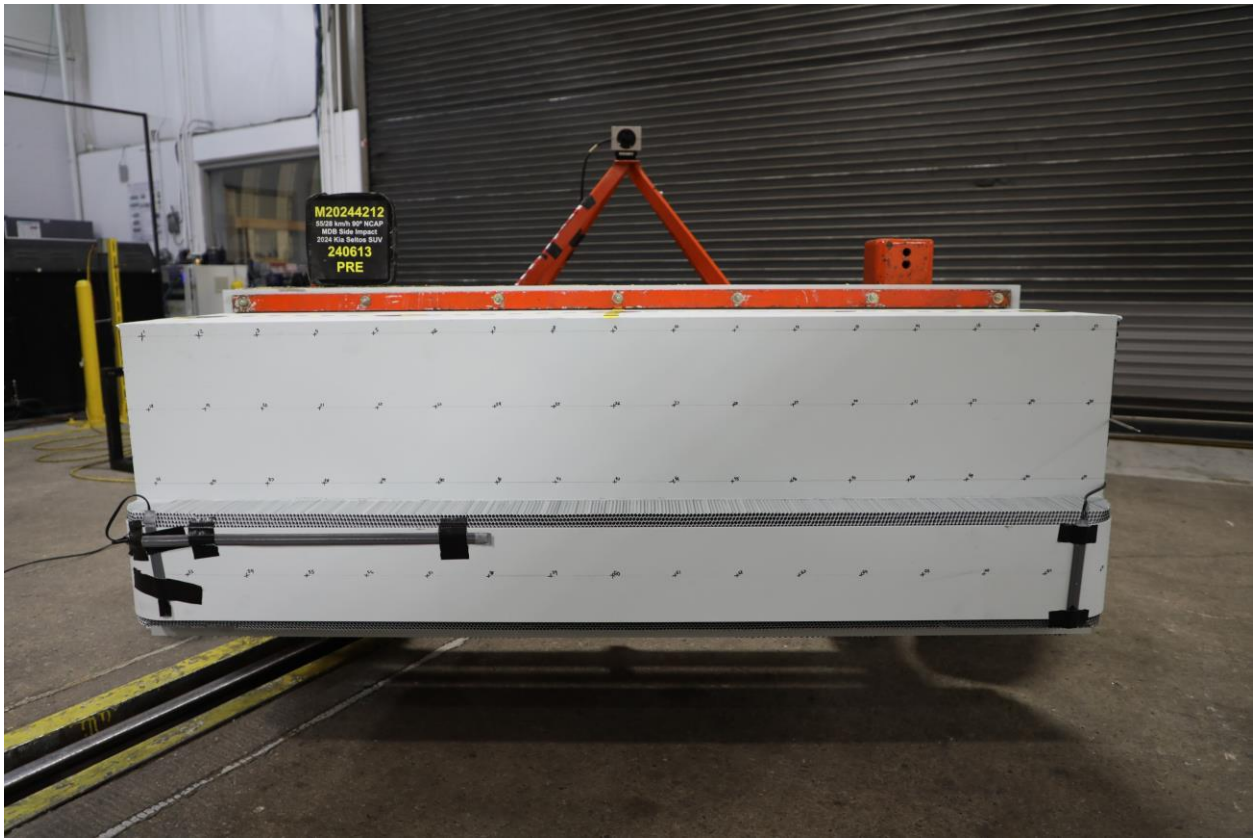
084 Pre-Test Front View of MDB Impactor Face
