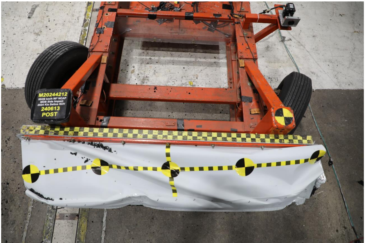
087 Post-Test Top View of MDB Impactor Face
