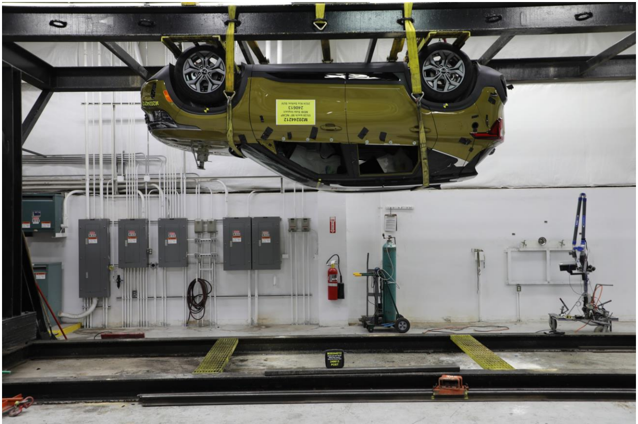
098 FMVSS No. 301 Static Rollover 180 Degrees
