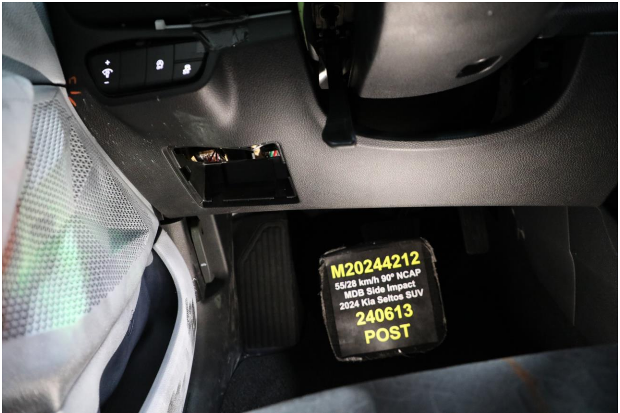
054 Post-Test Driver Dummy Close-Up Knee Contact View
