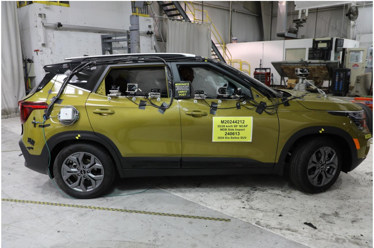
014 Post-Test Right Side View of Test Vehicle
