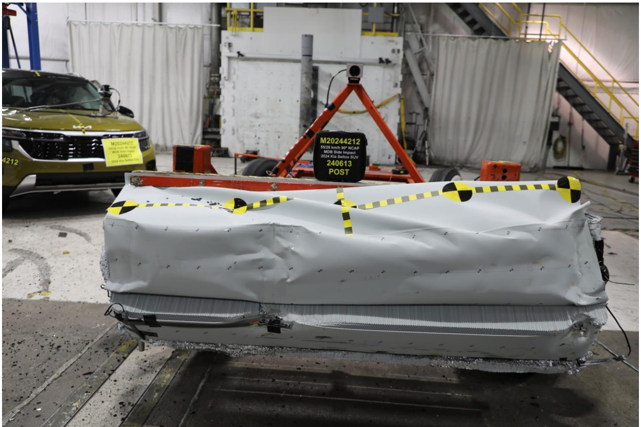
085 Post-Test Front View of MDB Impactor Face
