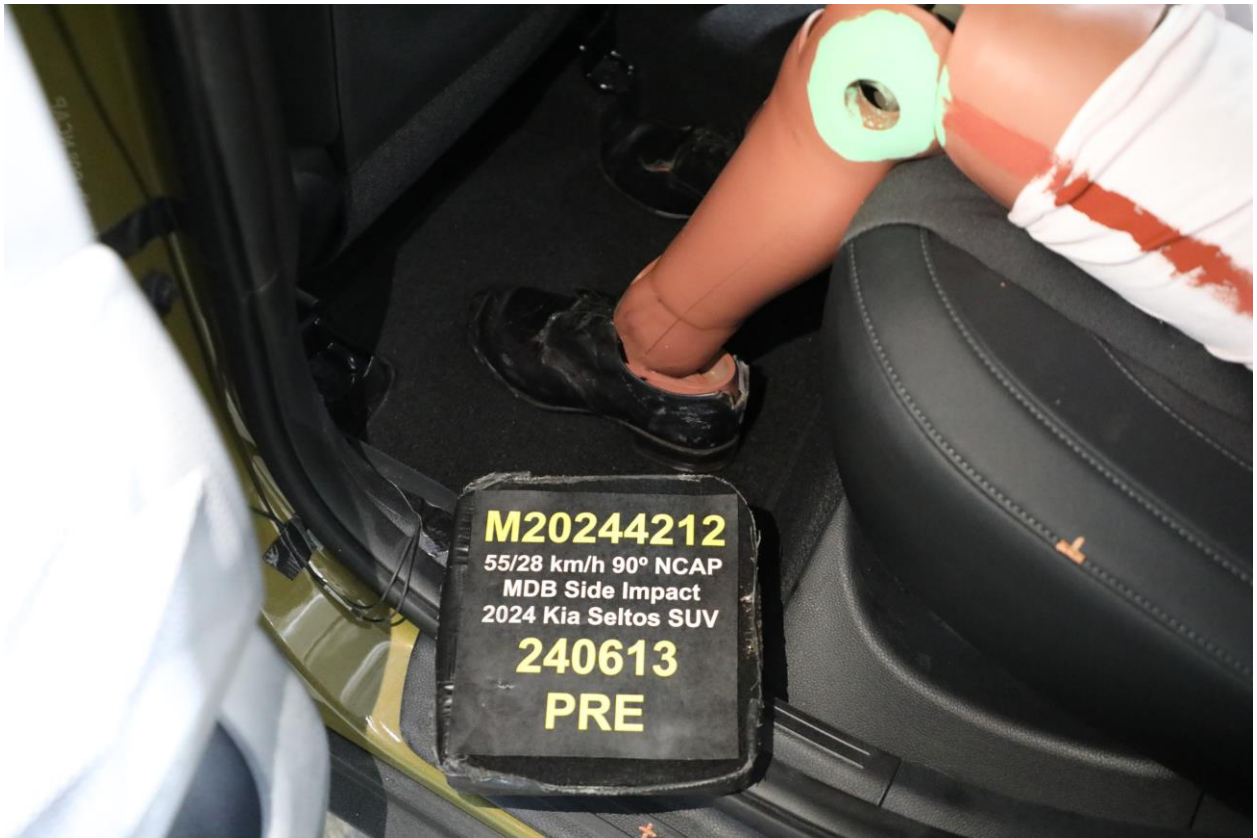
064 Pre-Test Placement of Rear Passenger Dummy's Feet
