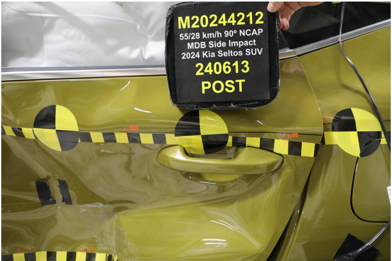
024 Post-Test Left Rear Door Latch Close-Up
