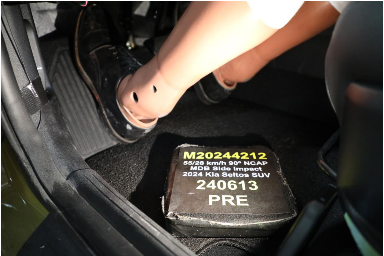
034 Pre-Test Placement of Driver's Dummy Feet
