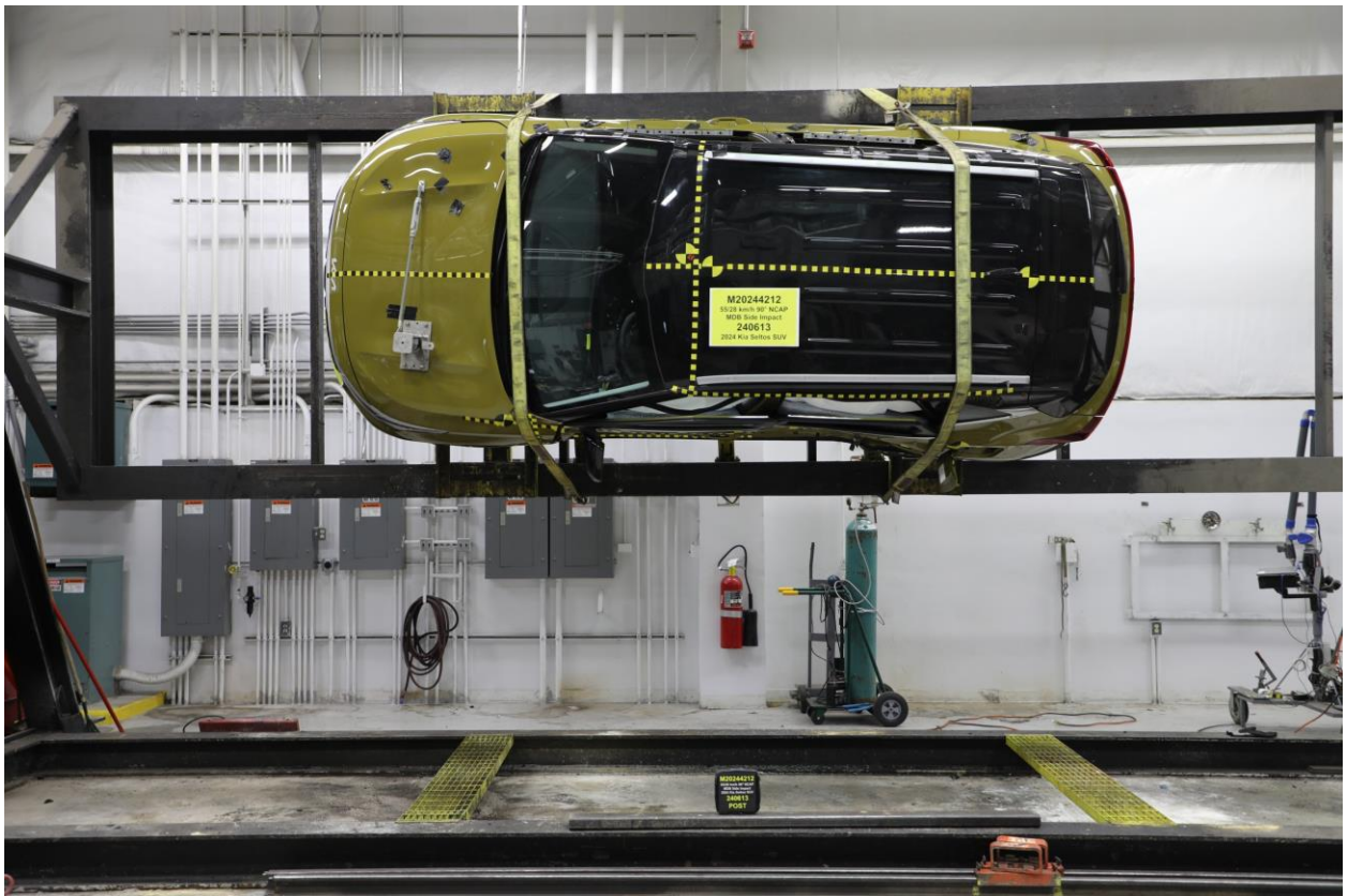
097 FMVSS No. 301 Static Rollover 90 Degrees
