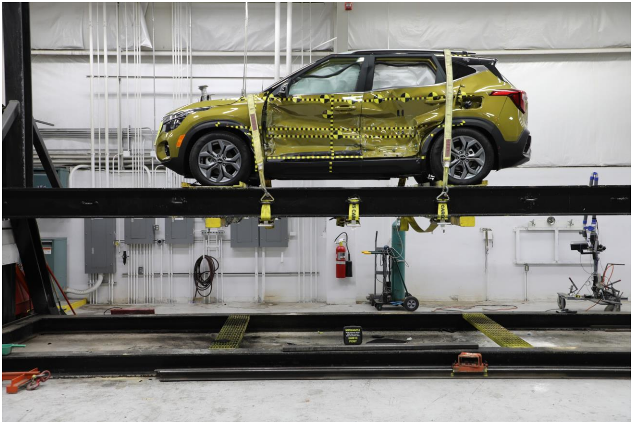
100 FMVSS No. 301 Static Rollover 360 Degrees
