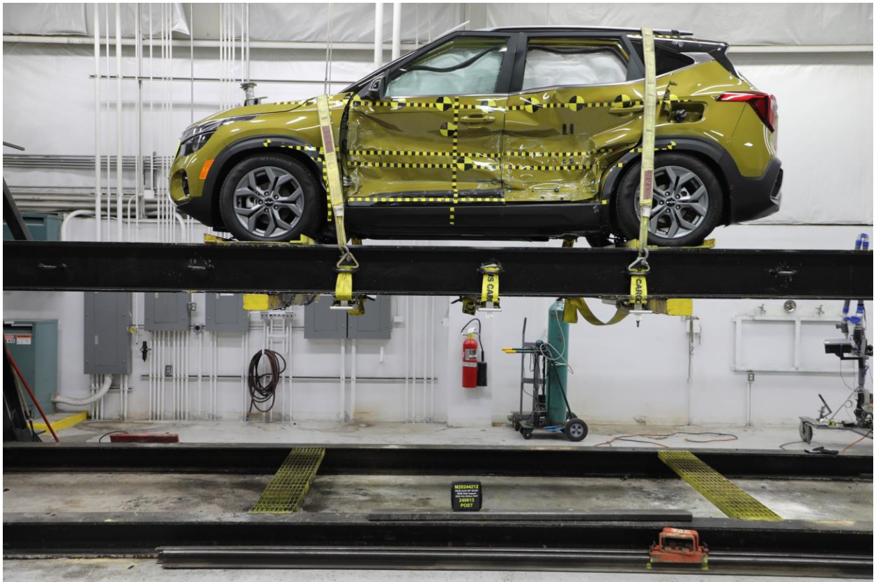
096 FMVSS No. 301 Static Rollover 0 Degrees
