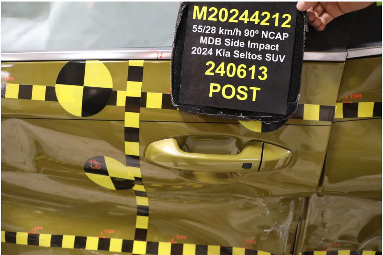
022 Post-Test Left Front Door Latch Close-Up
