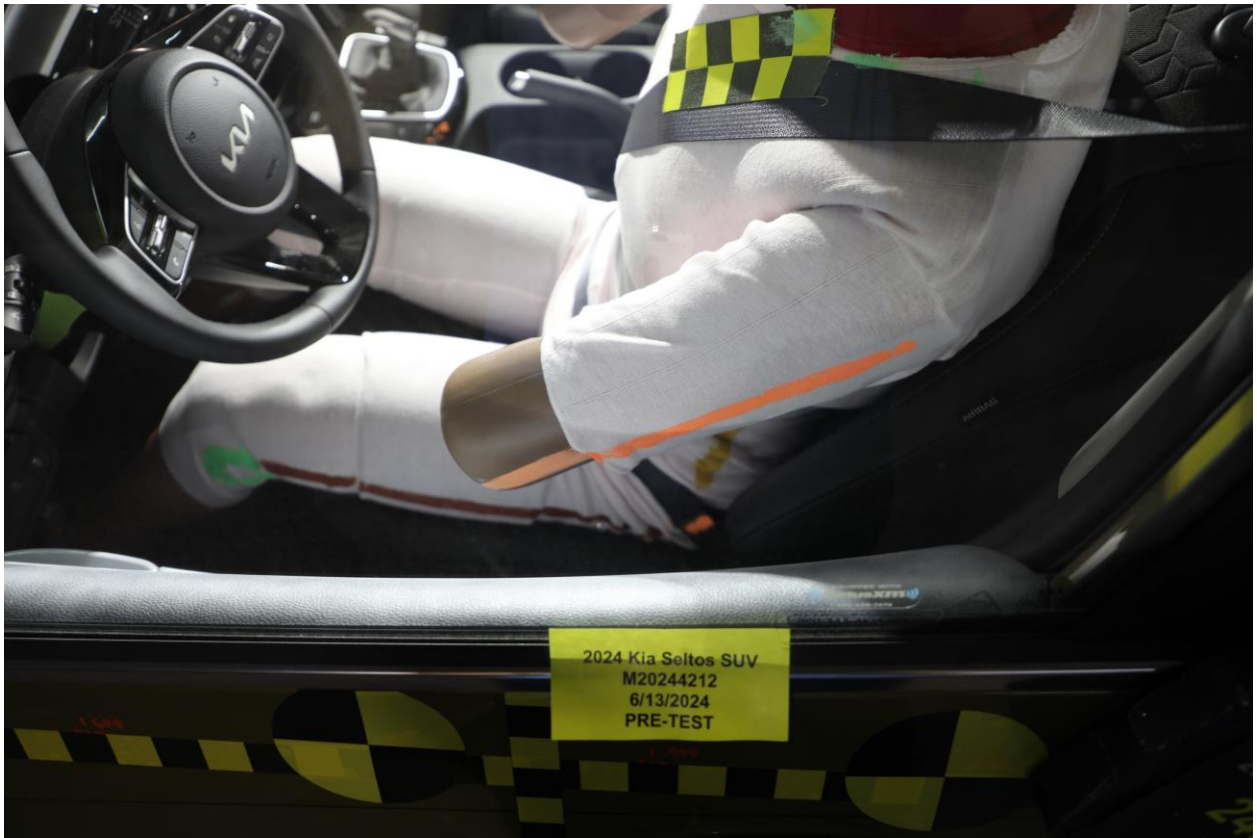
042 Pre-Test Driver Dummy and Door Clearance View
