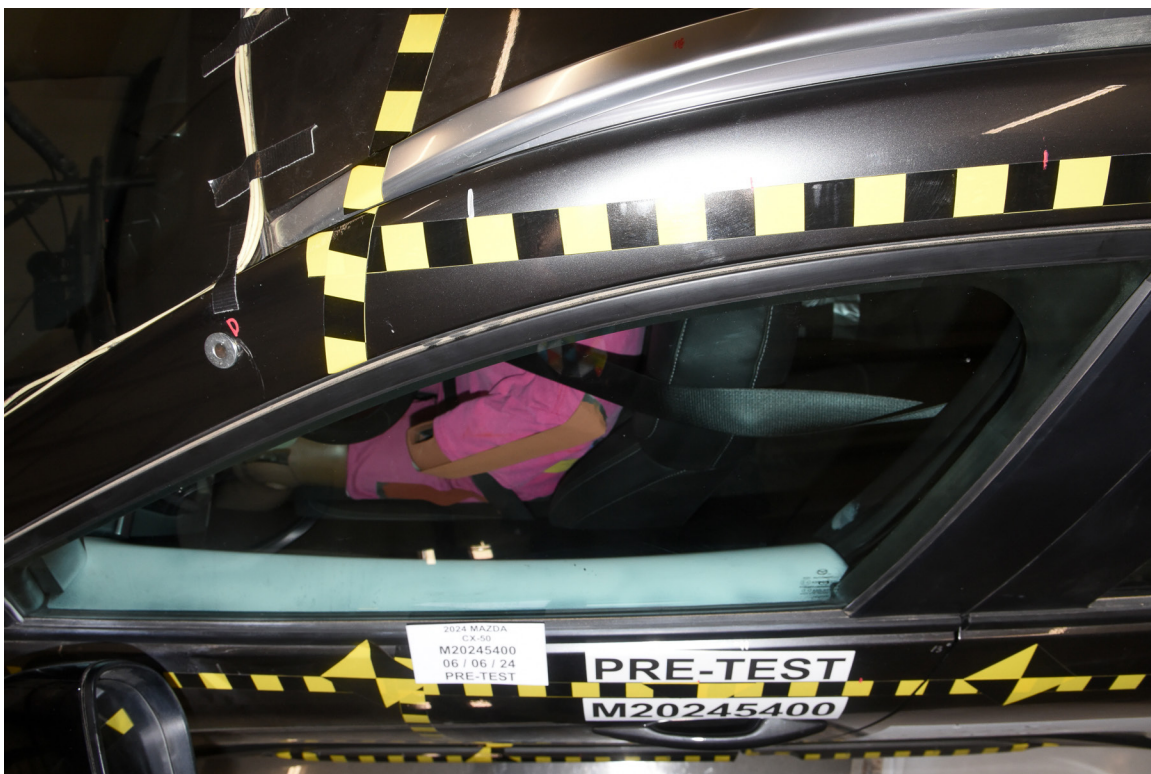
FIGURE 40. Pre-Test Dummy and Door Clearance View
