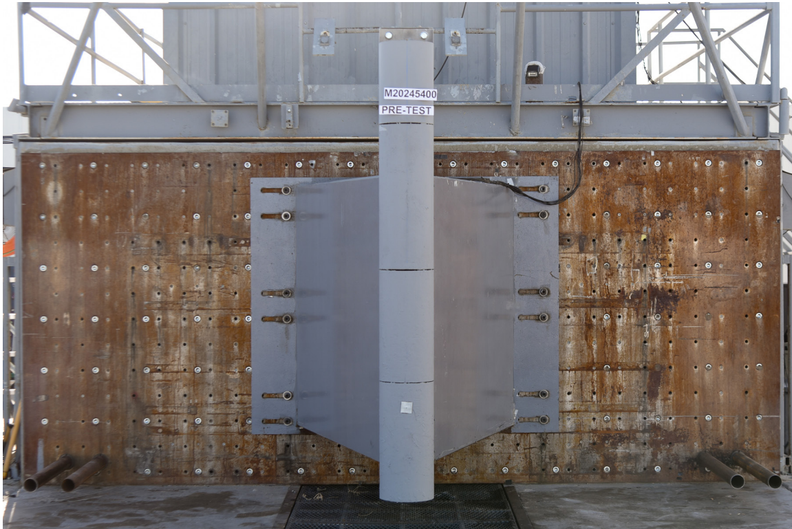
FIGURE 59. Pre-Test Pole Barrier Front View
