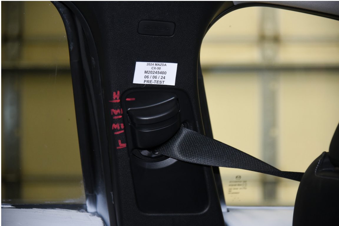
FIGURE 33. Pre-Test View of Belt Anchorage for Dummy
