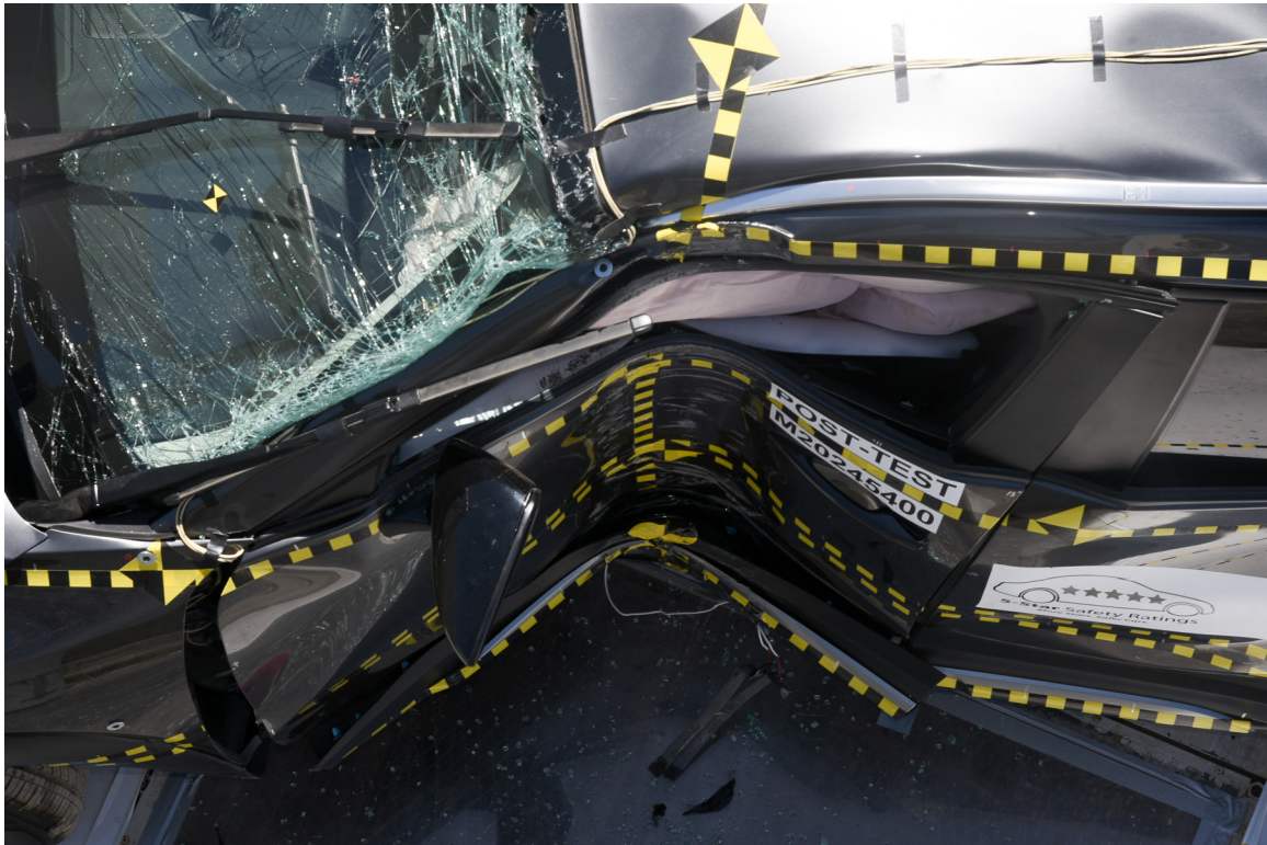
FIGURE 41. Post-Test Dummy and Door Clearance View
