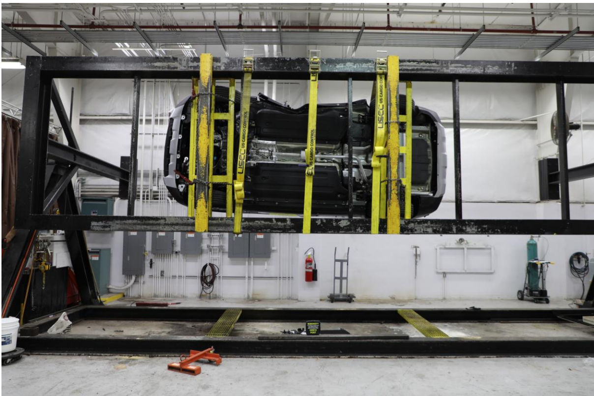
No. 068 FMVSS No. 301 Static Rollover 270 Degrees
