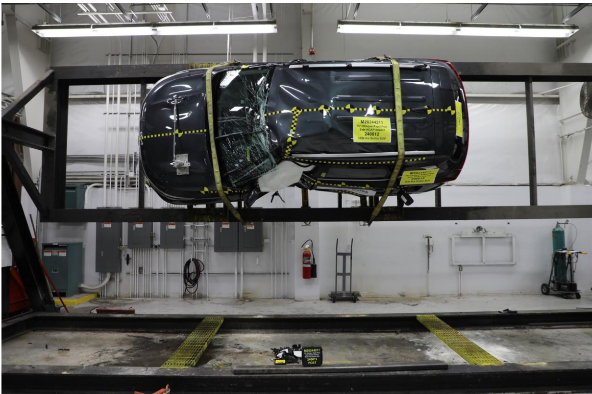
No. 066 FMVSS No. 301 Static Rollover 90 Degrees
