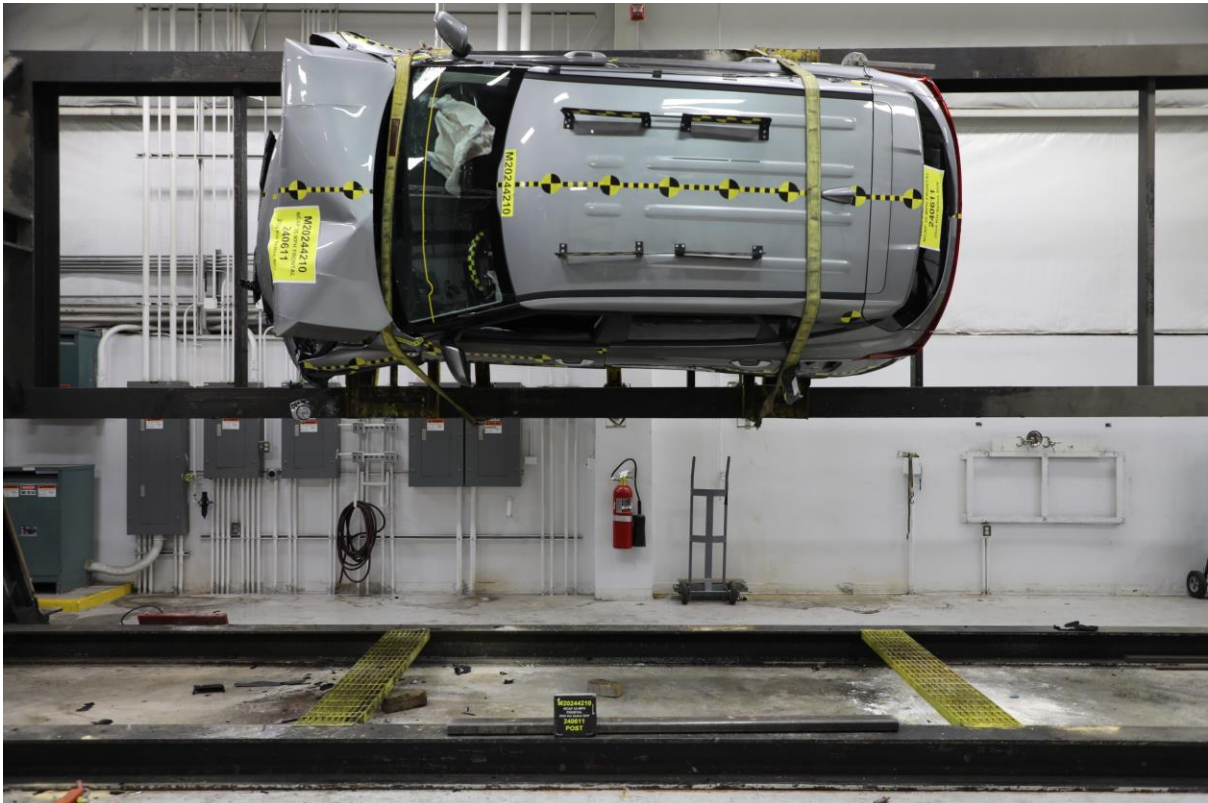
078 Vehicle at 90° on Static Rollover Device
