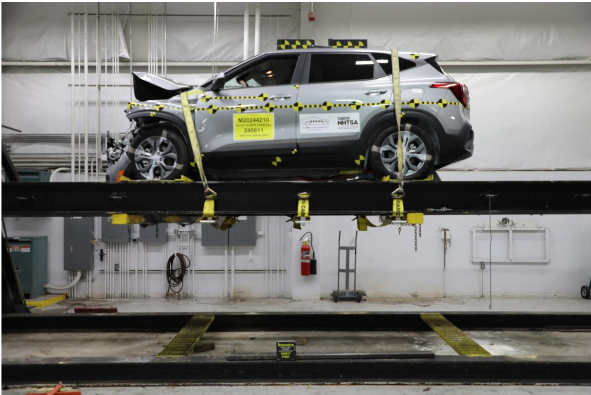
077 Vehicle at 0° on Static Rollover Device
