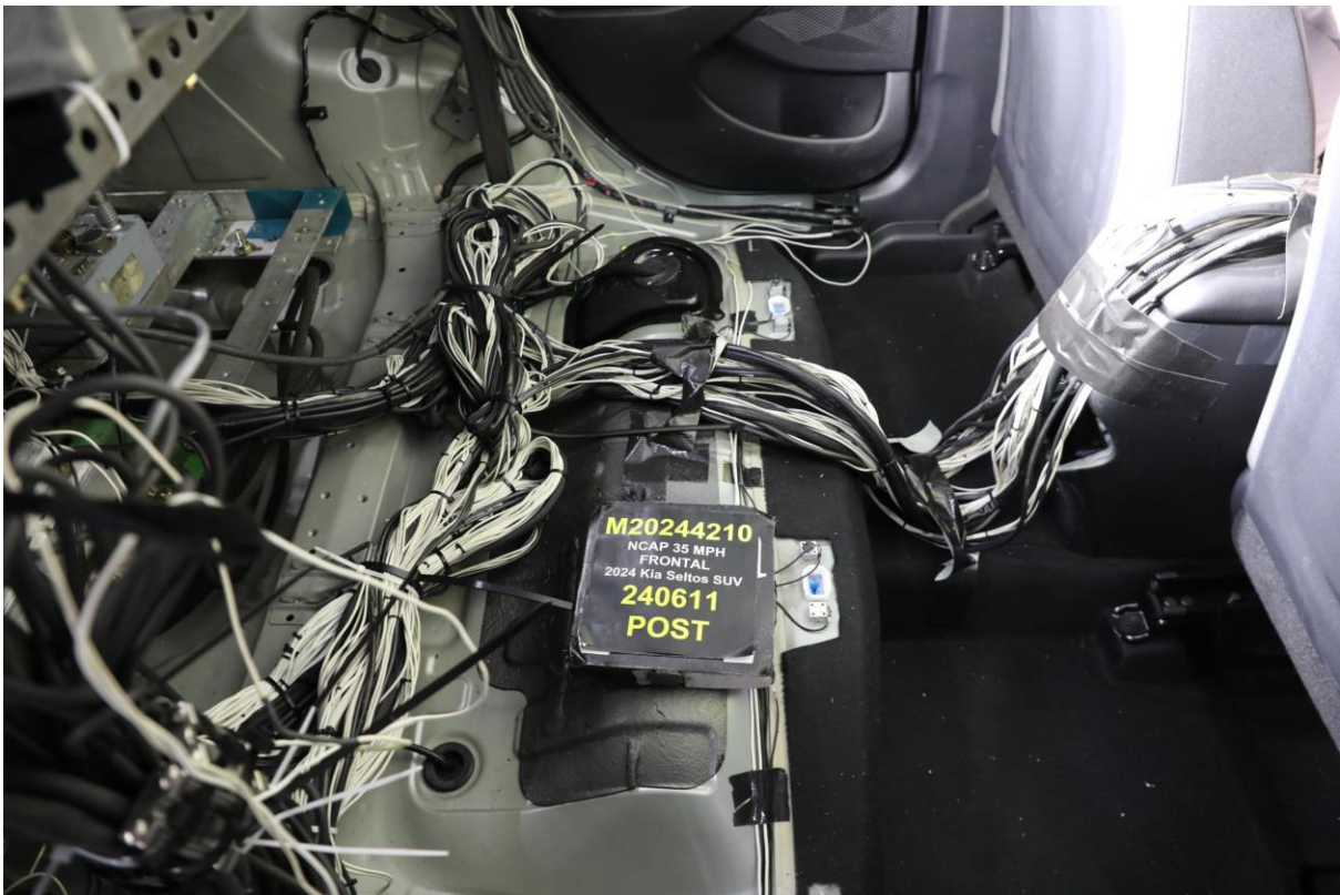
029 Post-Test Dummy Cable Routing
