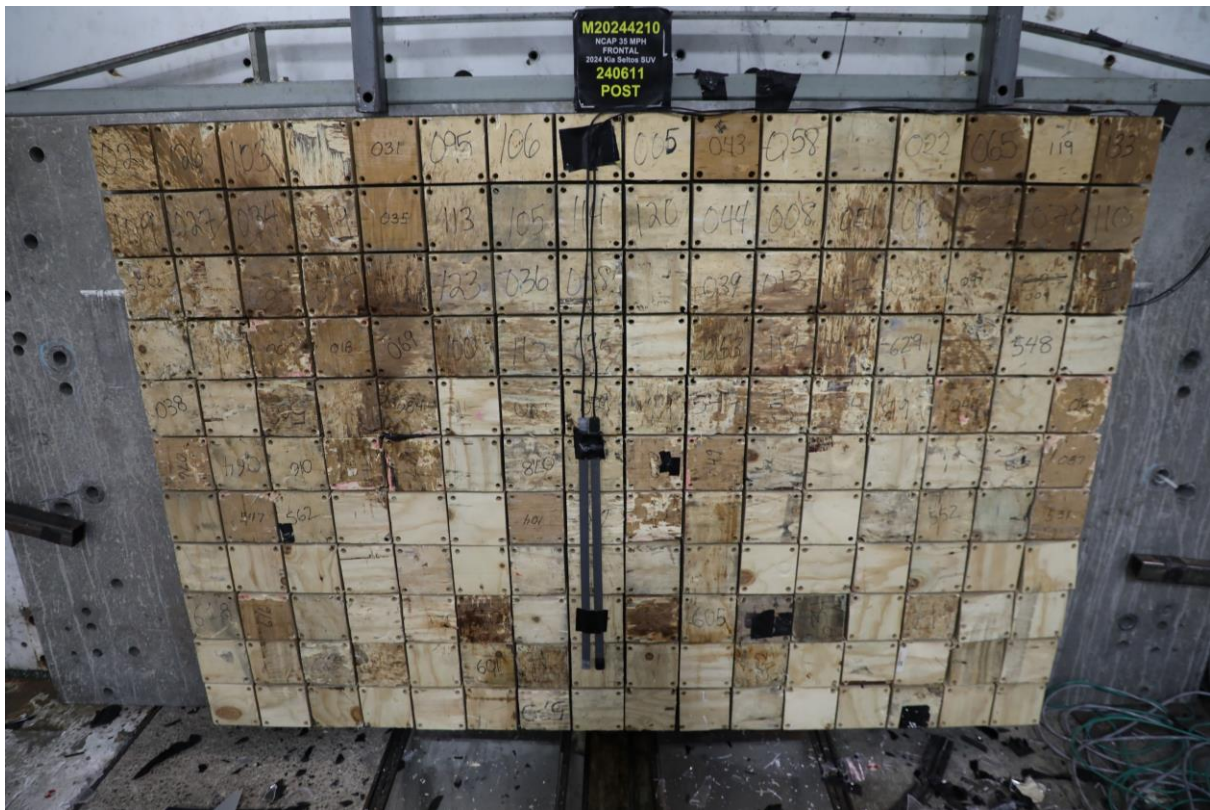
003 Post-Test Load Cell Wall
