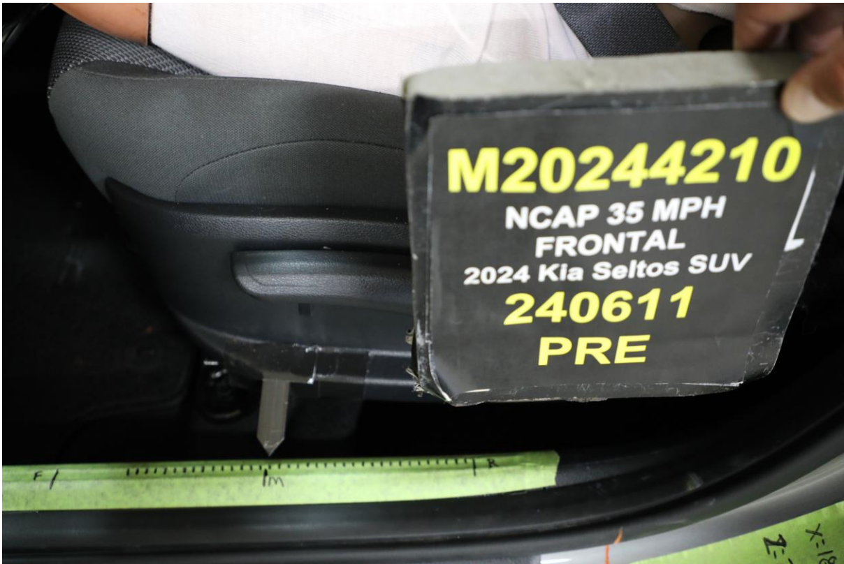
036 Pre-Test Driver's Seat Fore-Aft Markings
