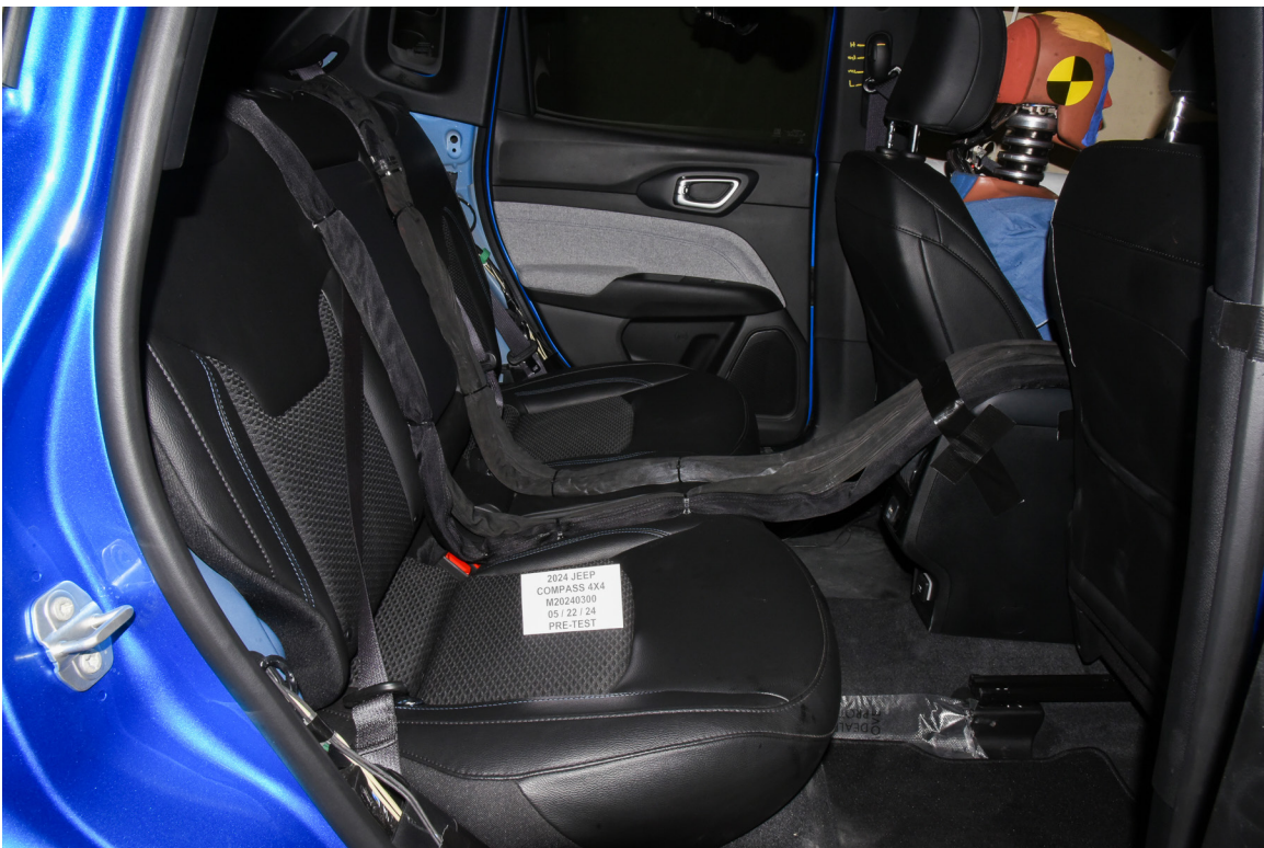
FIGURE 28. Pre-Test Dummy Cable Routing
