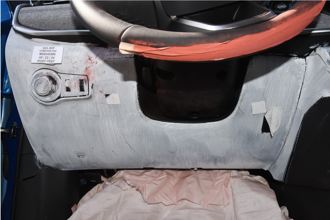
FIGURE 45. Post-Test Driver's Side Knee Bolster
