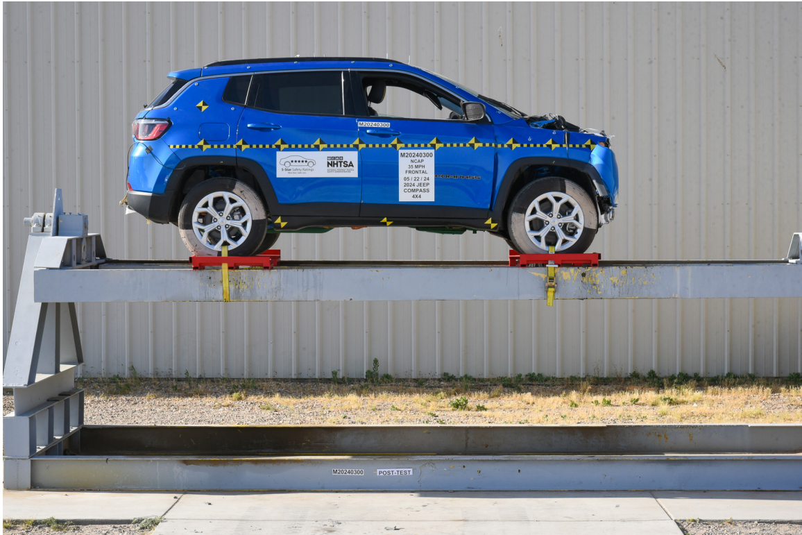
FIGURE 77. Vehicle at 0° on Static Rollover Device
