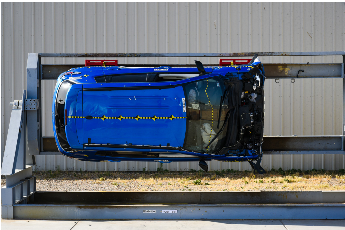
FIGURE 78. Vehicle at 90° on Static Rollover Device
