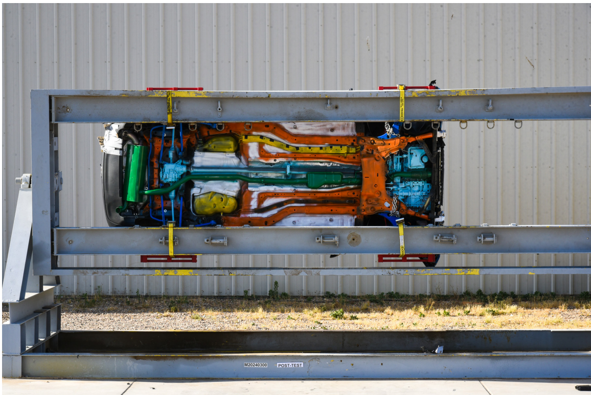
FIGURE 80. Vehicle at 270° on Static Rollover Device
