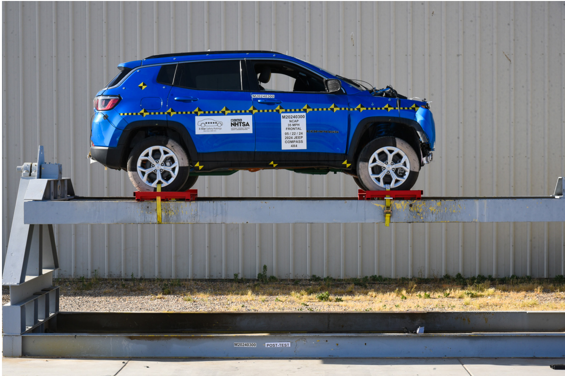
FIGURE 81. Vehicle at 360° on Static Rollover Device
