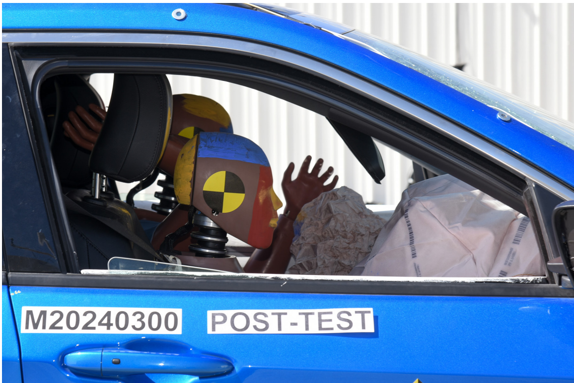
FIGURE 56. Post-Test Passenger Dummy Window View
