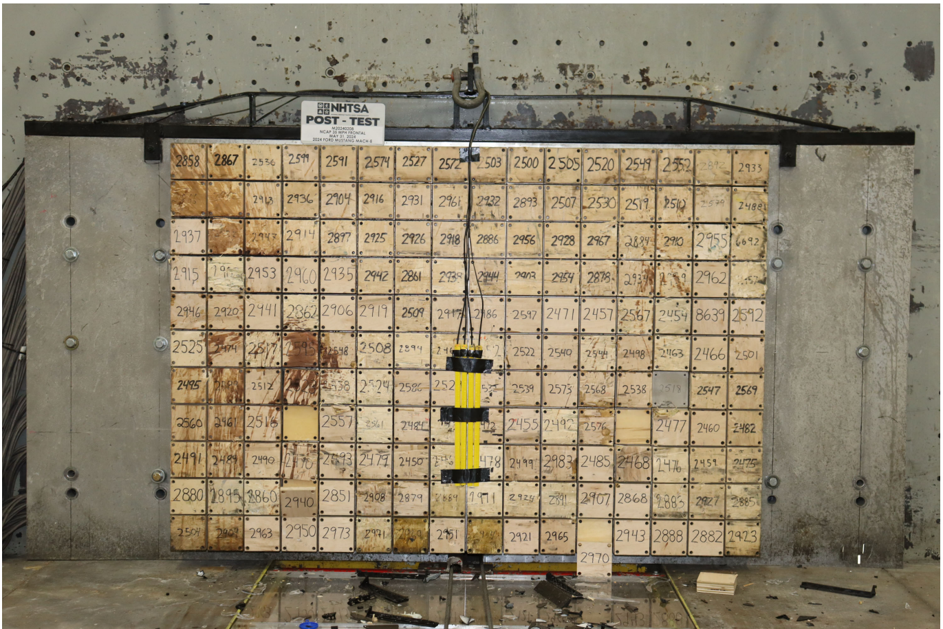
Photo No. 003 - Post-Test Load Cell Wall
