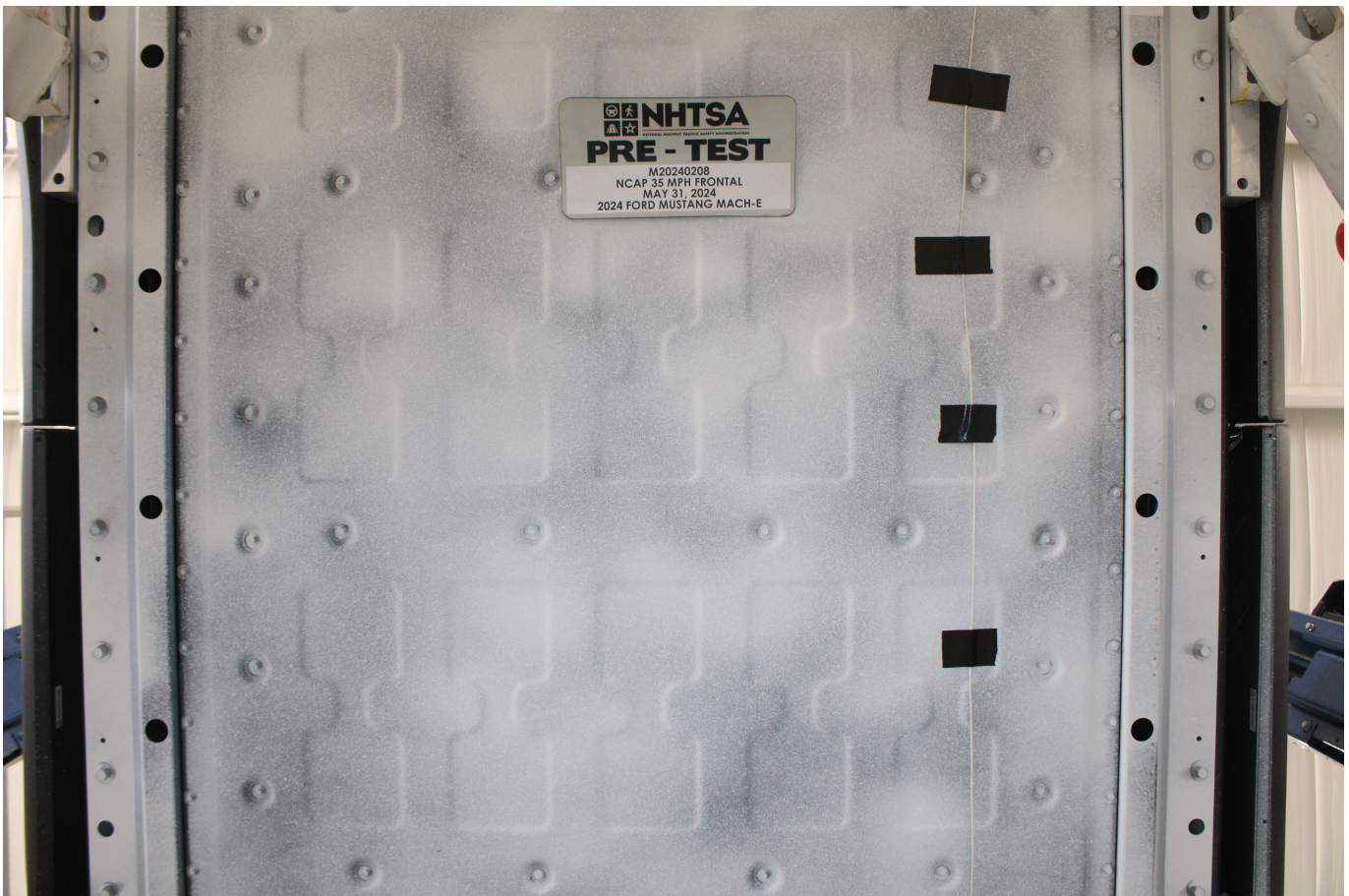
Photo No. 305-09 - Pre-Impact View of Propulsion Battery
