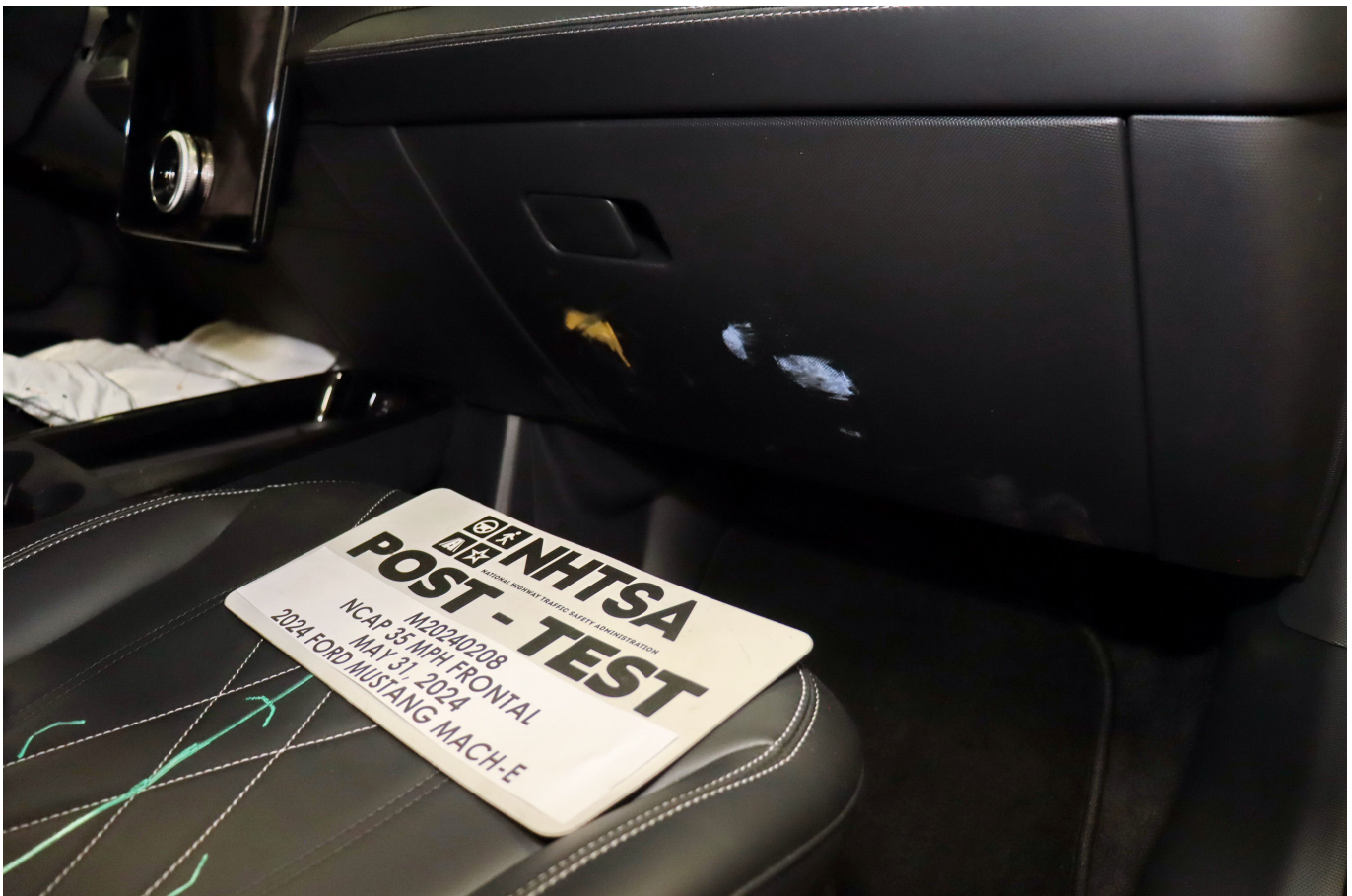
Photo No. 068 - Post-Test Passenger's Side Knee Bolster
