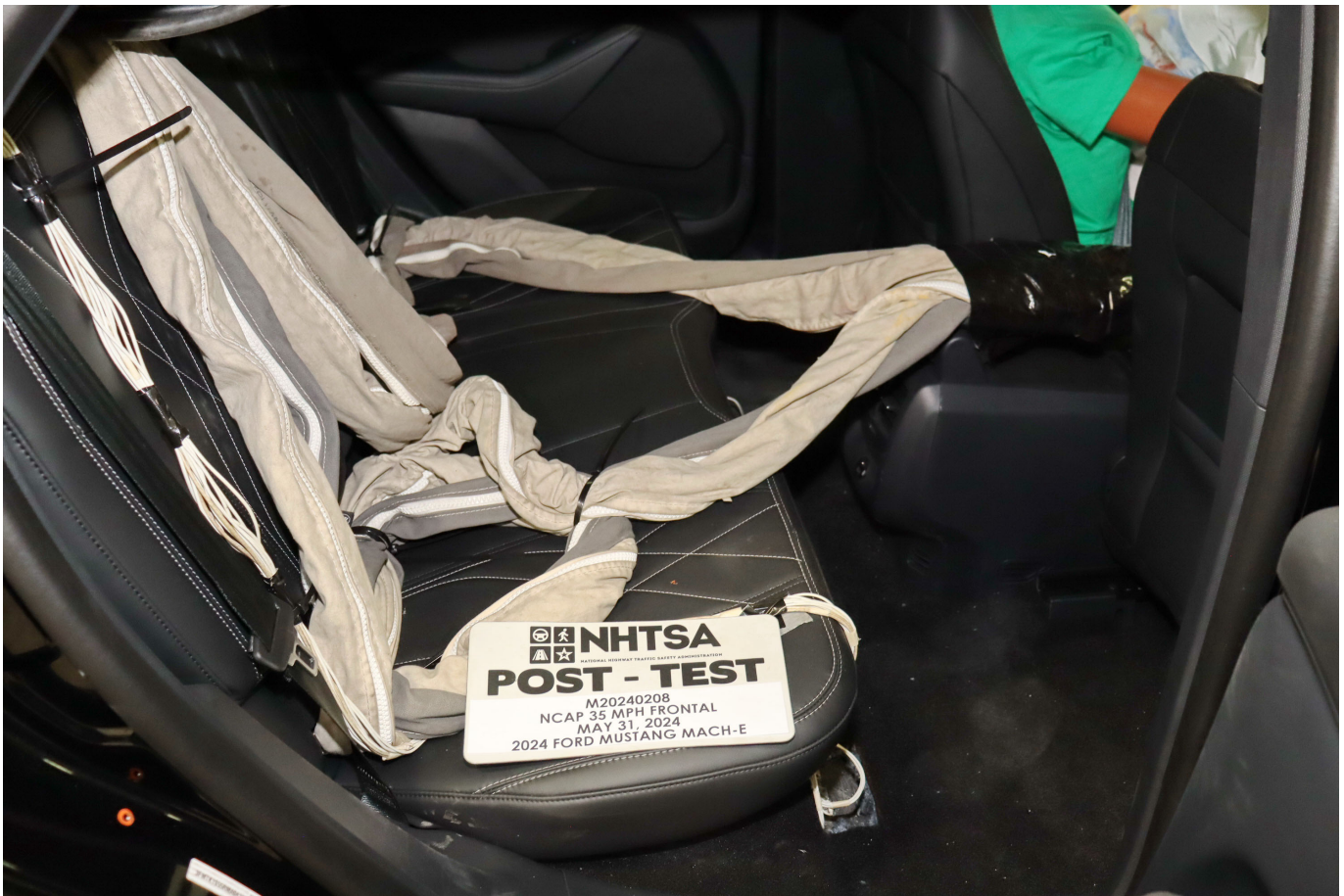
Photo No. 029 - Post-Test Dummy Cable Routing
