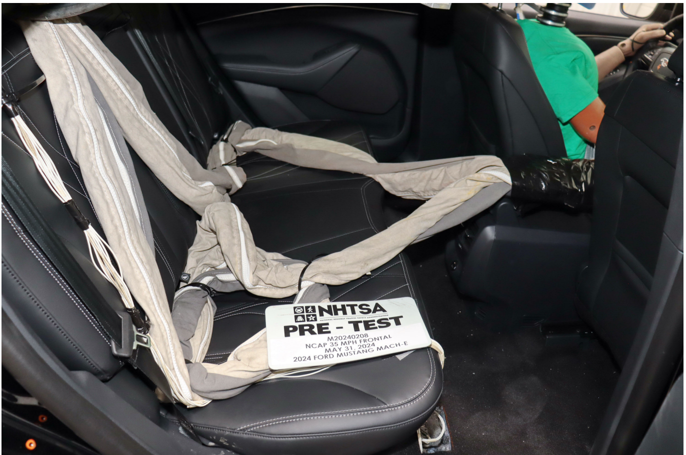
Photo No. 028 - Pre-Test Dummy Cable Routing
