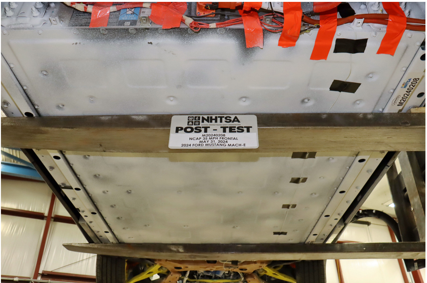
Photo No. 305-11 - Post-Impact Rear View of Propulsion Battery
