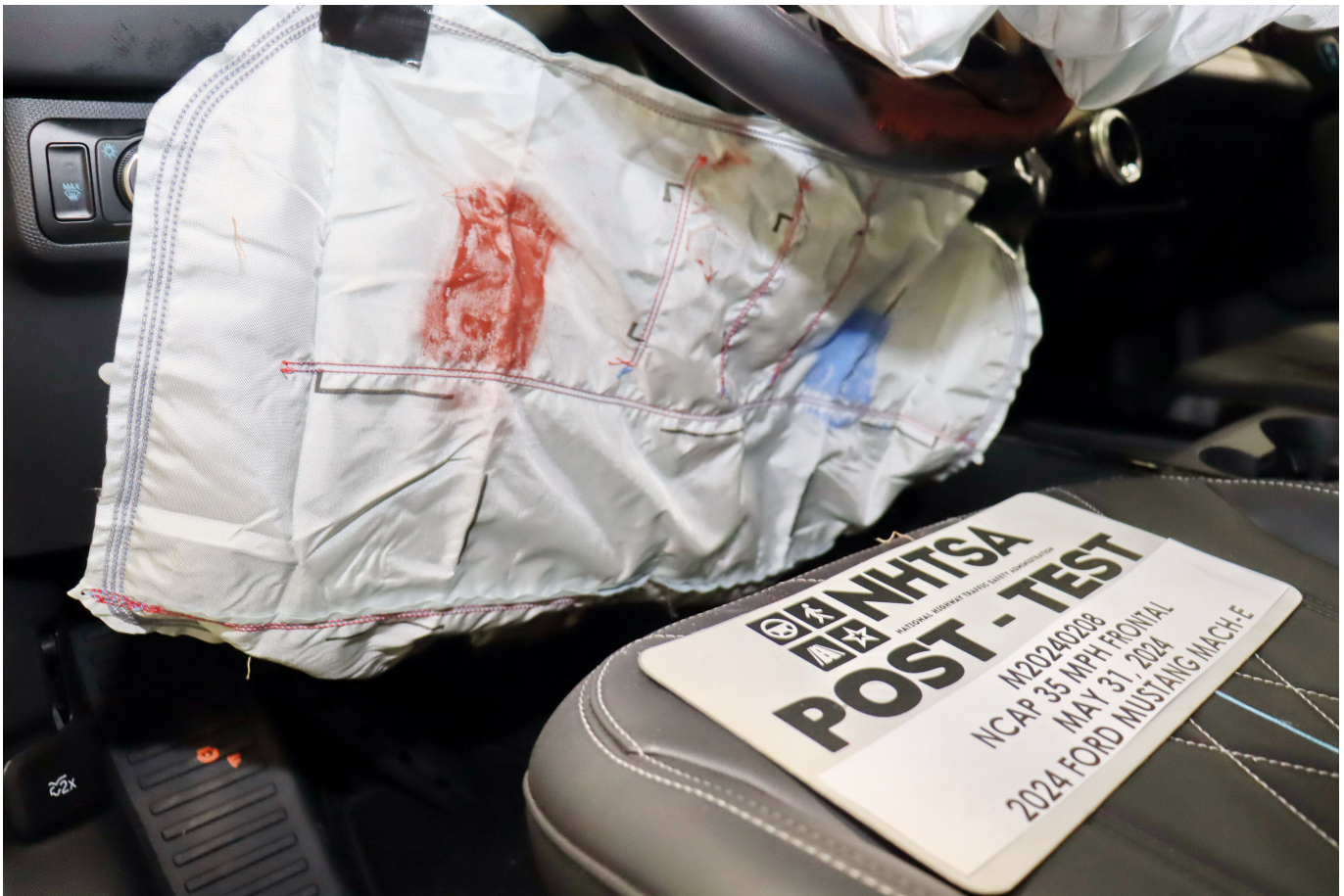
Photo No. 045 - Post-Test Driver's Side Knee Bolster
