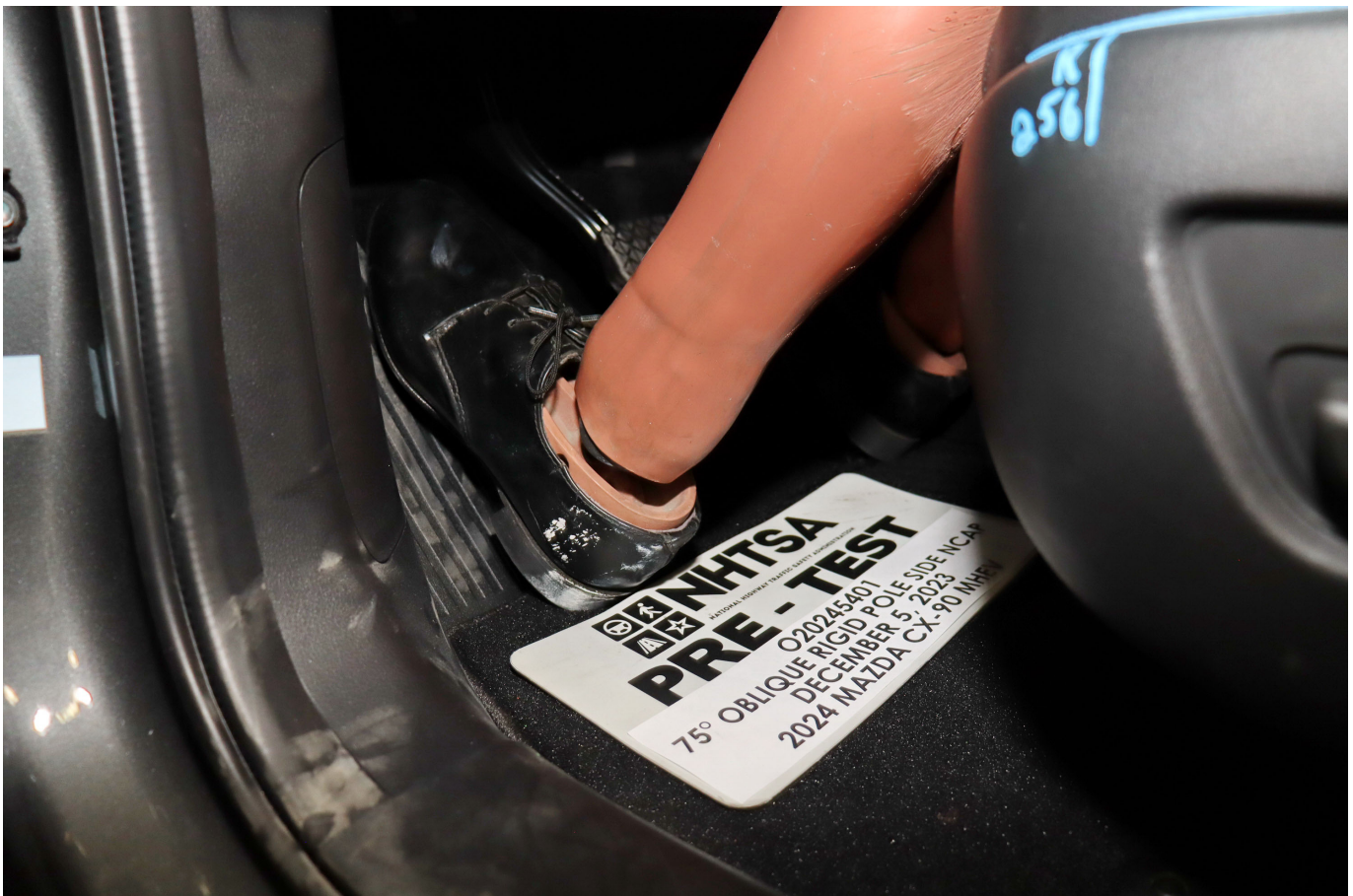
Photo No. 032 - Pre-Test Placement of Dummy's Feet
