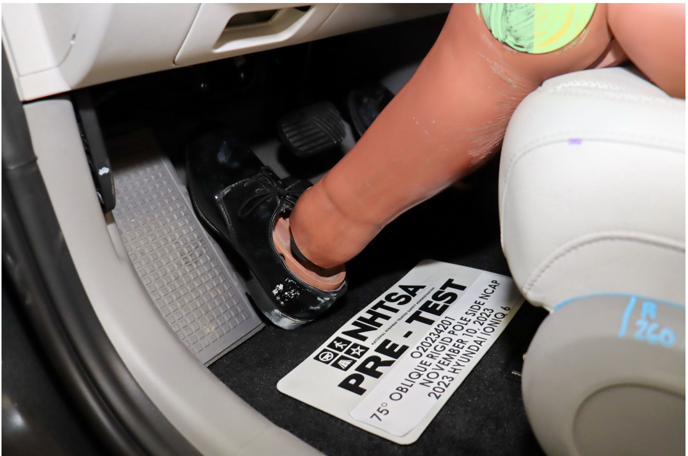
Photo No. 032 - Pre-Test Placement of Dummy's Feet
