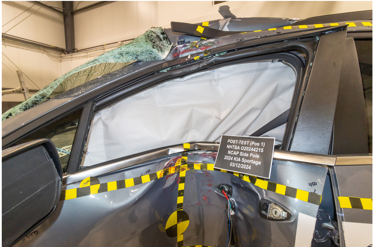
Figure A-25: Post-Test Left Side View of Dummy Shoulder and Door Top View
