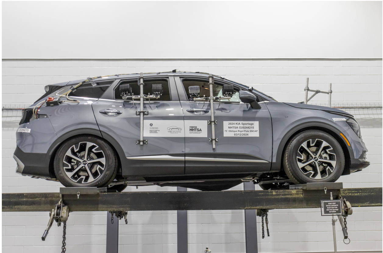
Figure A-65: FMVSS No. 301 Static Rollover 0 Degrees
