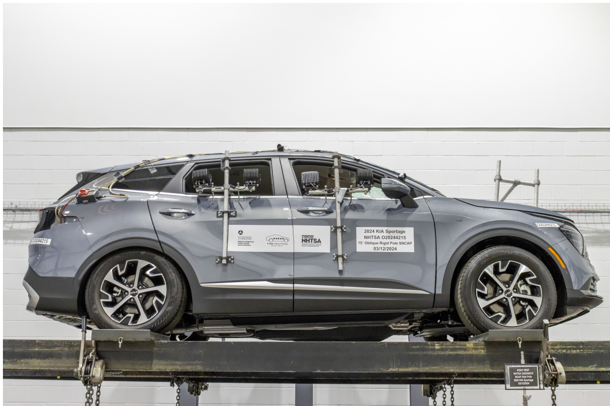
Figure A-69: FMVSS No. 301 Static Rollover 360 Degrees
