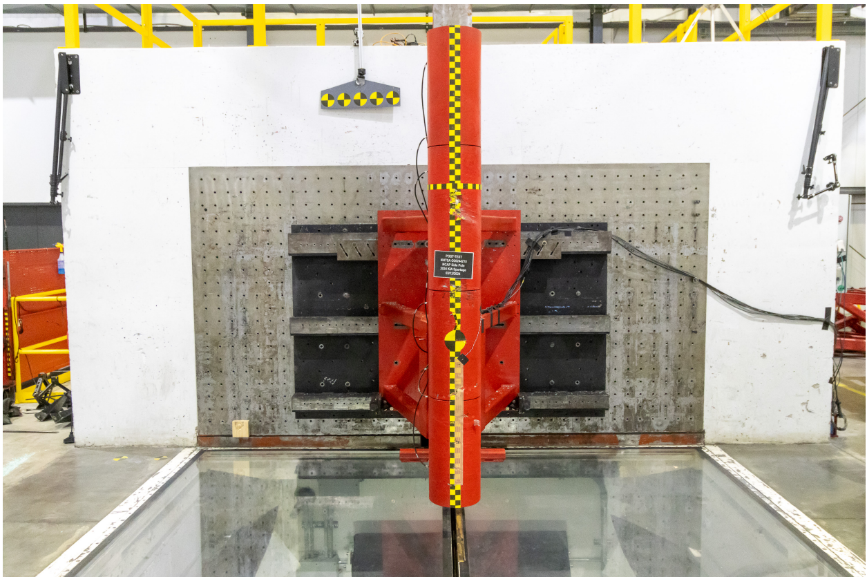
Figure A-60: Post-Test Pole Barrier Front View
