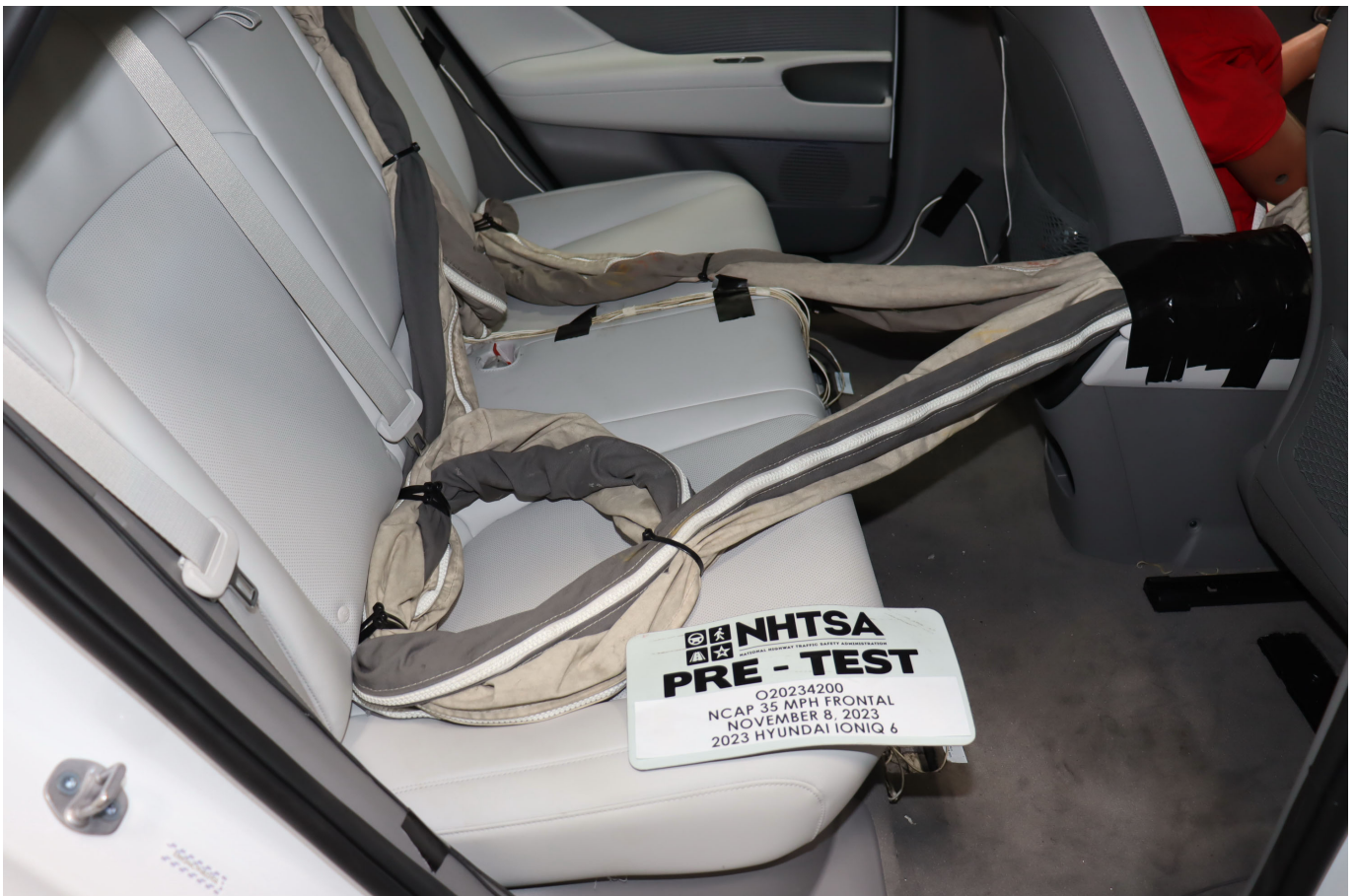
Photo No. 028 - Pre-Test Dummy Cable Routing
