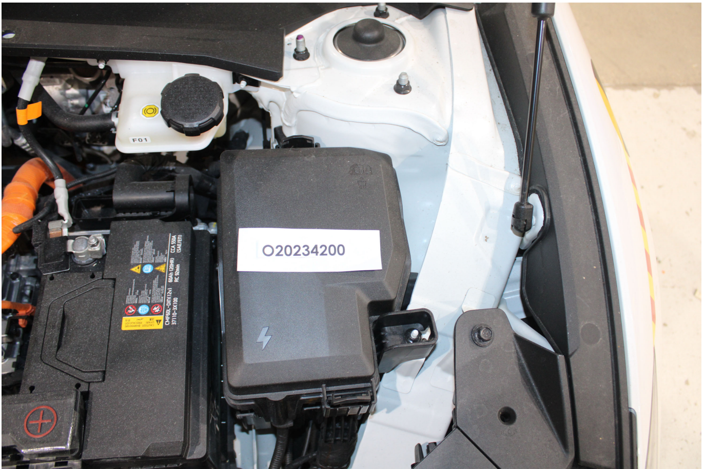
Photo No. 305-04 - First Responder Warning Location
