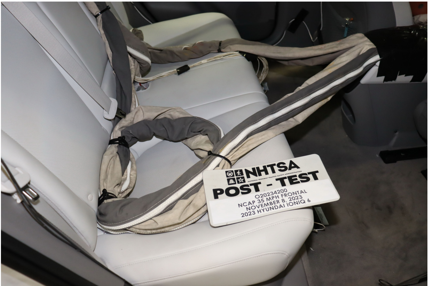
Photo No. 029 - Post-Test Dummy Cable Routing
