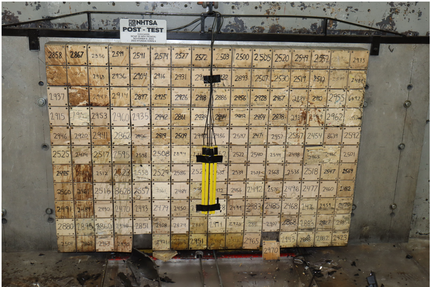
Photo No. 003 - Post-Test Load Cell Wall
