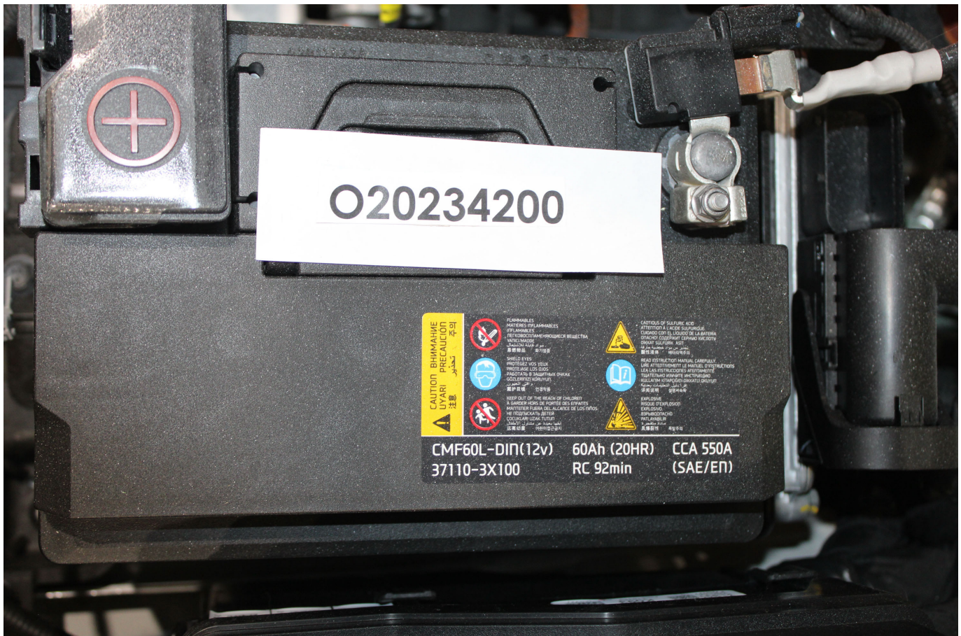
Photo No. 305-01 - Auxiliary Power Module Warning Label
