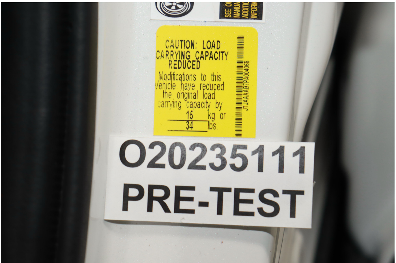
Photo No. 005a - Vehicle Load Carrying Capacity Reduction Label
