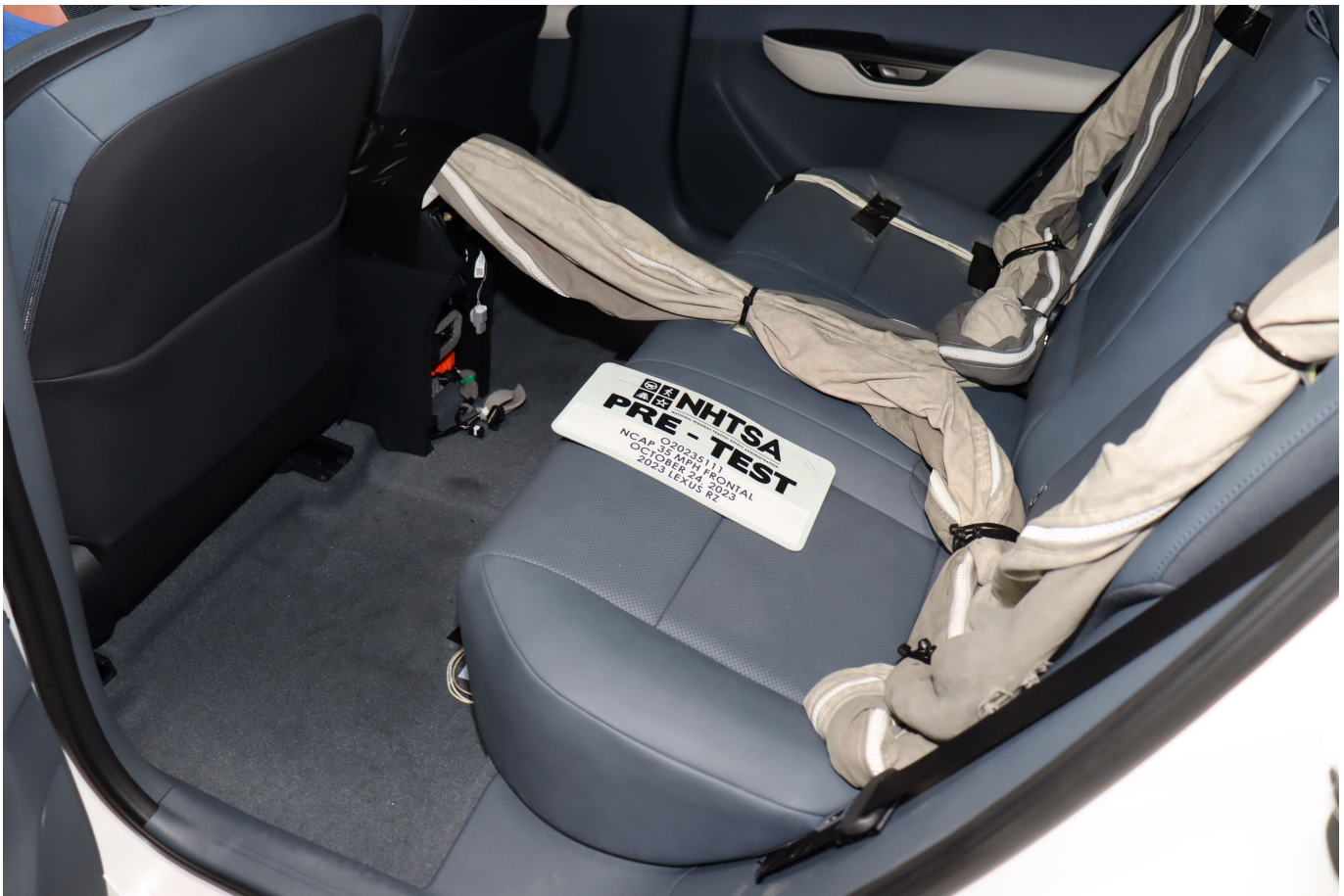
Photo No. 028 - Pre-Test Dummy Cable Routing
