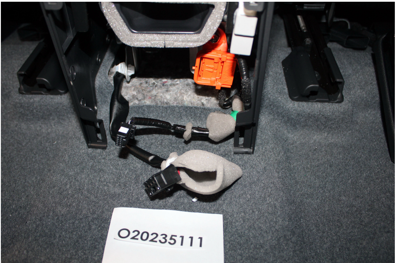
Photo No. 305-06 - Manual High Voltage Service Disconnect in Place
