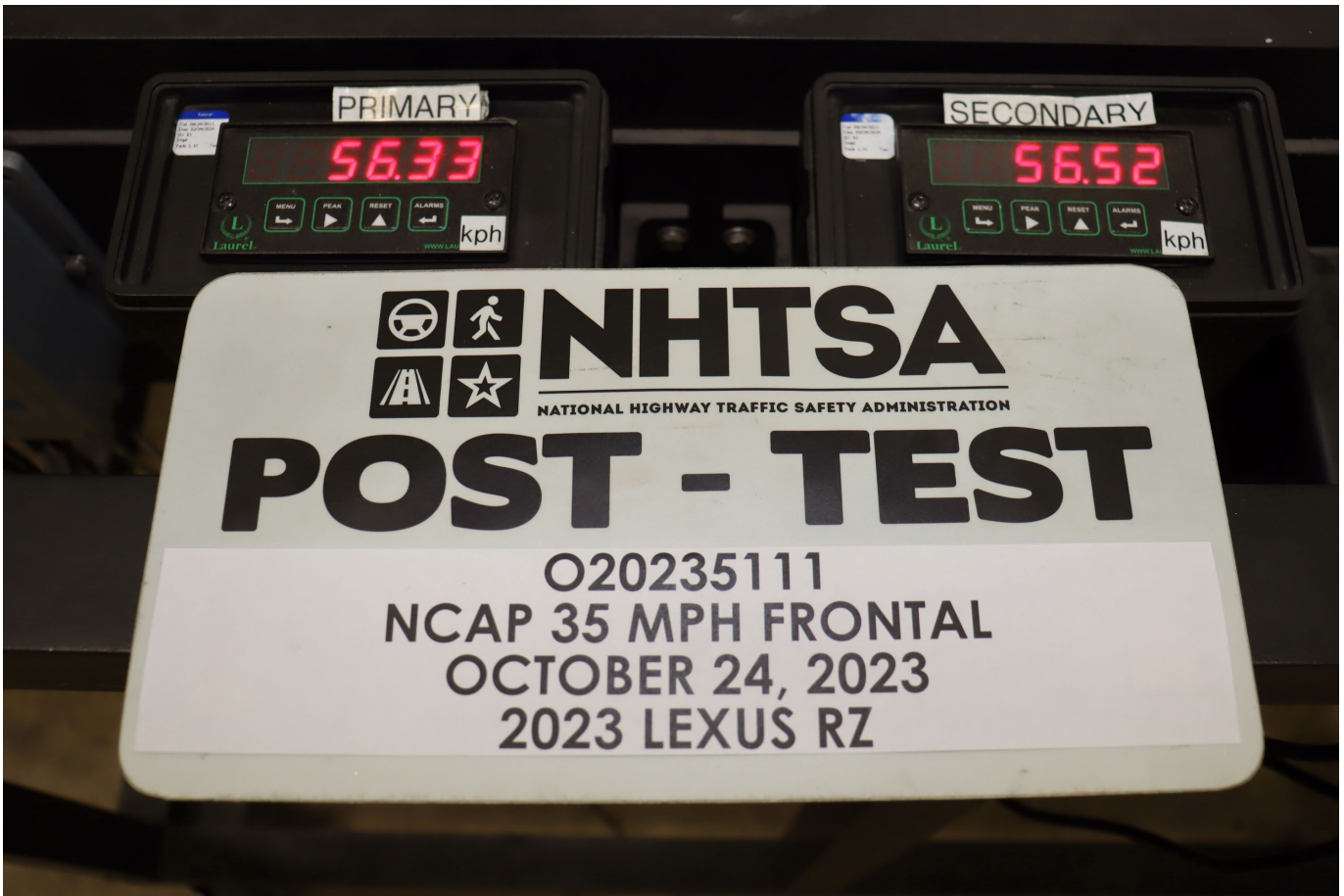
Photo No. 076 - Post-Test Speed Trap Read-Out
