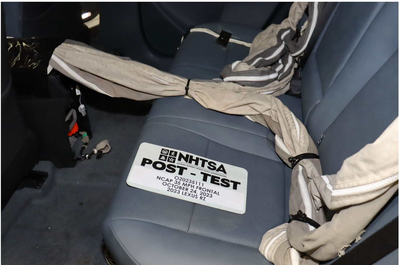
Photo No. 029 - Post-Test Dummy Cable Routing
