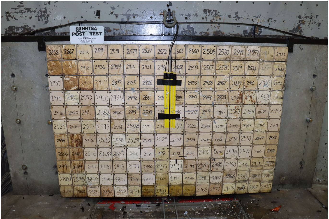
Photo No. 003 - Post-Test Load Cell Wall
