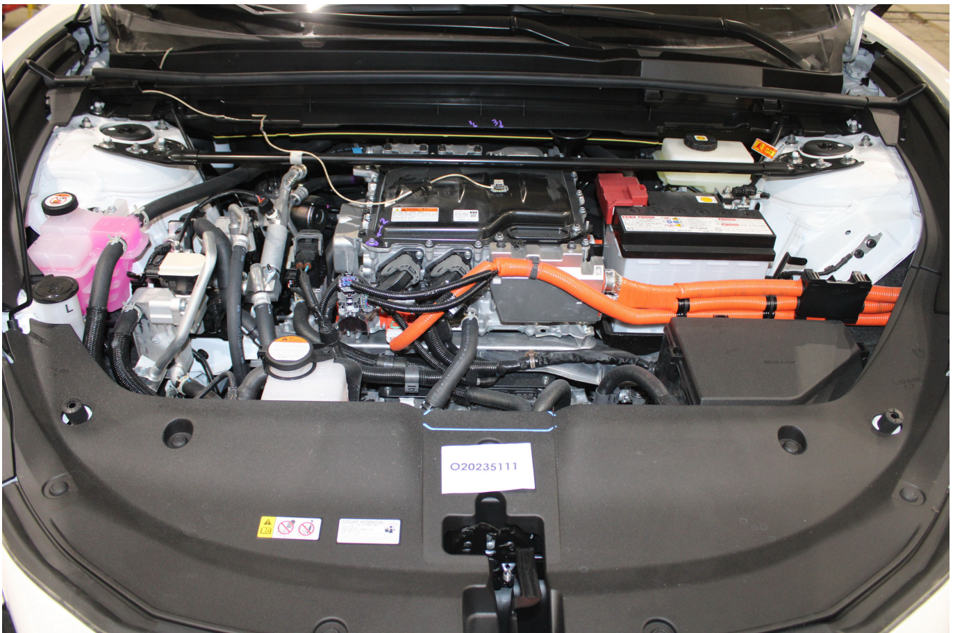
Photo No. 305-16 - Pre-Impact View of Electric Propulsion Drive
