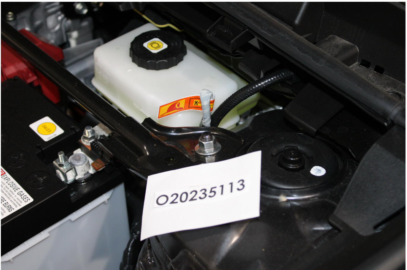
Photo No. 305-03 - First Responder Warning Label
