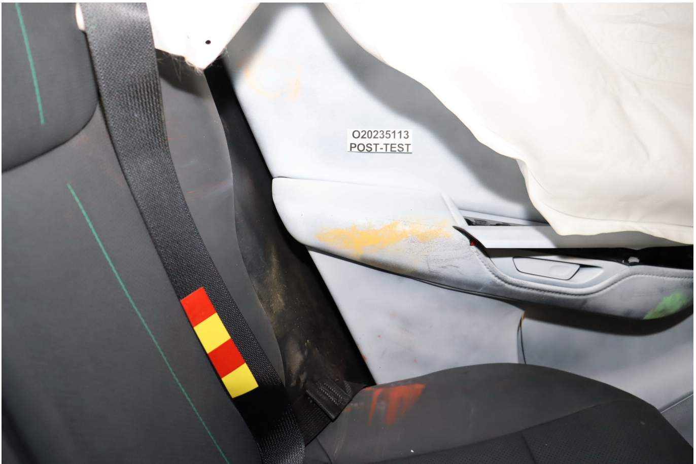
Photo No. 077 - Post-Test Rear Passenger Dummy Close-Up Torso Contact with Vehicle Interior View
