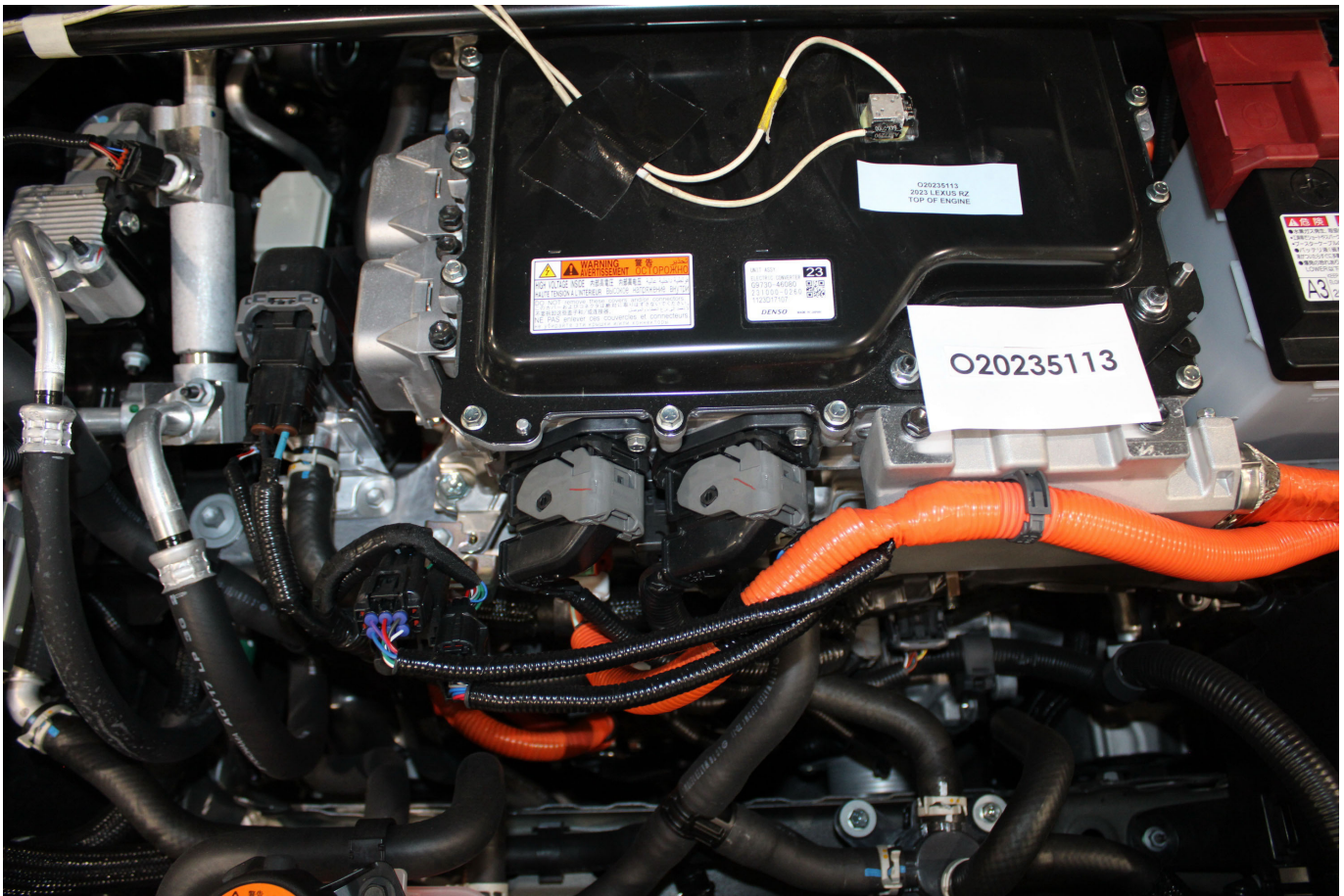
Photo No. 305-02 - Power Inverter Warning Label
