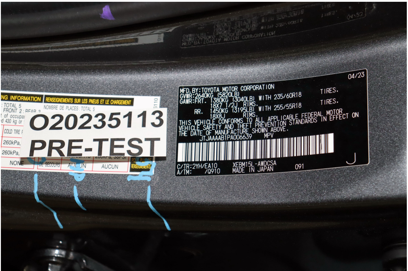
Photo No. 092 - Close-Up View of Vehicle's Certification Label
