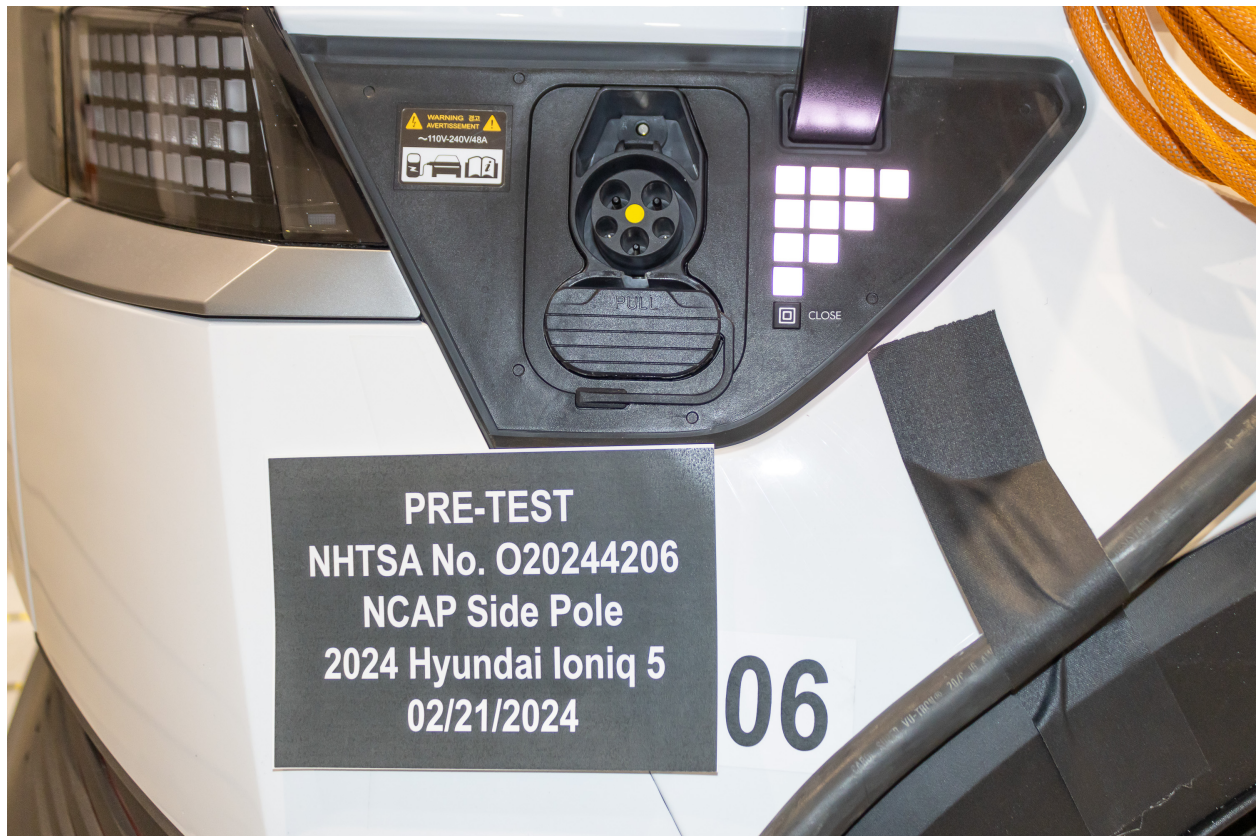
Figure A-55: Pre-Test Charging Port
