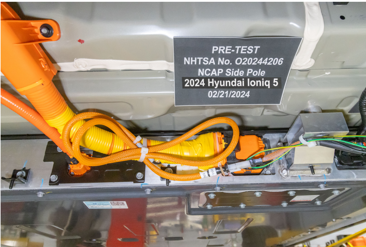
Figure 305-22: Pre-Impact View of High Voltage Leads Attached
