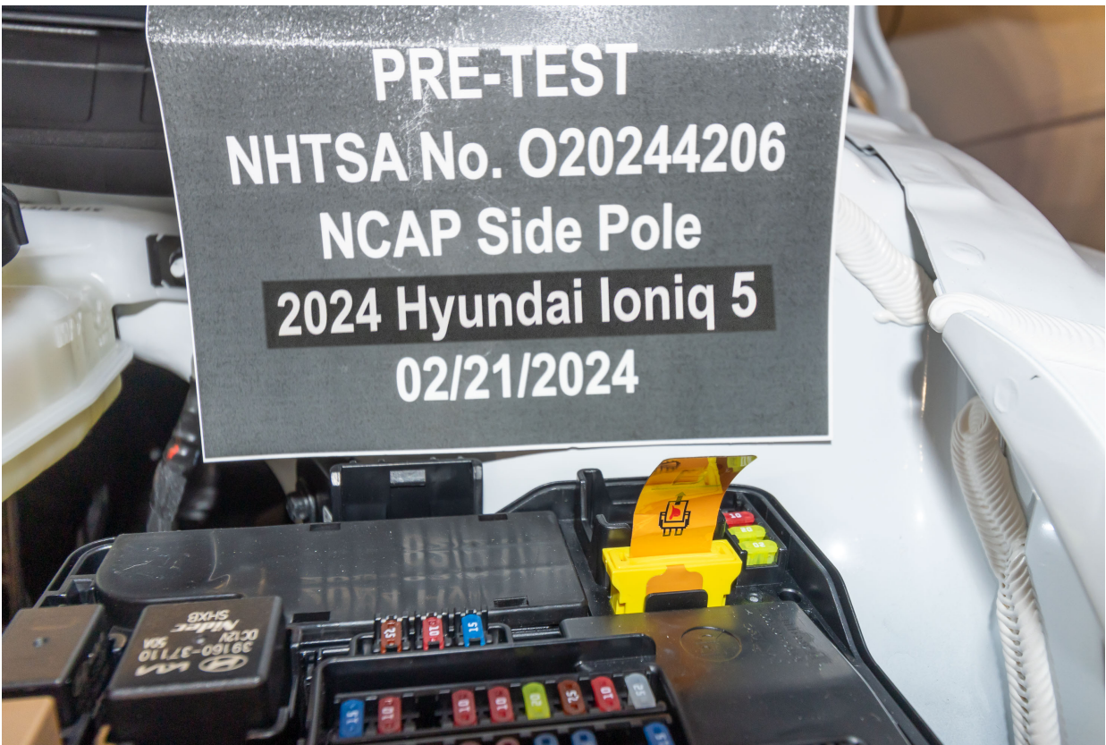
Figure 305-6: Manual High Voltage Service Disconnect in Place
