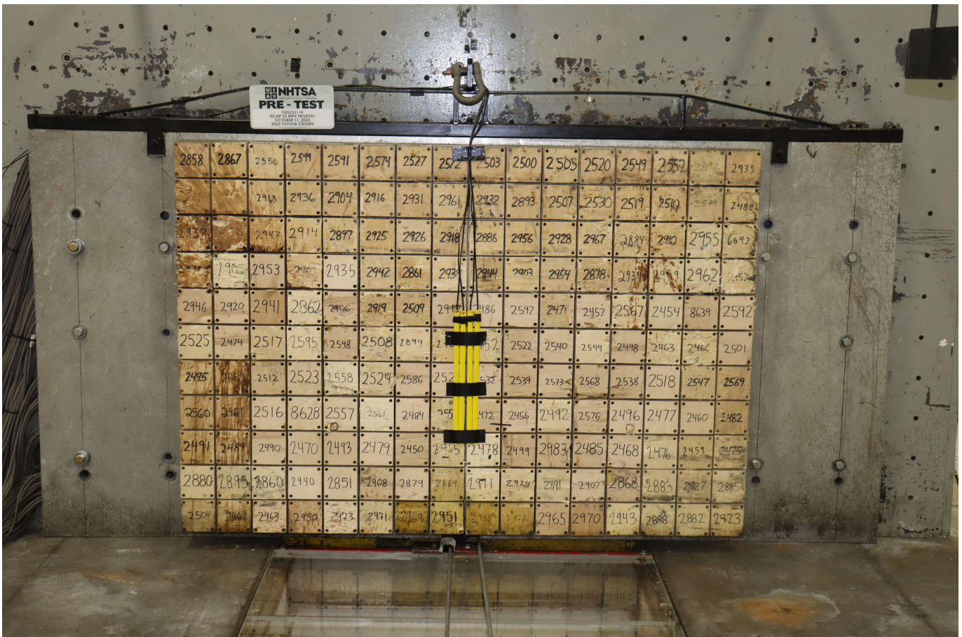
Photo No. 002 - Pre-Test Load Cell Wall
