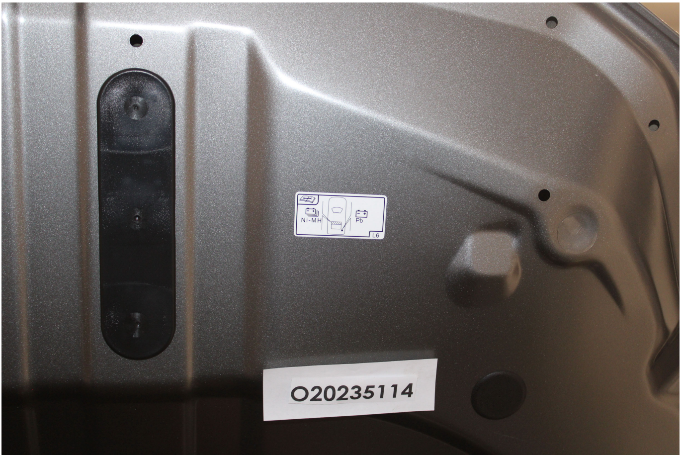
Photo No. 305-03 - First Responder Warning Label
