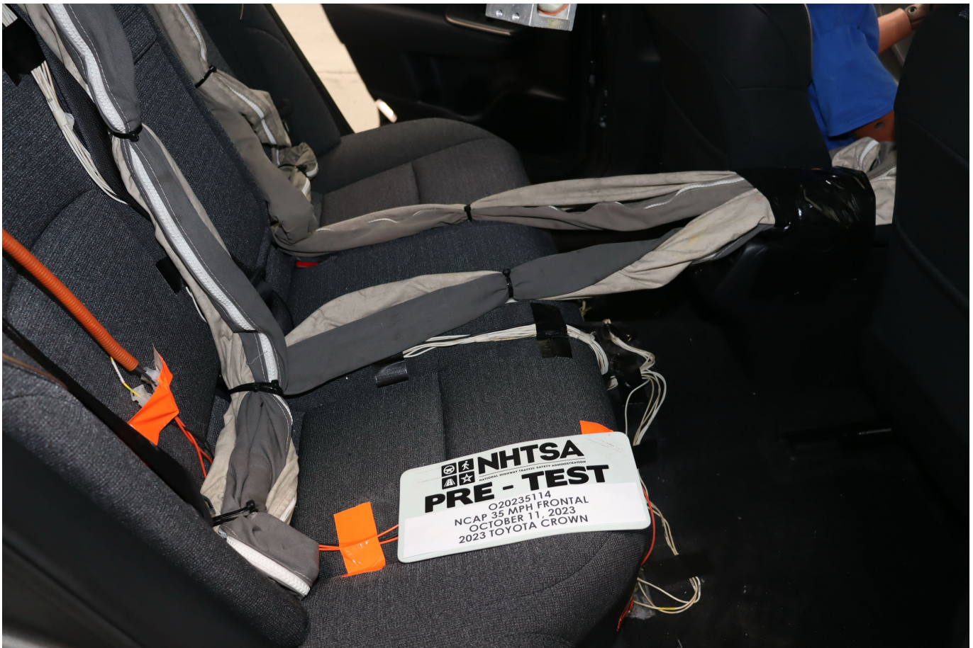
Photo No. 028 - Pre-Test Dummy Cable Routing
