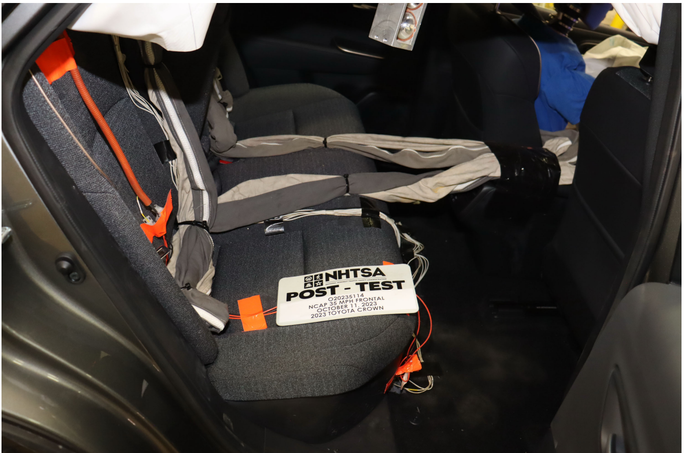
Photo No. 029 - Post-Test Dummy Cable Routing
