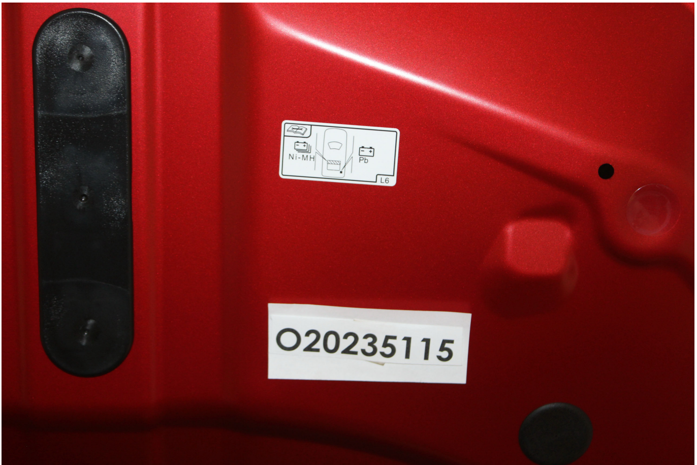
Photo No. 305-03 - First Responder Warning Label
