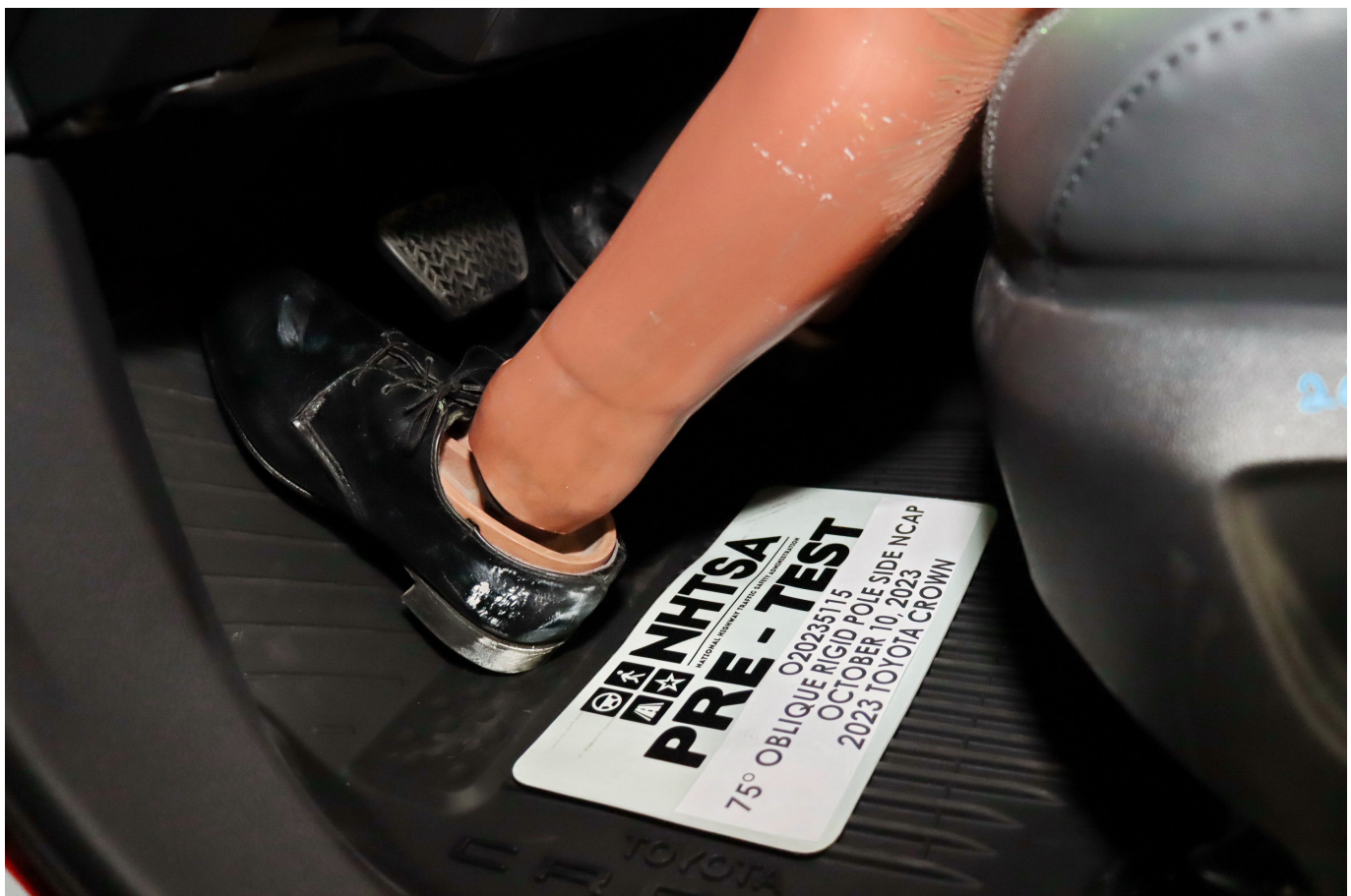
Photo No. 032 - Pre-Test Placement of Dummy's Feet
