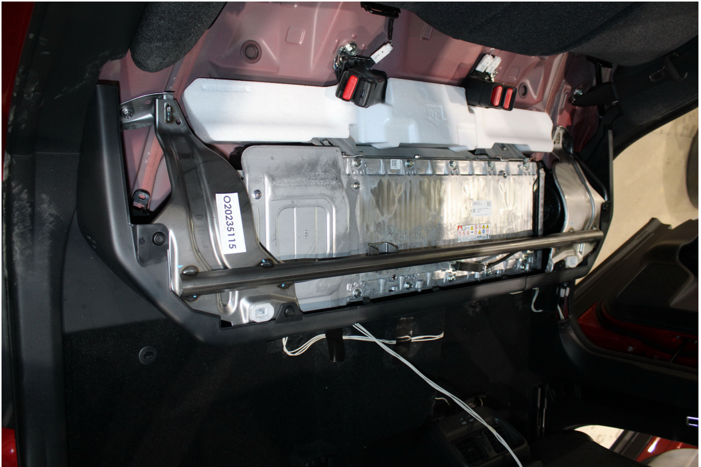
Photo No. 305-09 - Pre-Impact View of Propulsion Battery
