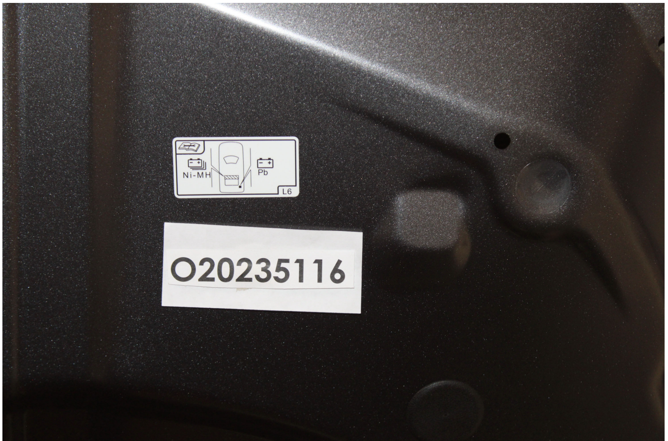
Photo No. 305-03 - First Responder Warning Label
