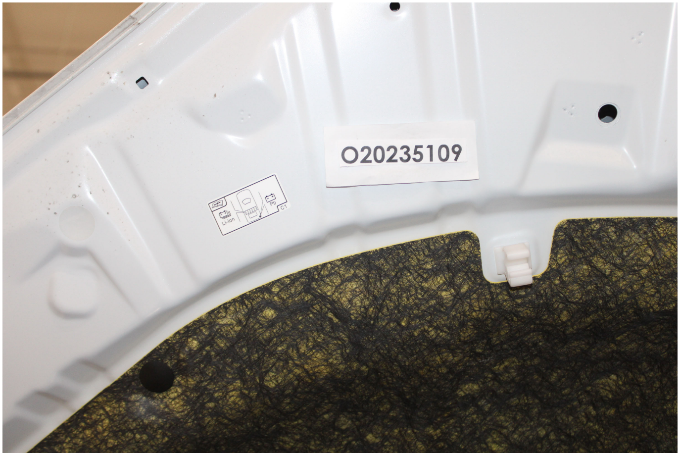
Photo No. 305-03 - First Responder Warning Label
