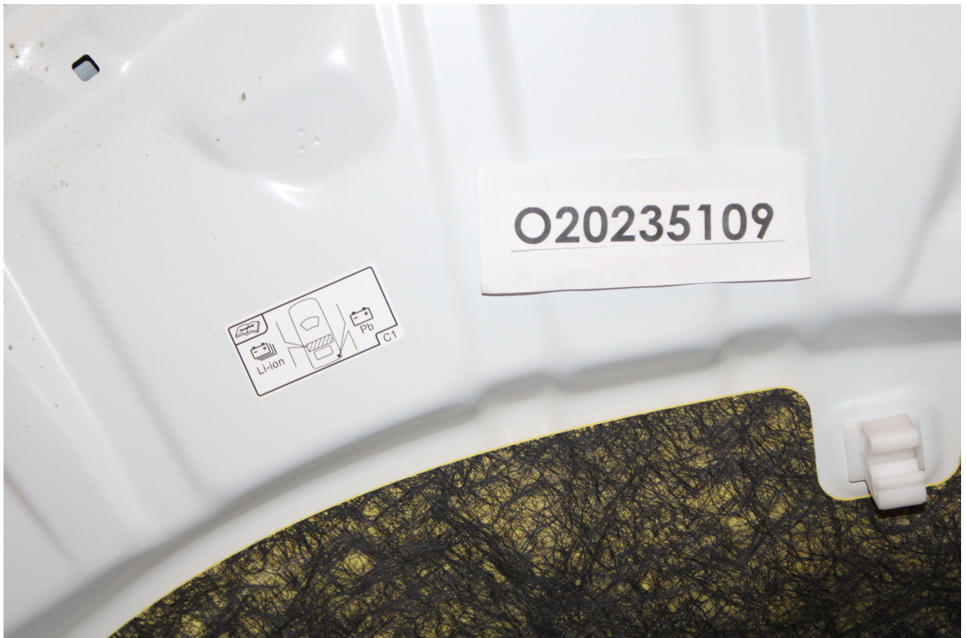
Photo No. 305-04 - First Responder Warning Location
