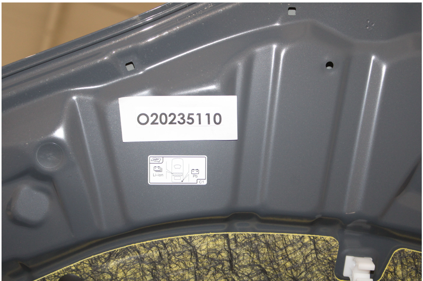
Photo No. 305-03 - First Responder Warning Label
