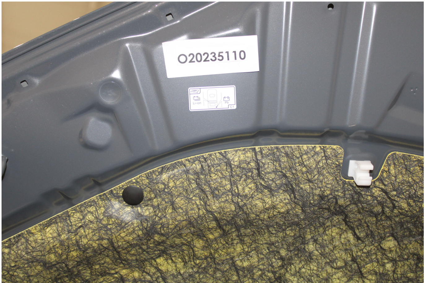
Photo No. 305-04 - First Responder Warning Location
