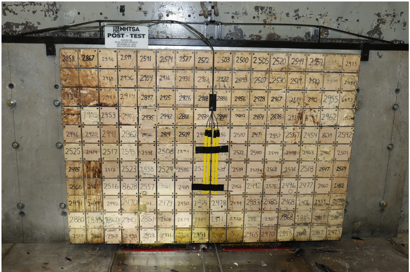
Photo No. 003 - Post-Test Load Cell Wall
