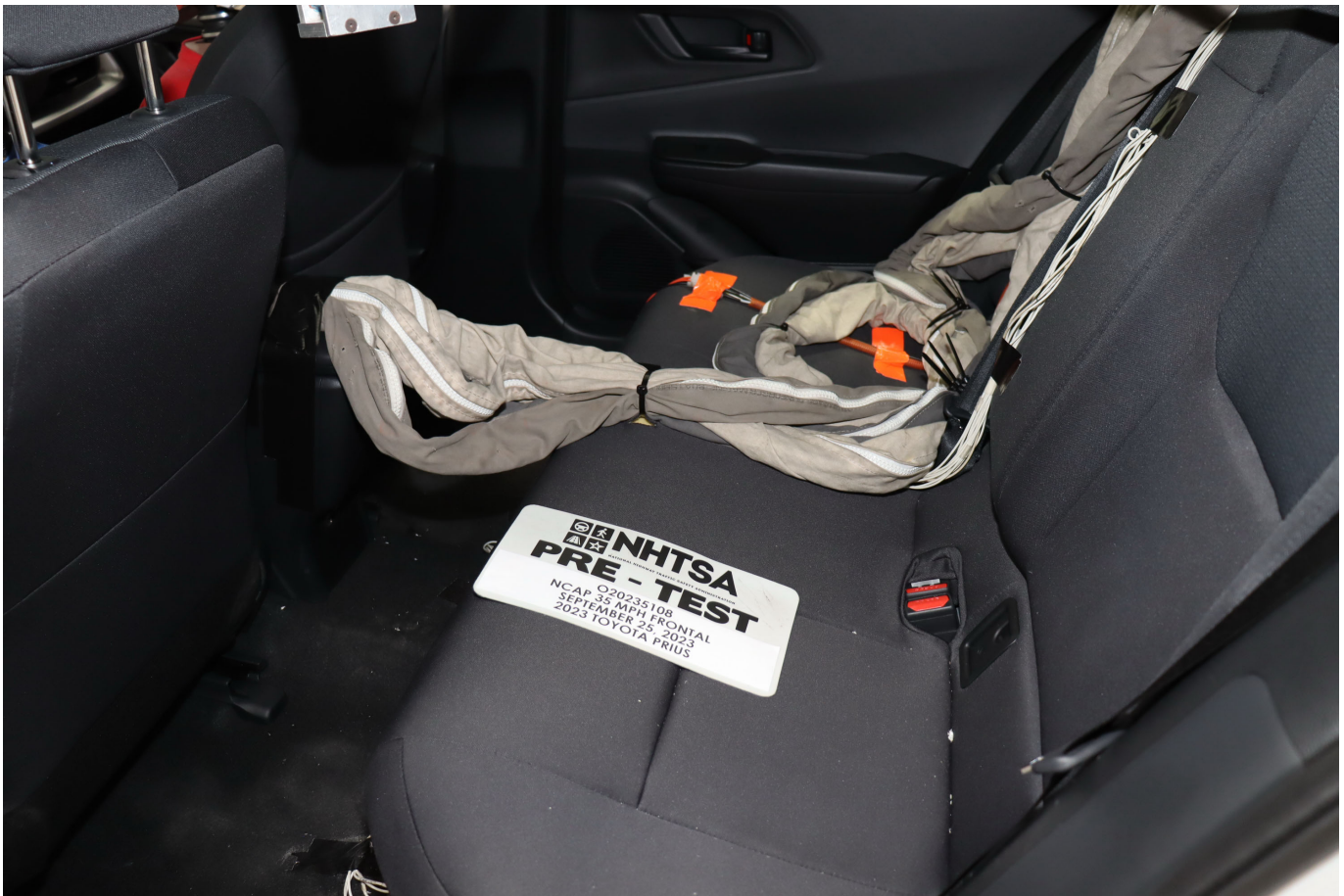
Photo No. 028 - Pre-Test Dummy Cable Routing
