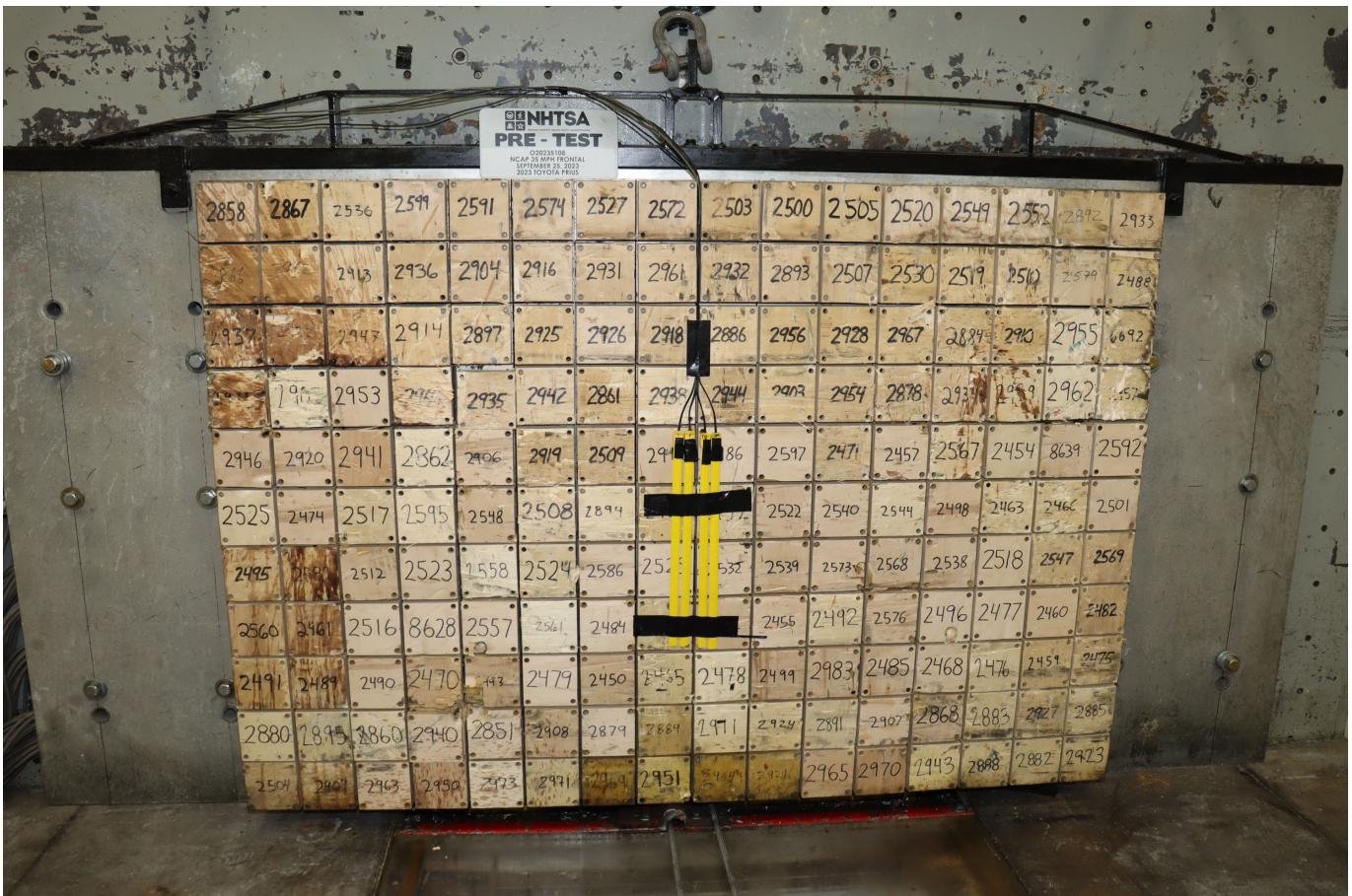
Photo No. 002 - Pre-Test Load Cell Wall
