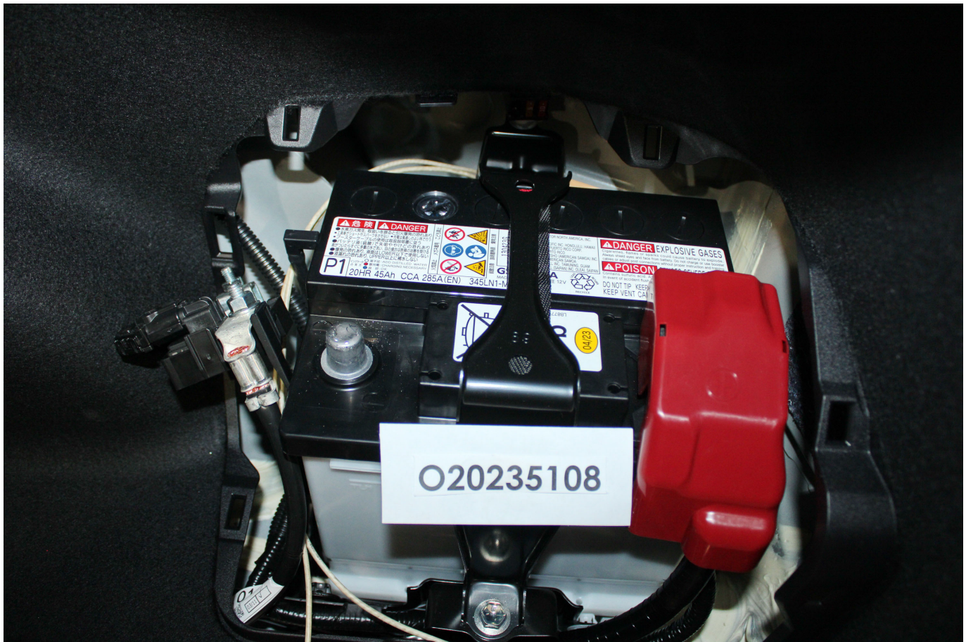
Photo No. 305-01 - Auxiliary Power Module Warning Label
