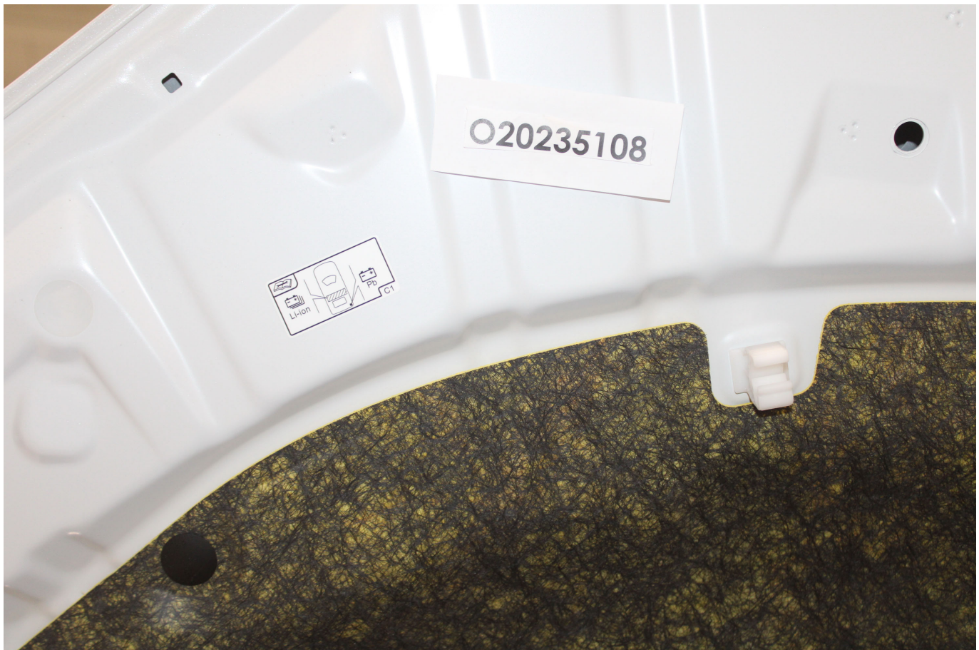
Photo No. 305-04 - First Responder Warning Location
