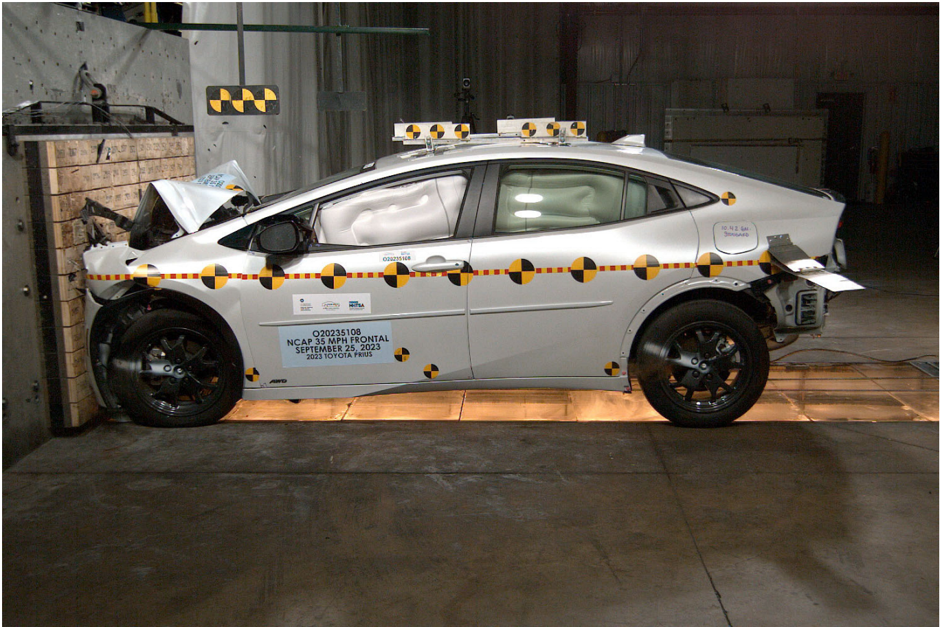
Photo No. 082 - 2023 Toyota Prius LE AWD 5-Door Hatchback Frontal Impact Event
