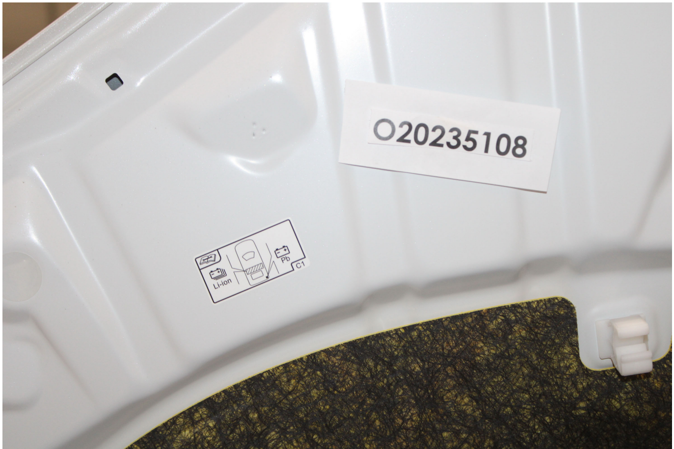
Photo No. 305-03 - First Responder Warning Label
