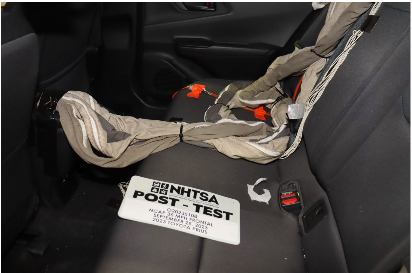
Photo No. 029 - Post-Test Dummy Cable Routing
