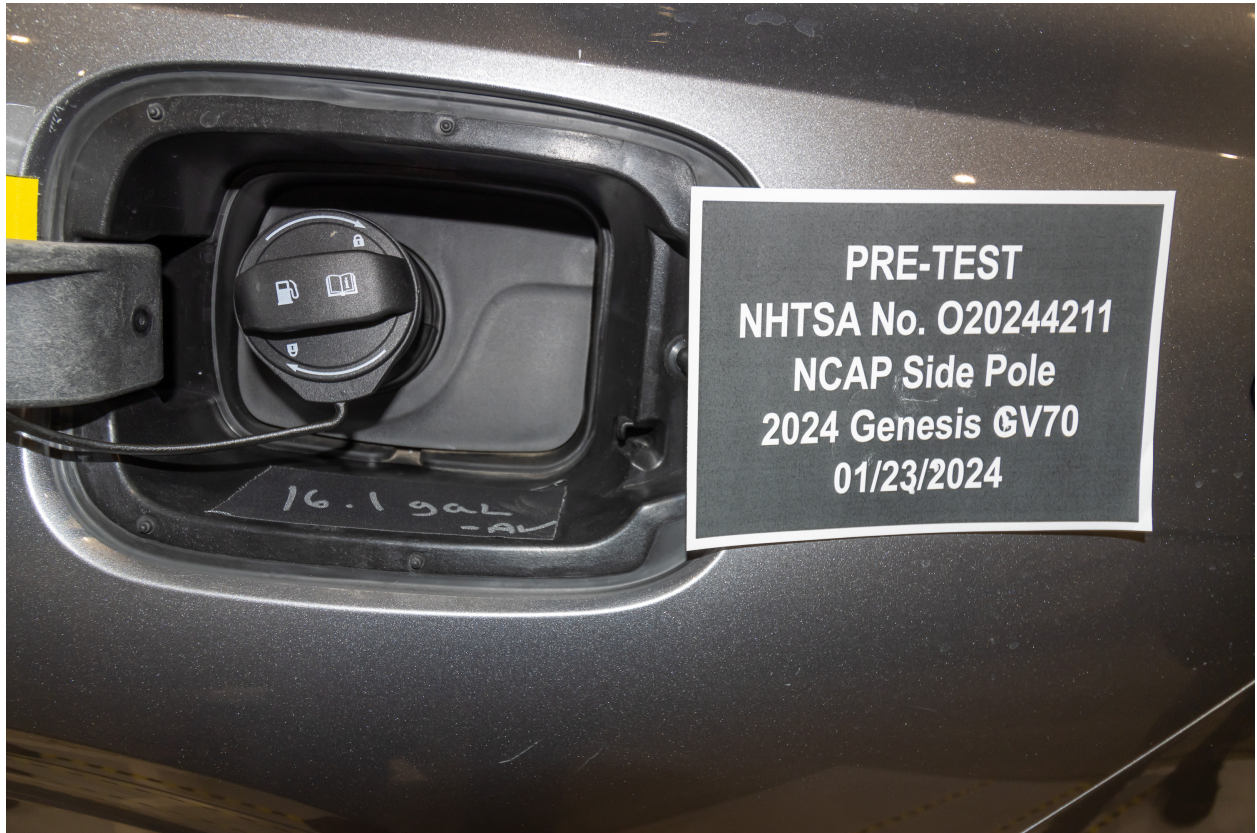
Figure A-55: Pre-Test View of Fuel Filler Cap or Fuel Filler Neck
