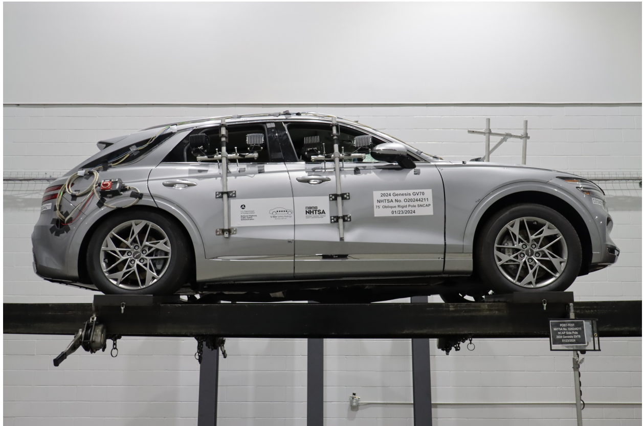
Figure A-65: FMVSS No. 301 Static Rollover 0 Degrees
