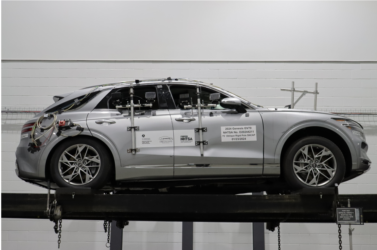
Figure A-69: FMVSS No. 301 Static Rollover 360 Degrees
