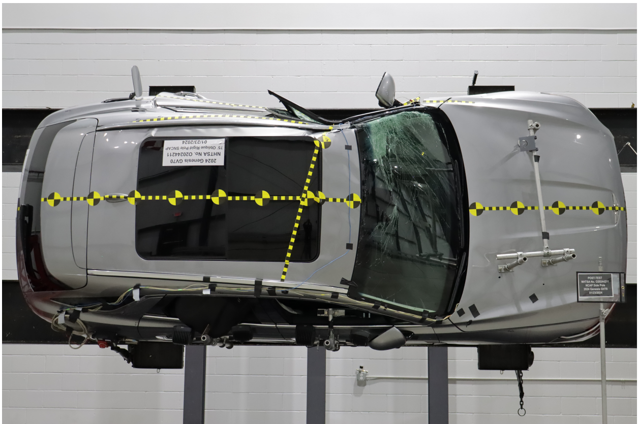
Figure A-68: FMVSS No. 301 Static Rollover 270 Degrees
