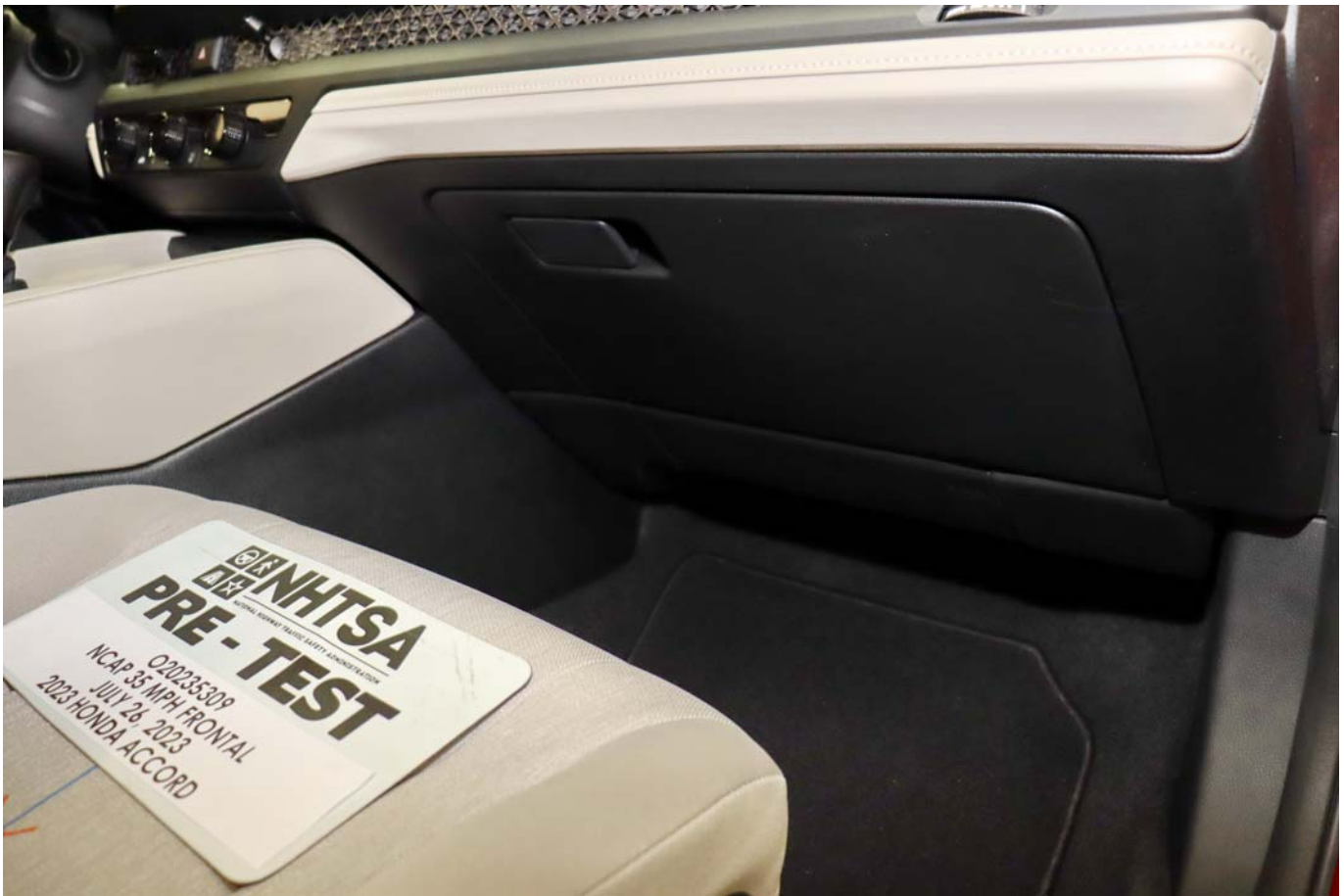
Photo No. 067 - Pre-Test Passenger's Side Knee Bolster
