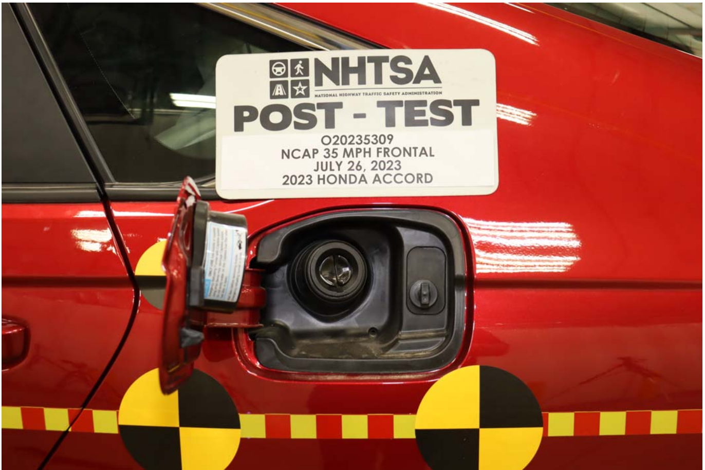
Photo No. 023 - Post-Test Fuel Filler Cap View
