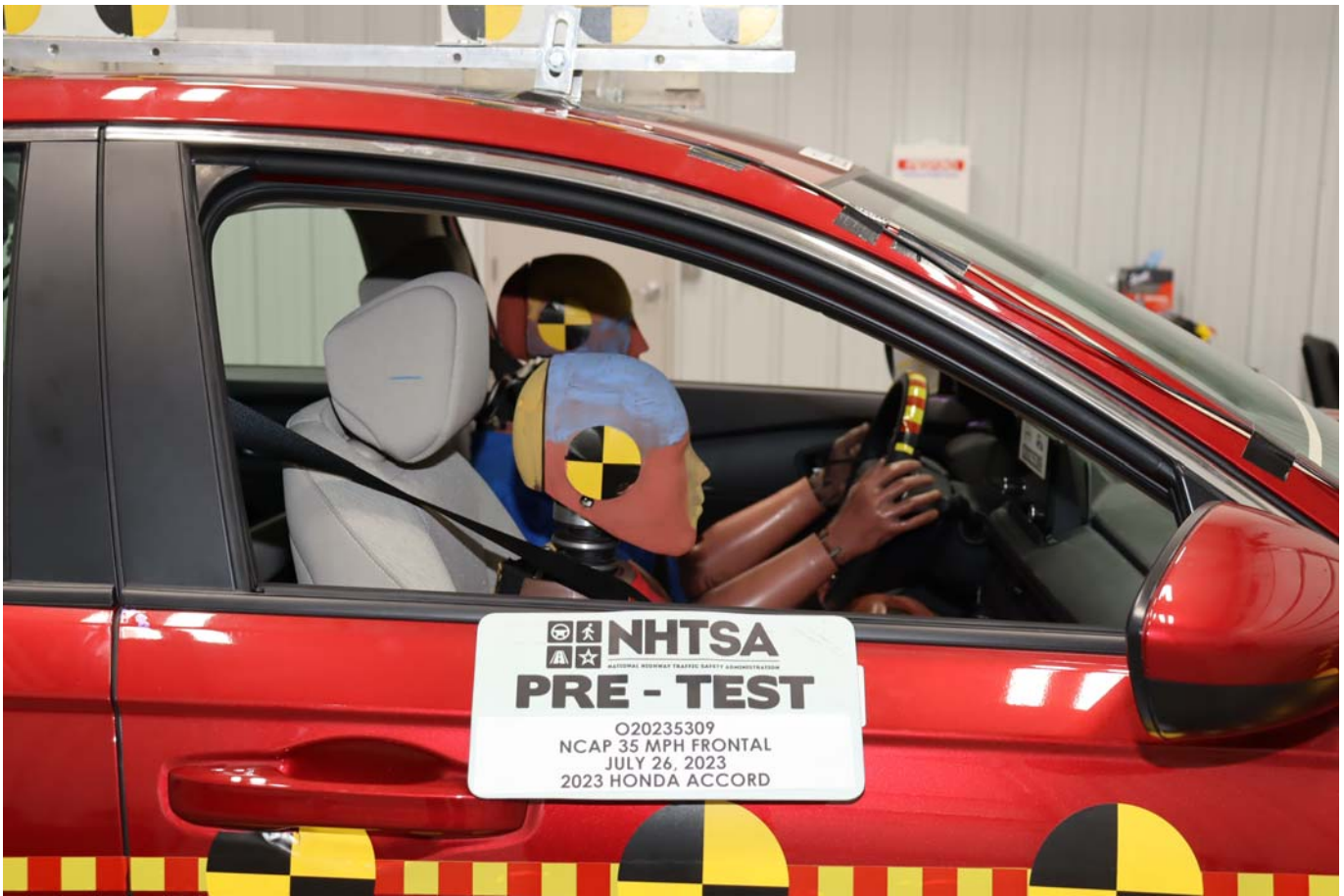
Photo No. 055 - Pre-Test Passenger Dummy Window View
