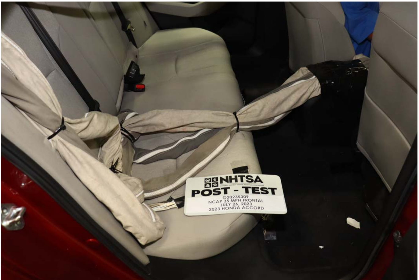
Photo No. 029 - Post-Test Dummy Cable Routing
