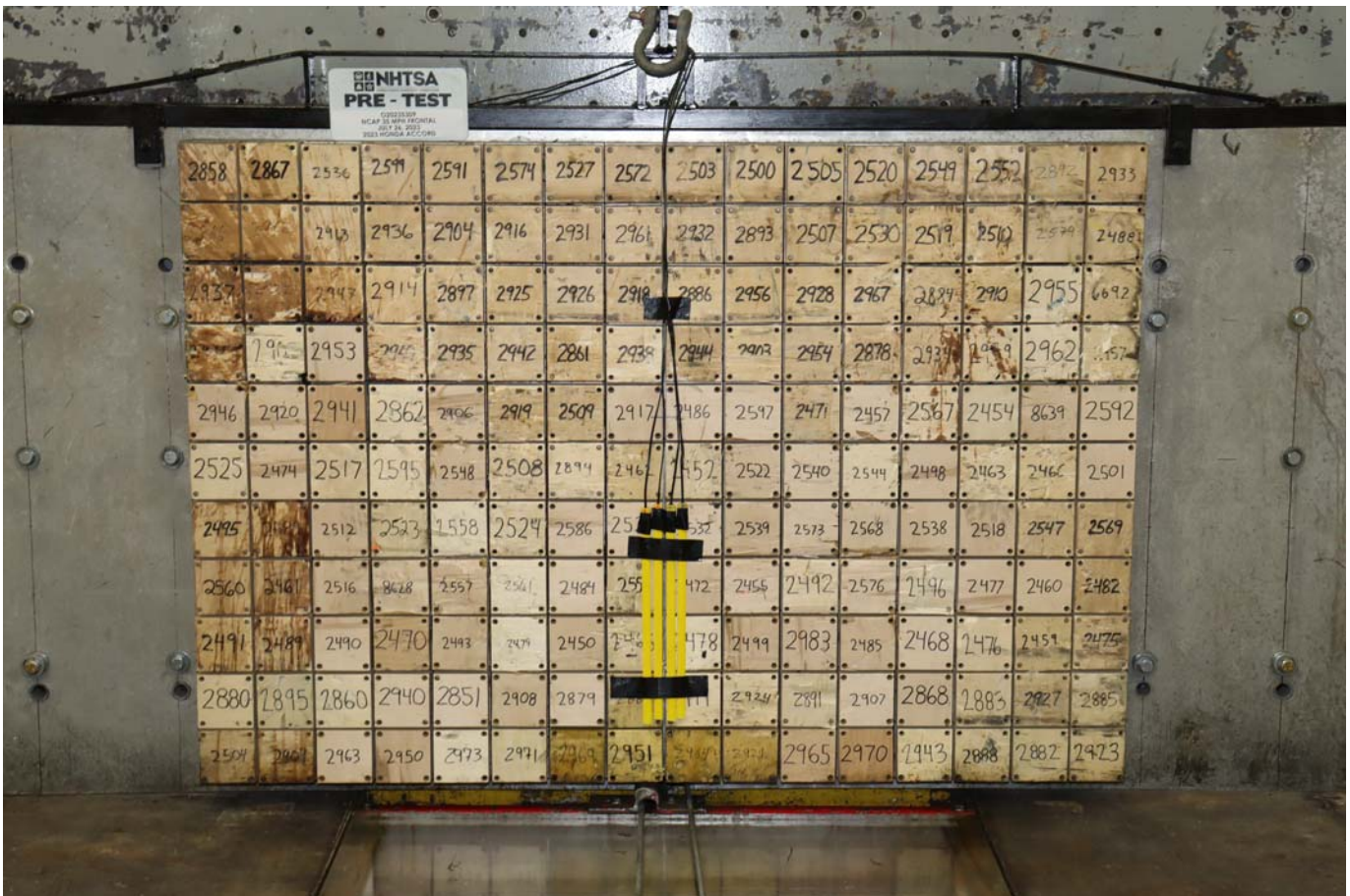
Photo No. 002 - Pre-Test Load Cell Wall
