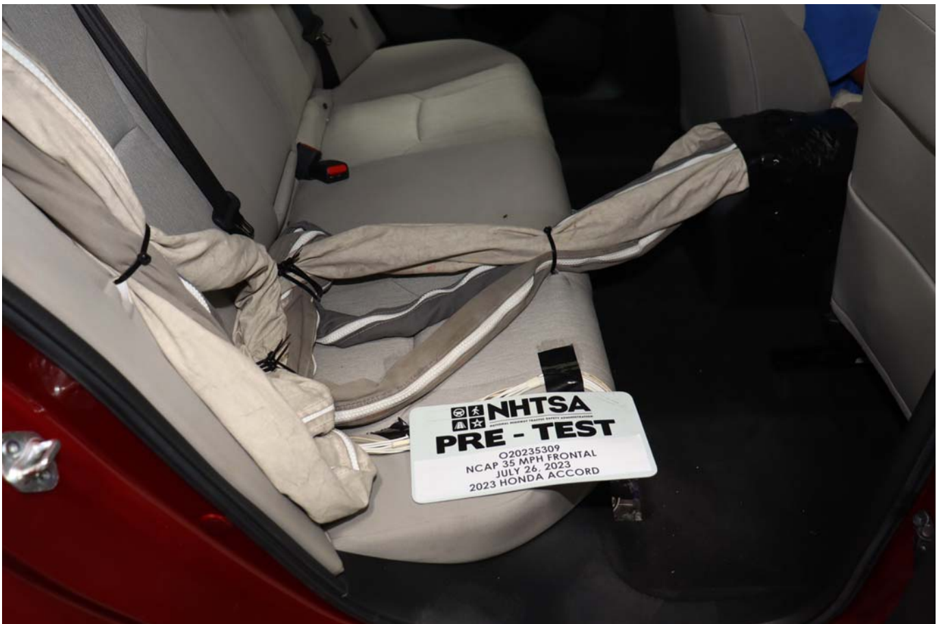
Photo No. 028 - Pre-Test Dummy Cable Routing
