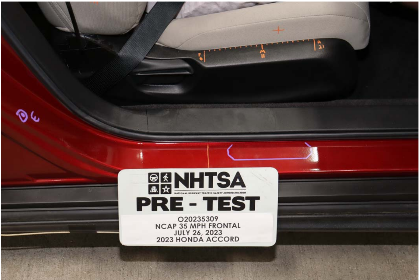
Photo No. 059 - Pre-Test Passenger's Seat Fore-Aft Markings
