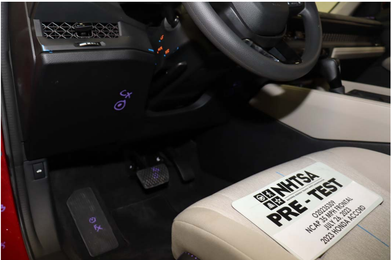
Photo No. 044 - Pre-Test Driver's Side Knee Bolster
