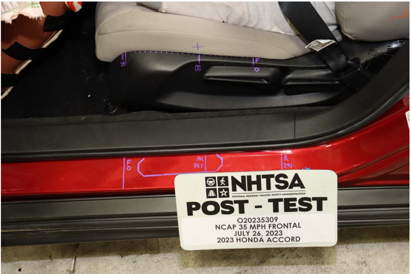
Photo No. 037 - Post-Test Driver's Seat Fore-Aft Markings
