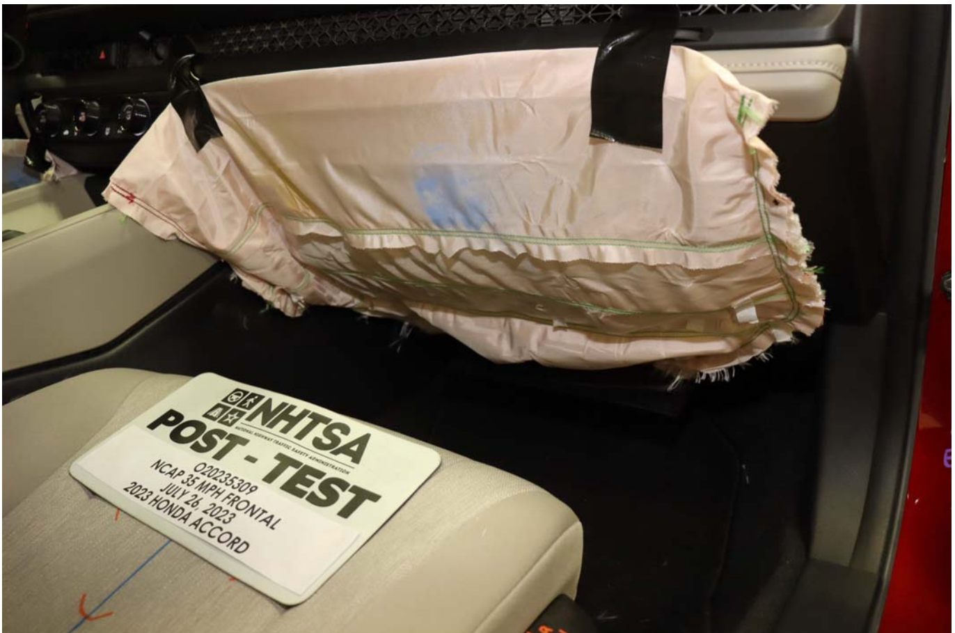
Photo No. 068 - Post-Test Passenger's Side Knee Bolster
