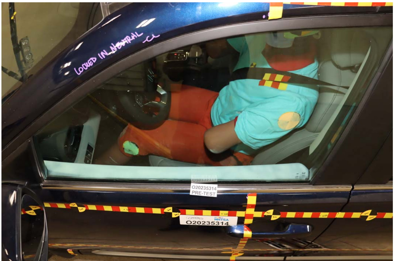
Photo No. 042 - Pre-Test Driver Dummy and Door Clearance View
