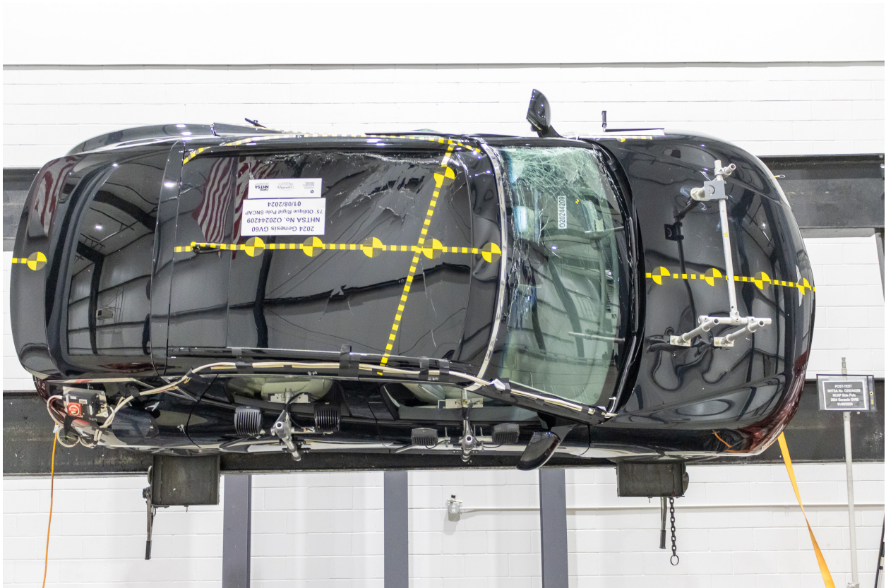
Figure A-66: FMVSS No. 301 Static Rollover 90 Degrees
