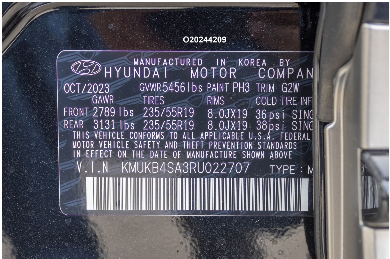
Figure A-57: Close-Up View of Vehicle's Certification Label
