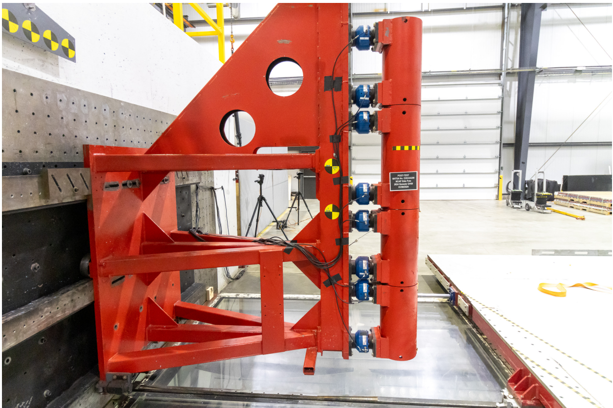
Figure A-62: Post-Test Pole Barrier Side View
