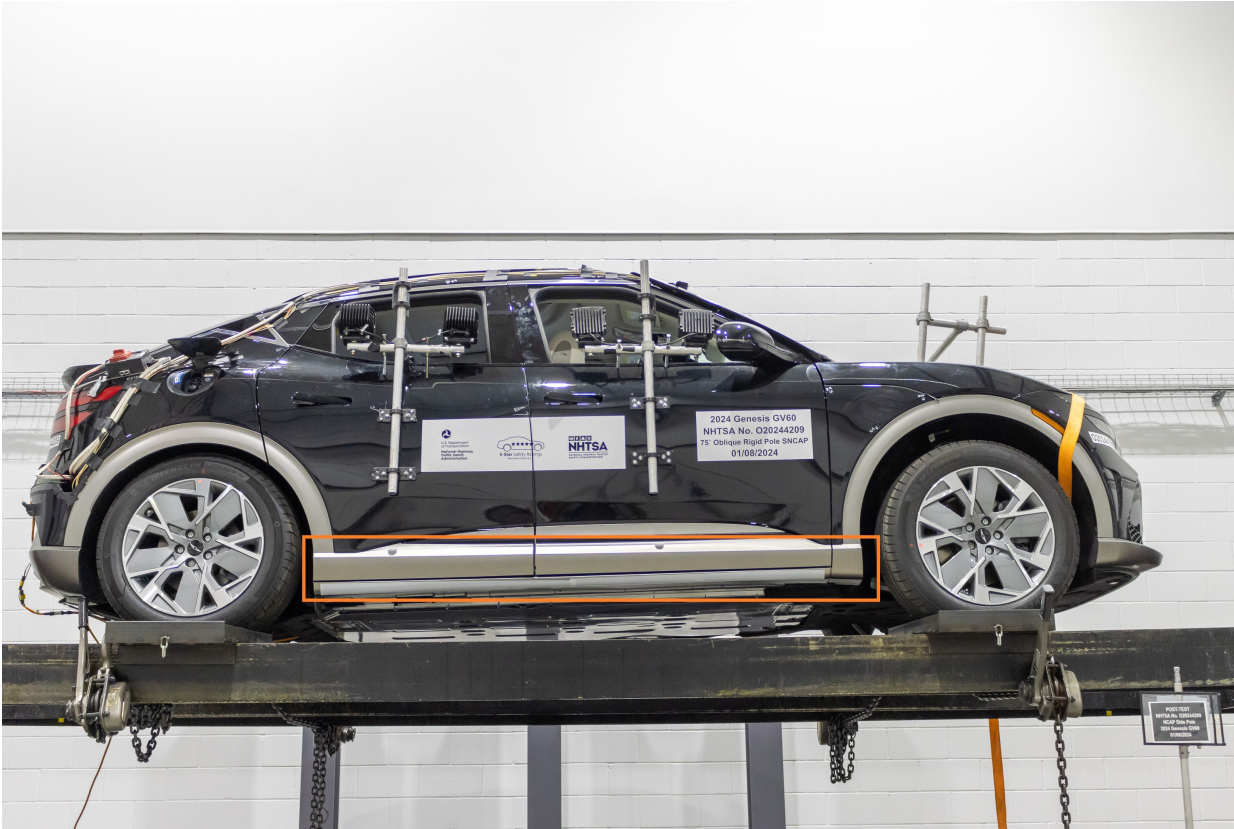
Figure 305-31: FMVSS No. 305 Static Rollover 360 Degrees
