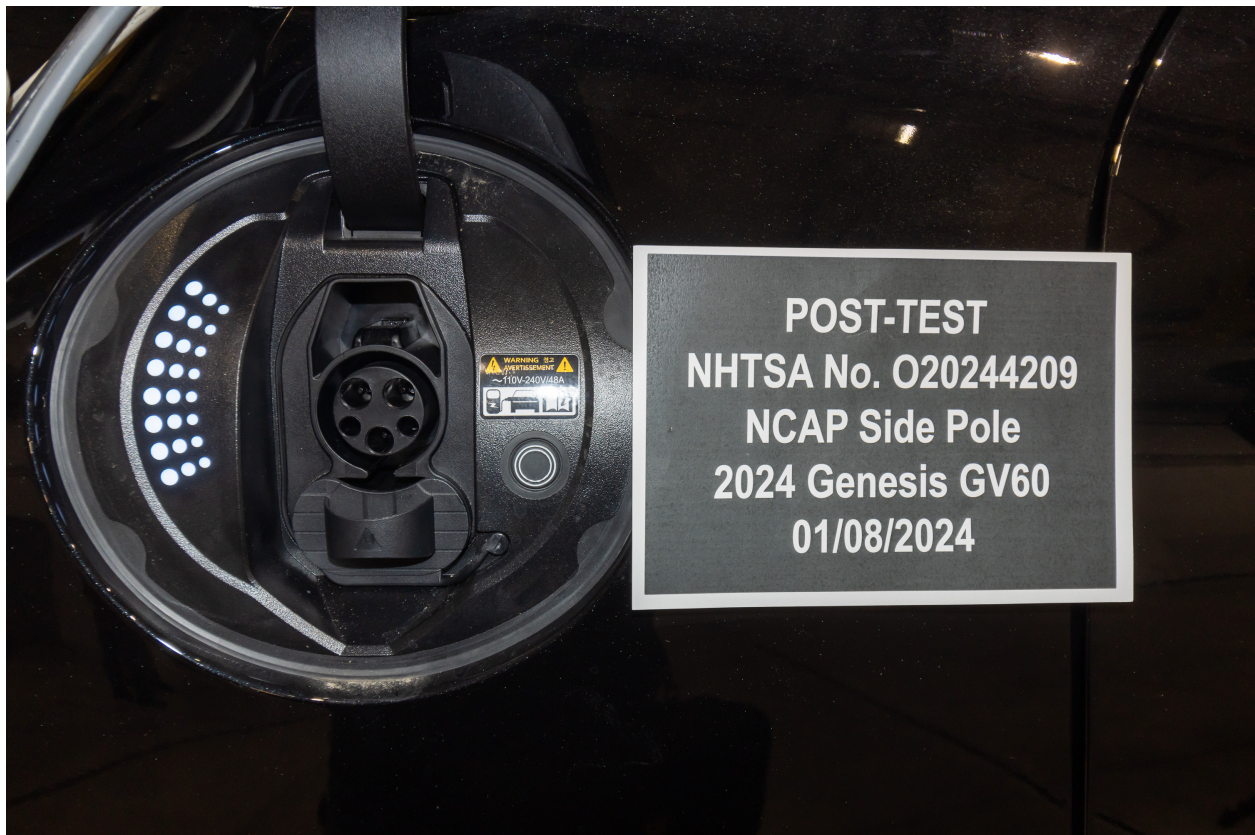
Figure A-56: Post-Test Charging Port
