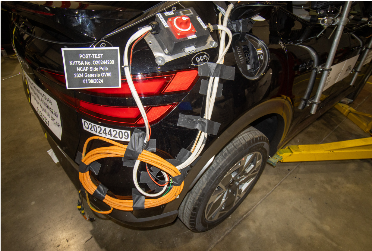
Figure 305-25: Post-Impact View of Installed Test Interface Port
