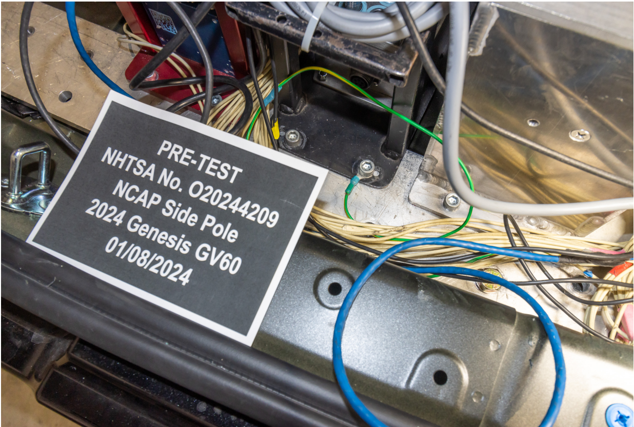
Figure 305-21: Pre-Impact View of Ground Lead Attached
