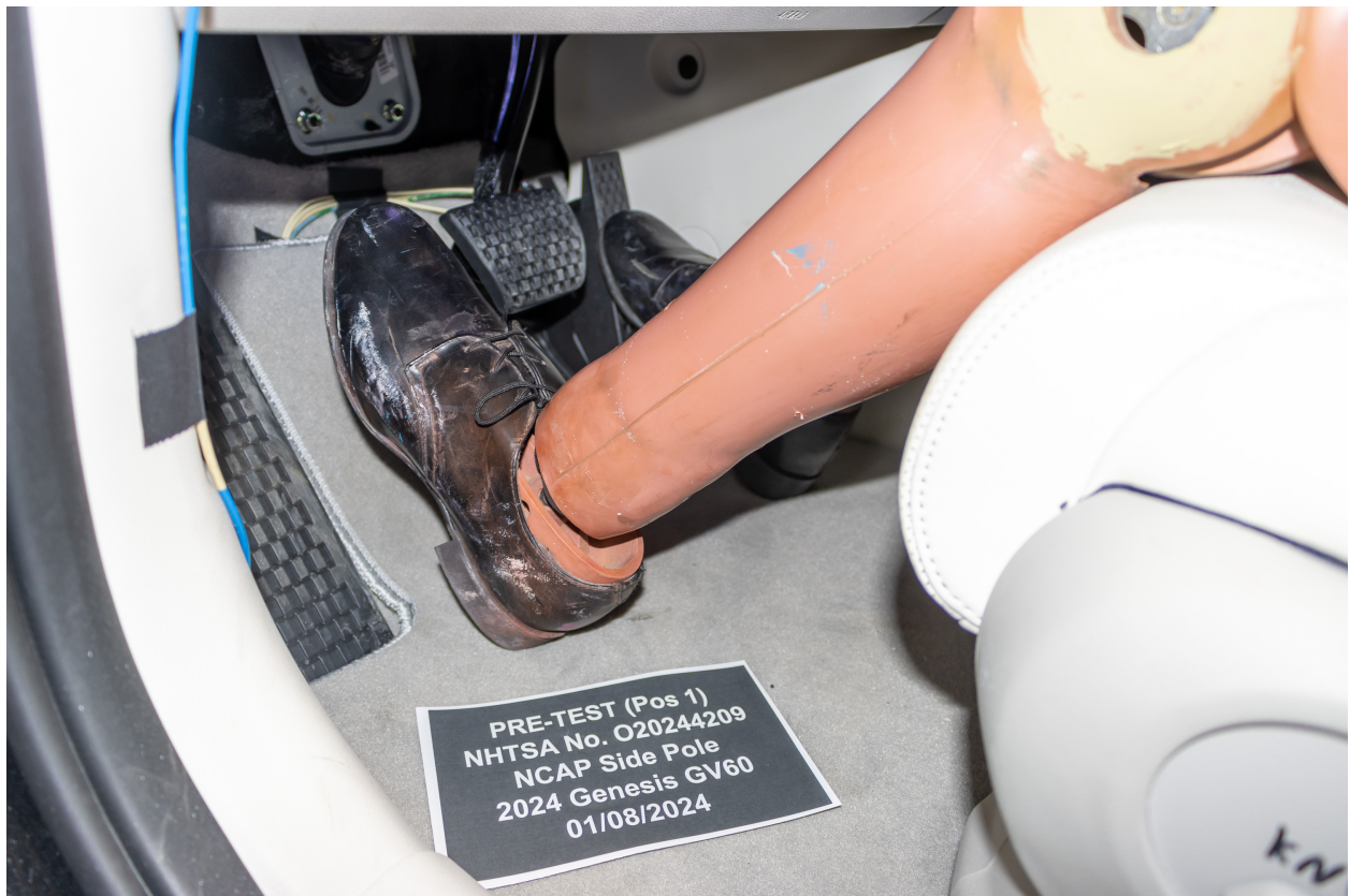
Figure A-32: Pre-Test Placement of Dummy's Feet
