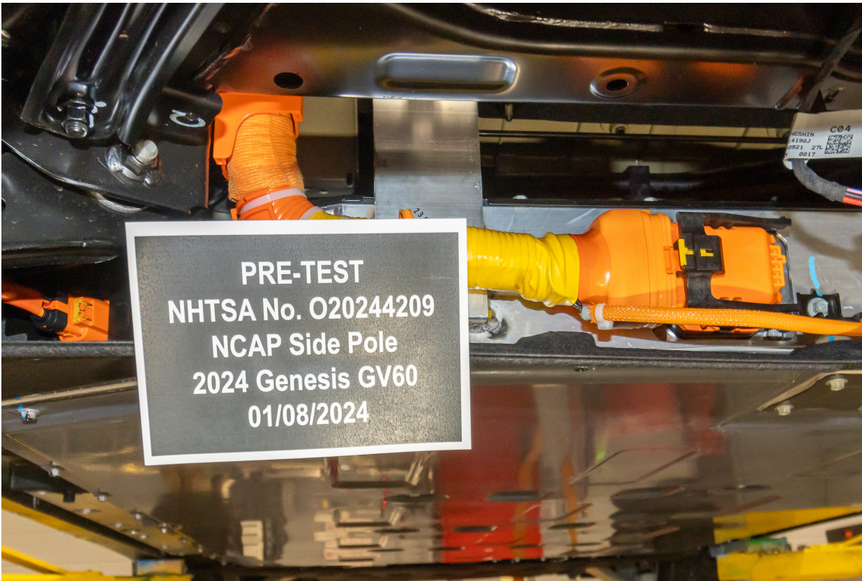
Figure 305-22: Pre-Impact View of High Voltage Leads Attached
