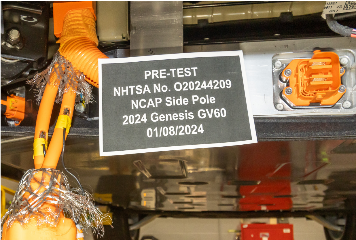
Figure 305-18: Pre-Impact View of High Voltage Interconnects
