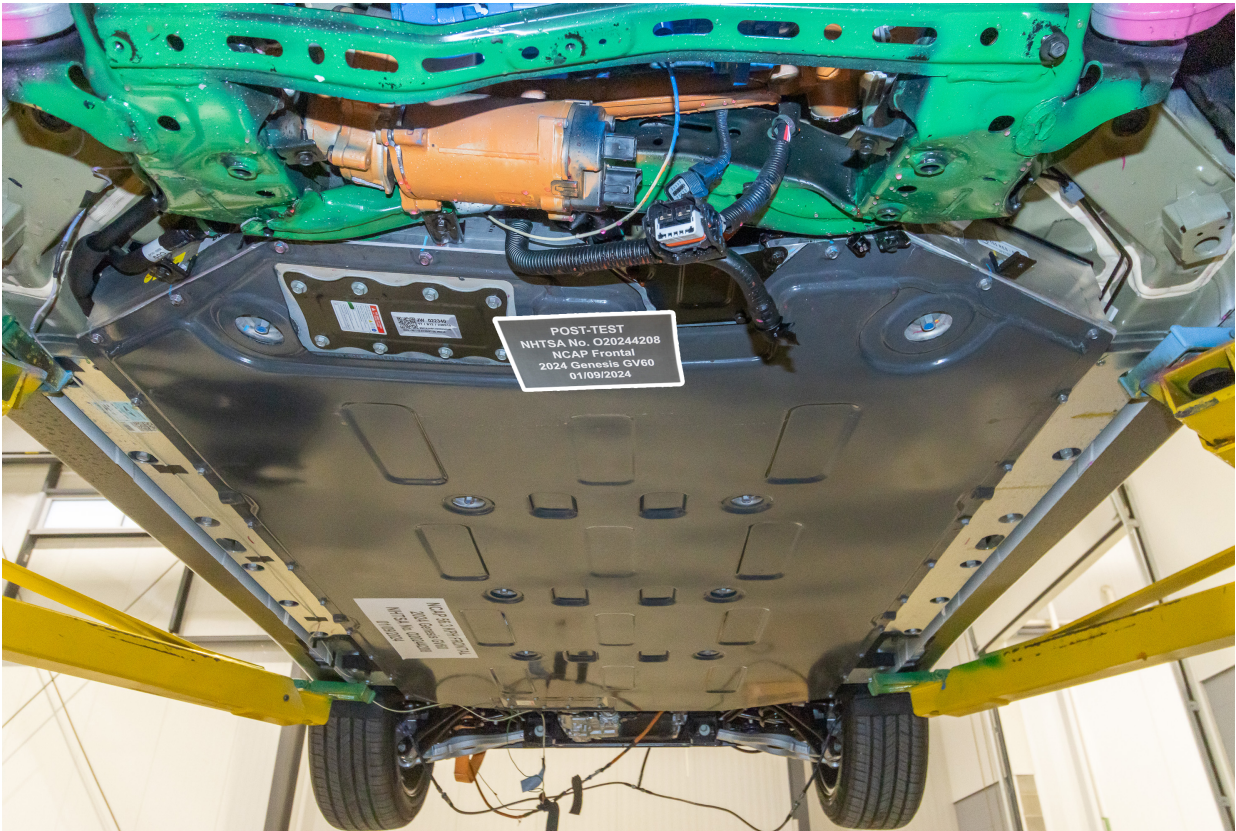
Figure 305-10: Post-Impact Front View of Propulsion Battery
