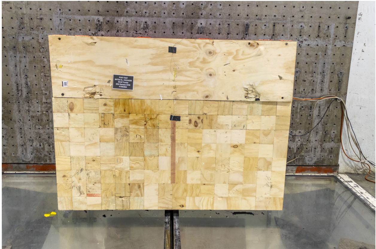
Figure A-3: Post-Test Load Cell Wall
