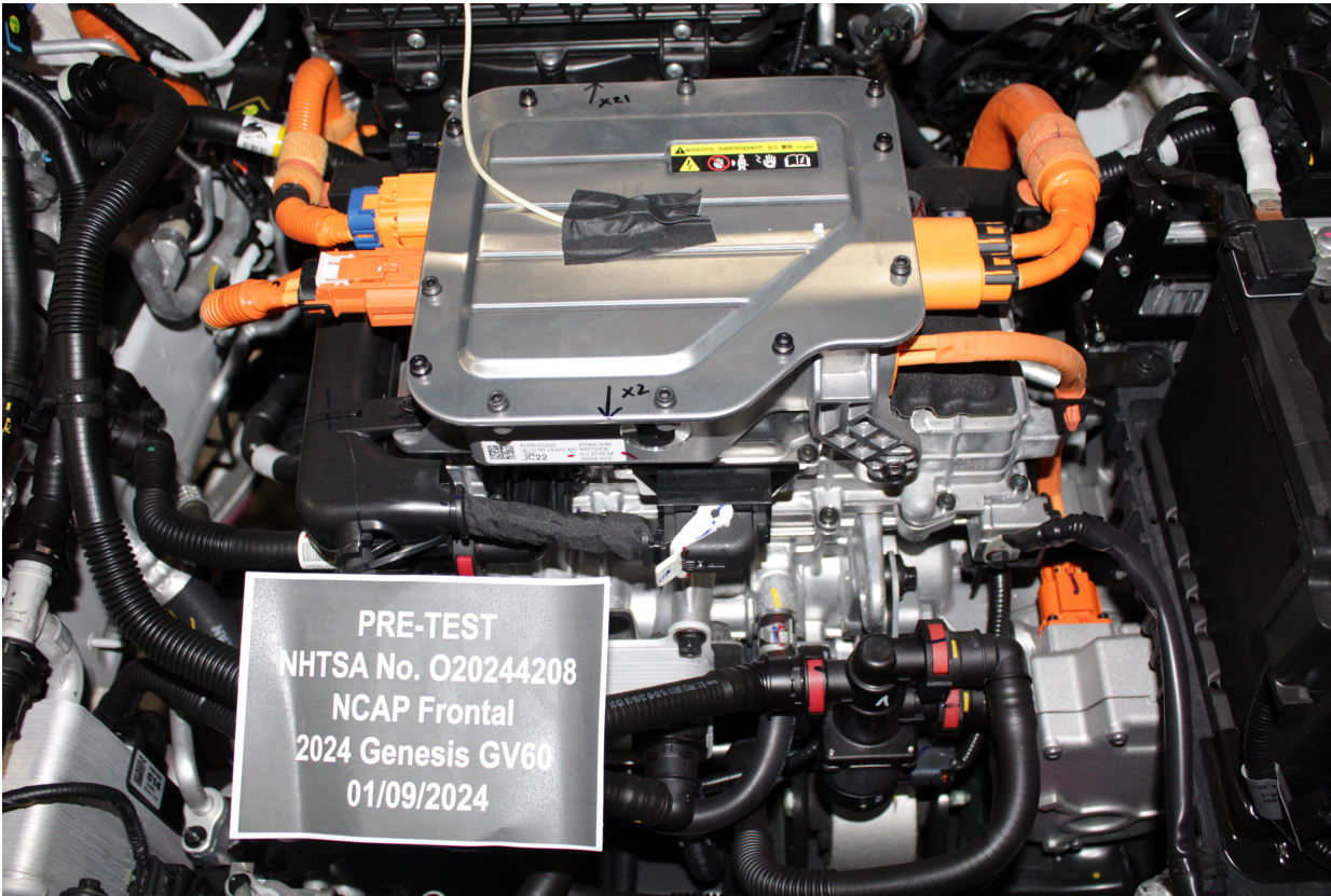
Figure 305-18: Pre-Impact View of High Voltage Interconnects
