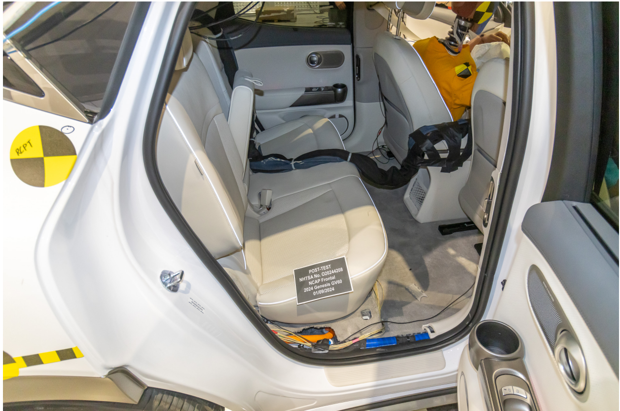
Figure A-29: Post-Test Dummy Cable Routing
