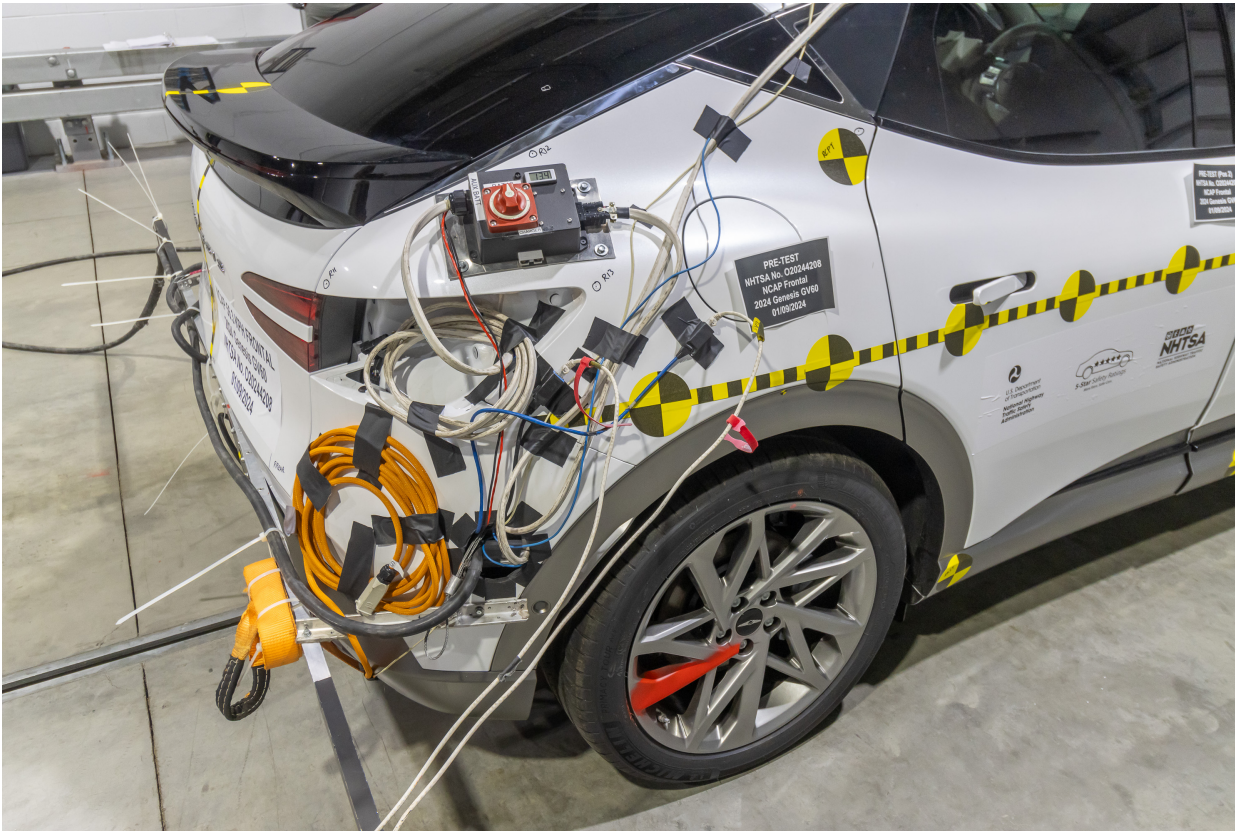
Figure 305-24: Pre-Impact View of Installed Test Interface Port
