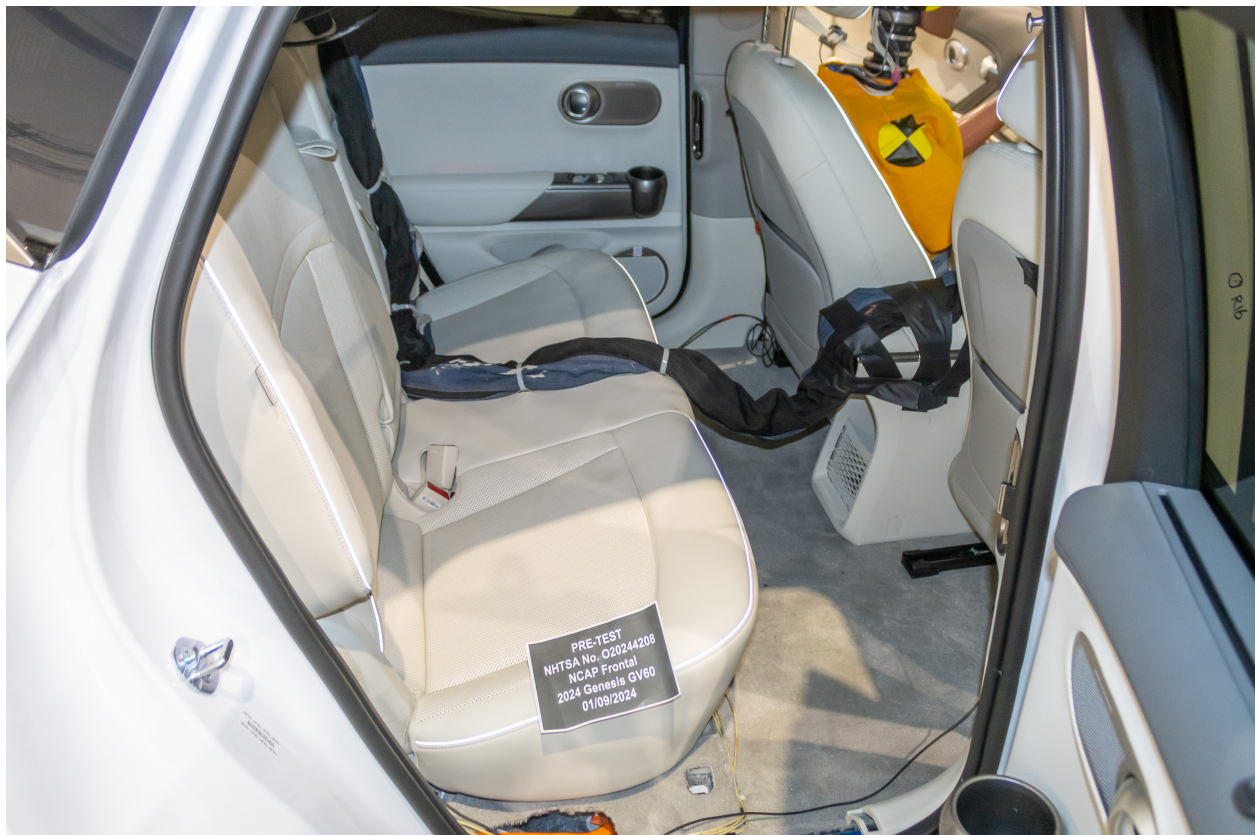
Figure A-28: Pre-Test Dummy Cable Routing
