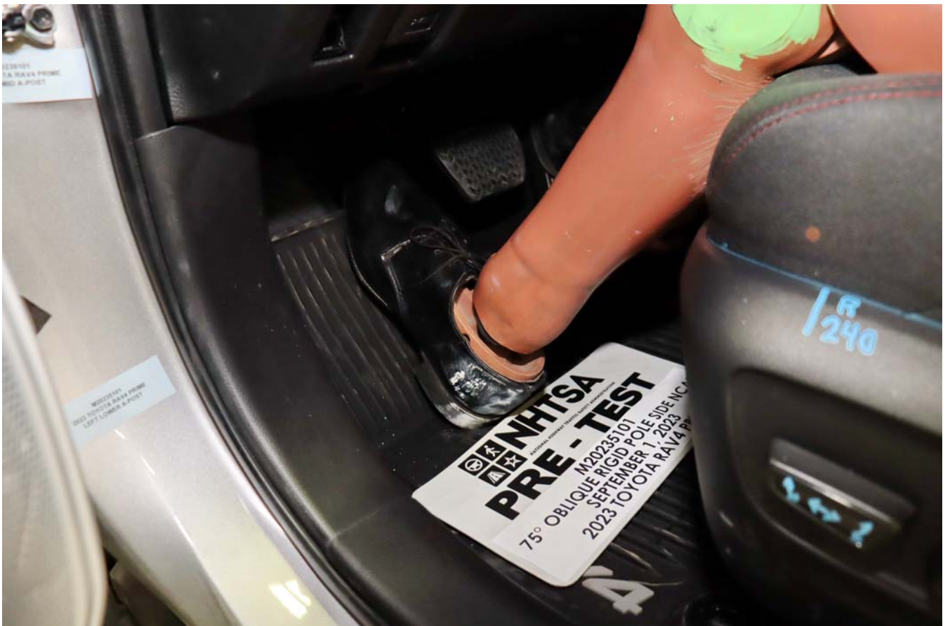
Photo No. 032 - Pre-Test Placement of Dummy's Feet
