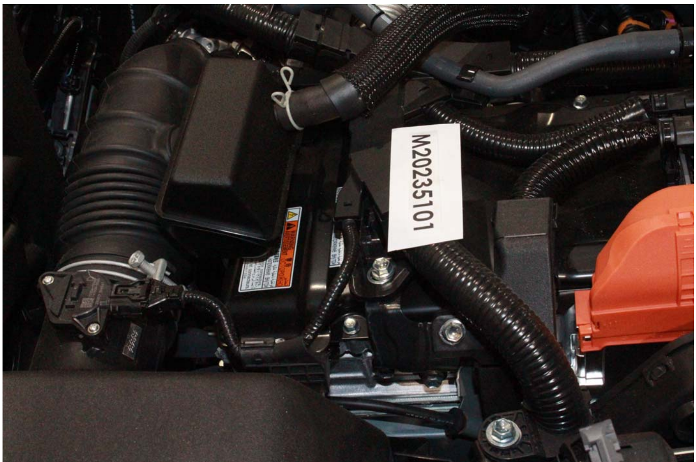
Photo No. 305-02 - Power Inverter Warning Label
