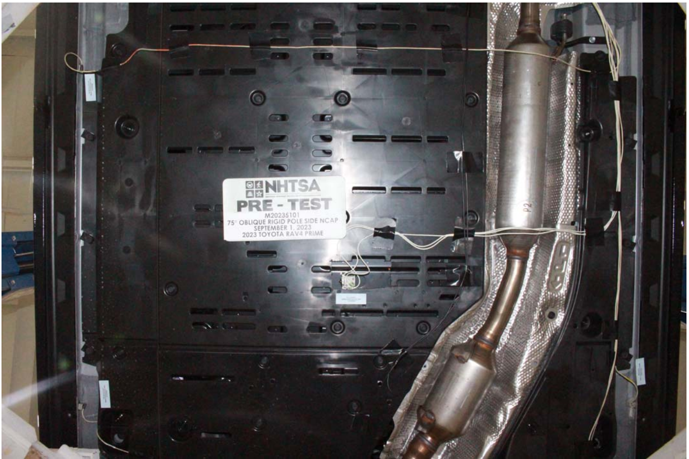
Photo No. 305-09 - Pre-Impact View of Propulsion Battery
