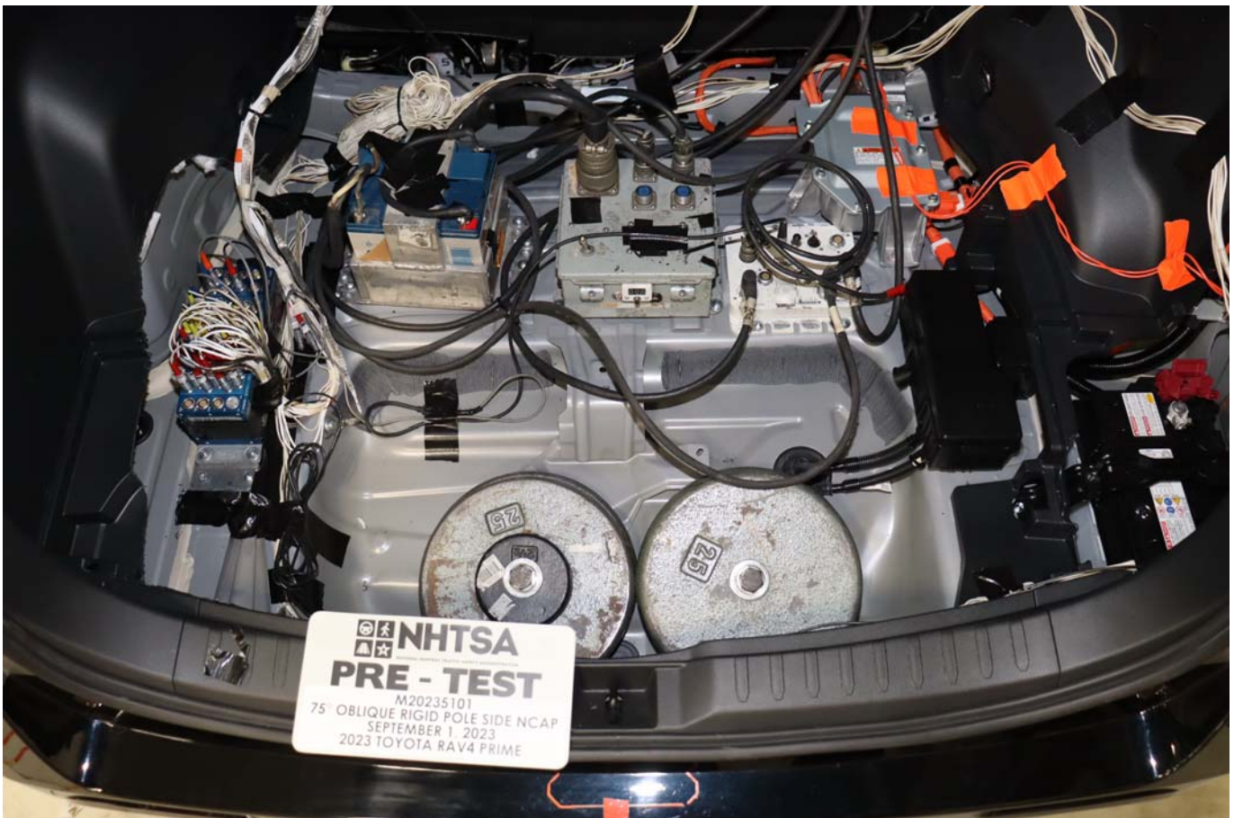
Photo No. 063 - Pre-Test Ballast View
