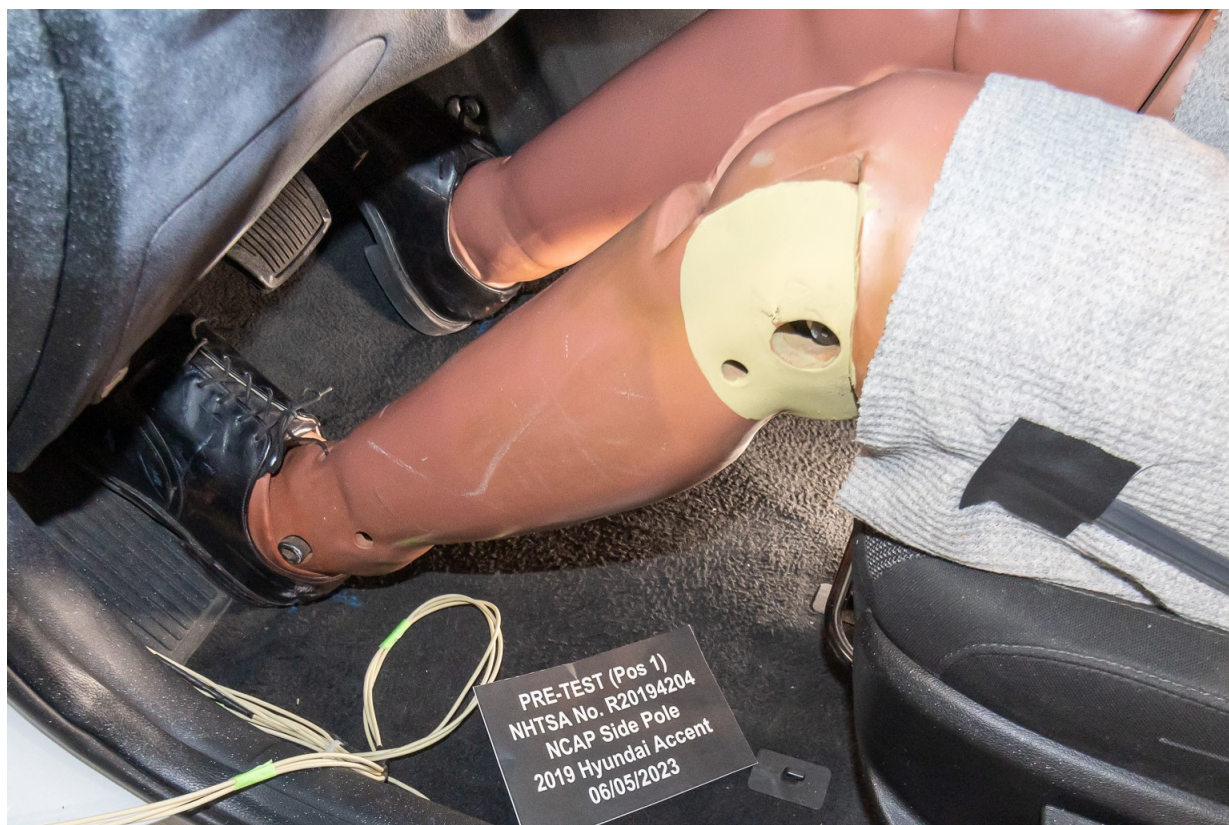
Figure A-32: Pre-Test Placement of Dummy's Feet
