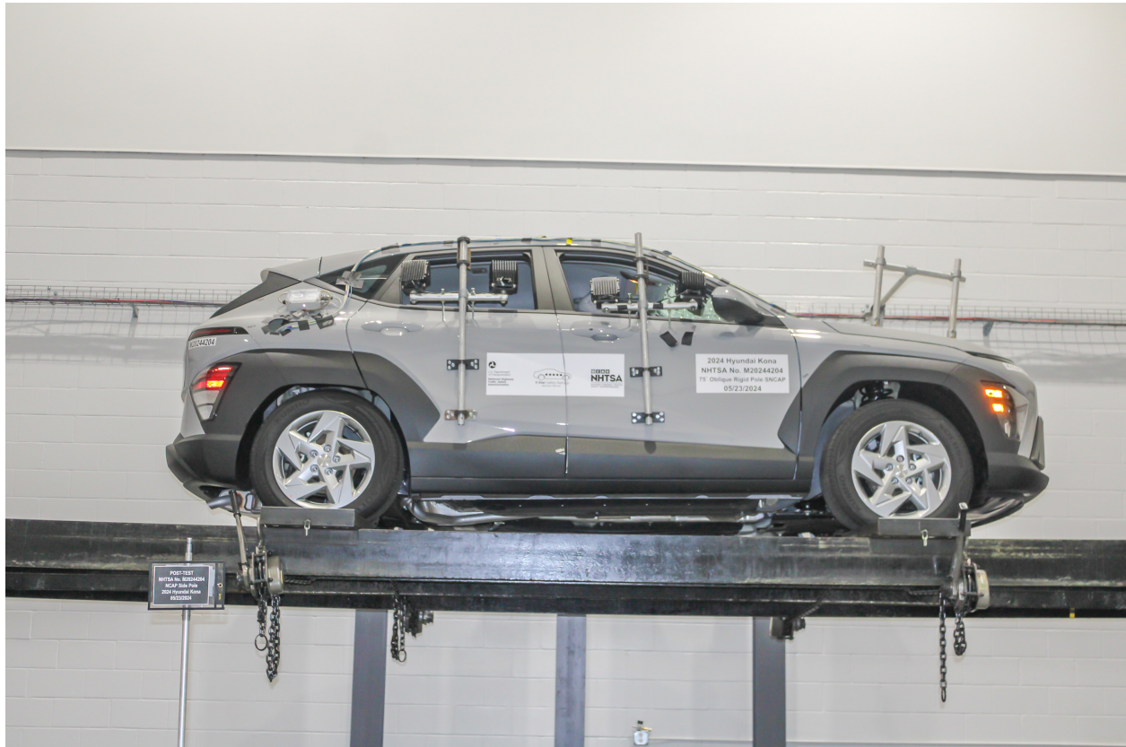
Figure A-69: FMVSS No. 301 Static Rollover 360 Degrees
