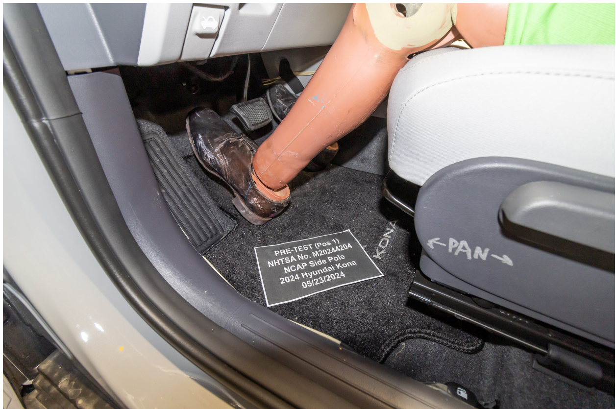
Figure A-32: Pre-Test Placement of Dummy's Feet
