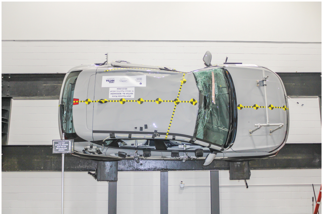
Figure A-68: FMVSS No. 301 Static Rollover 270 Degrees
