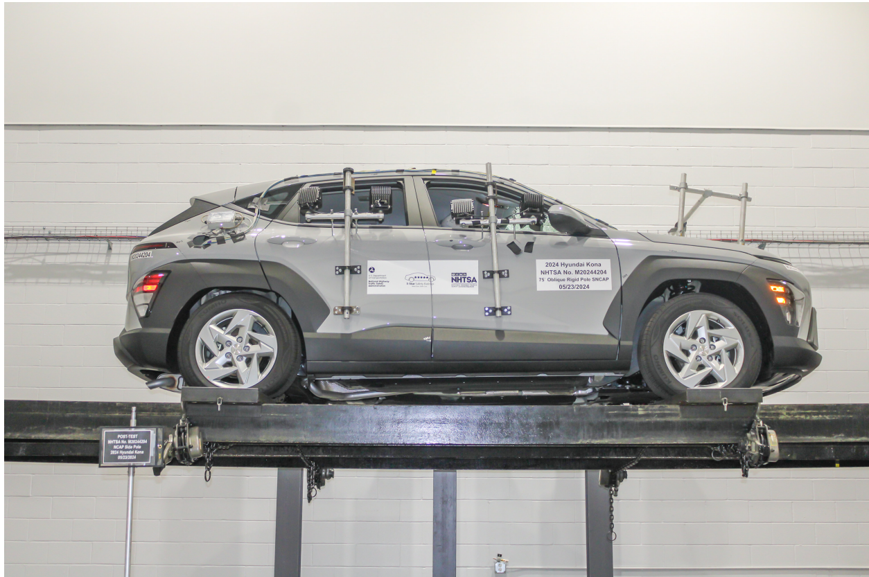
Figure A-65: FMVSS No. 301 Static Rollover 0 Degrees
