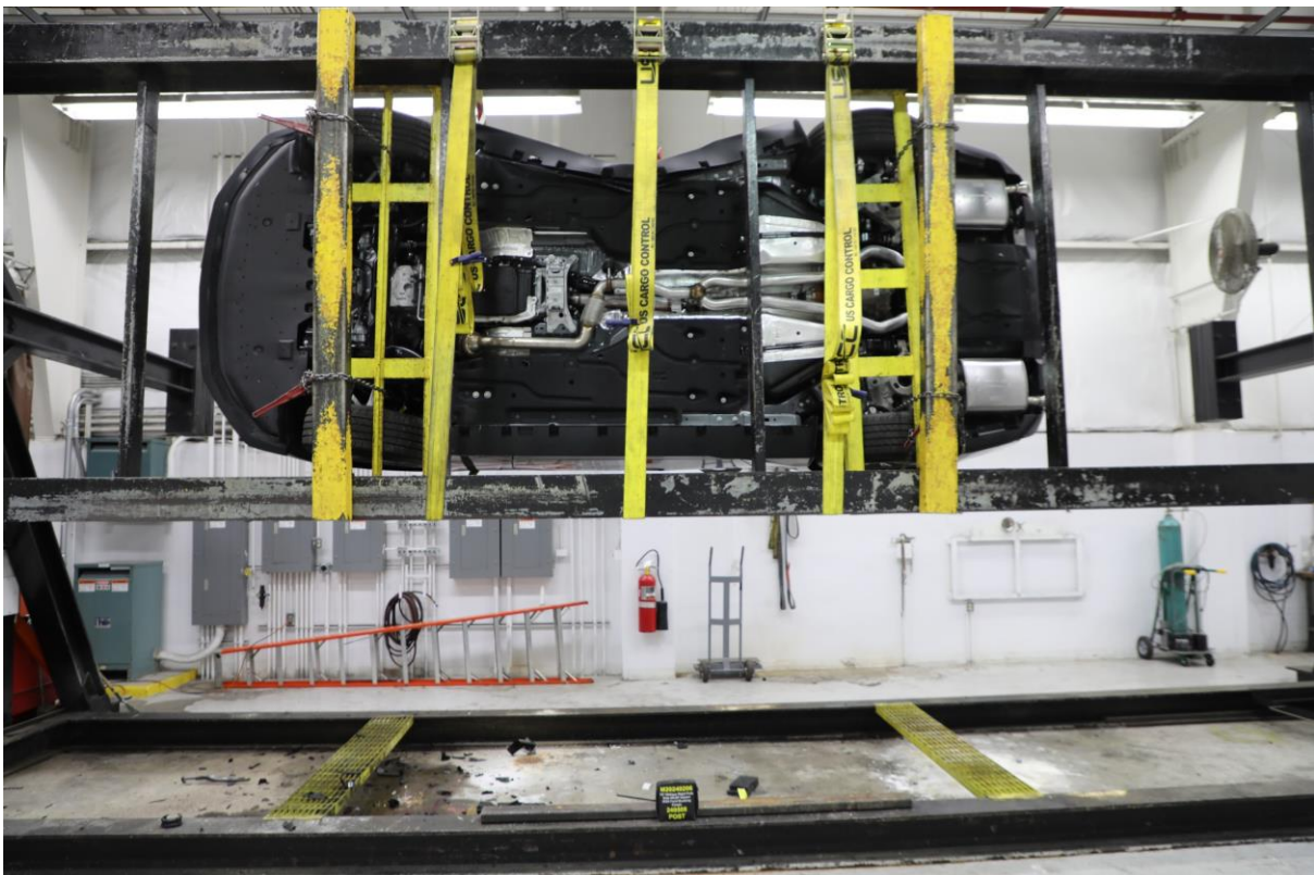
No. 068 FMVSS No. 301 Static Rollover 270 Degrees
