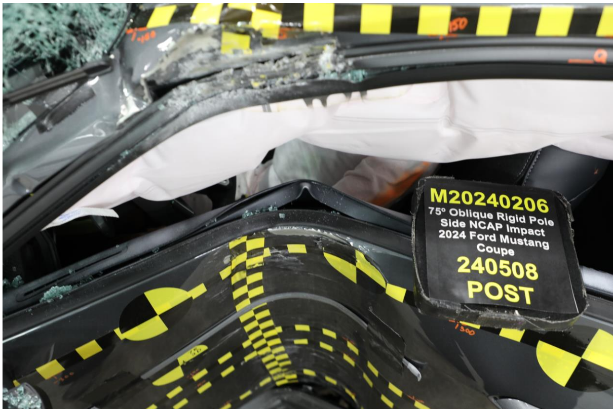
No. 041 Post-Test Dummy and Door Clearance View
