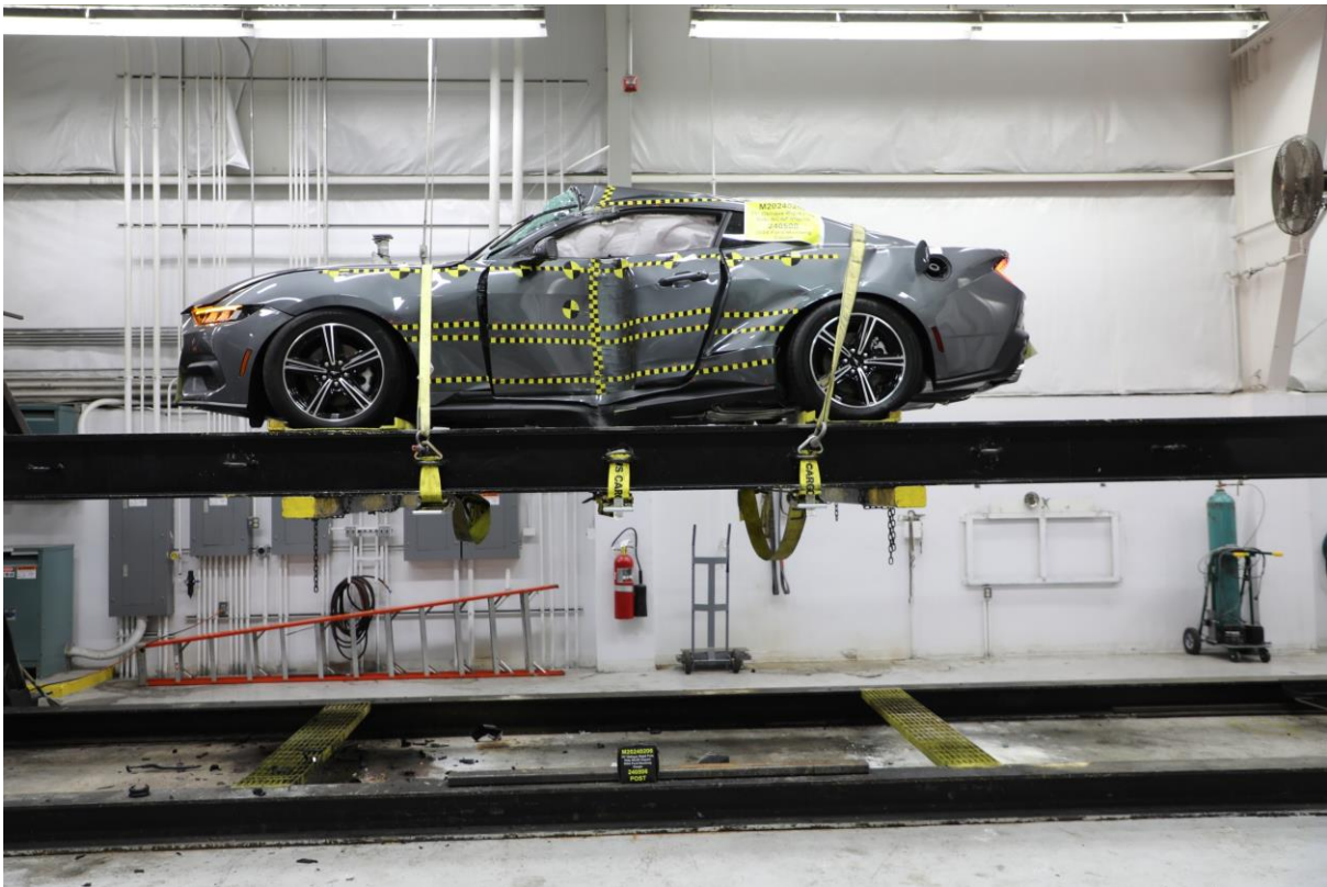
No. 069 FMVSS No. 301 Static Rollover 360 Degrees
