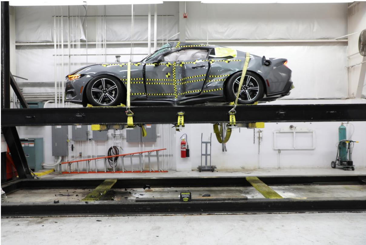
No. 065 FMVSS No. 301 Static Rollover 0 Degrees
