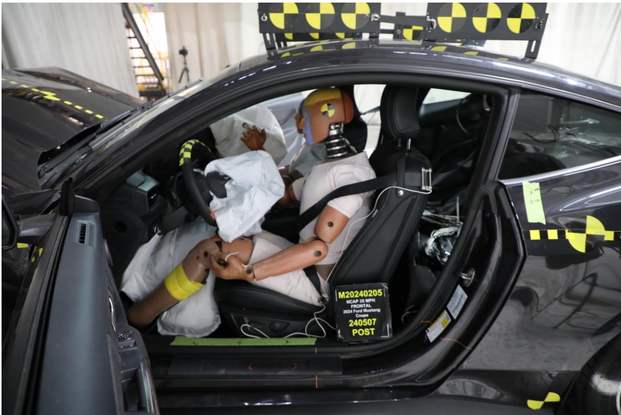
035 Post-Test Driver Dummy and Vehicle Interior View
