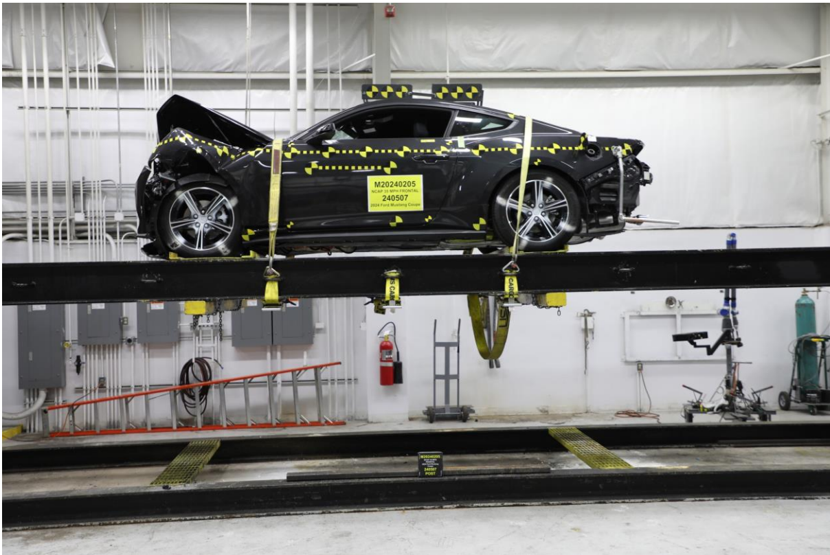
077 Vehicle at 0° on Static Rollover Device
