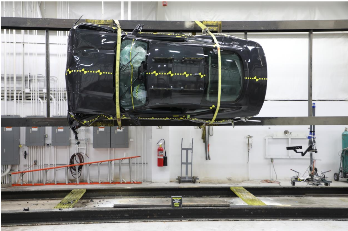
078 Vehicle at 90° on Static Rollover Device
