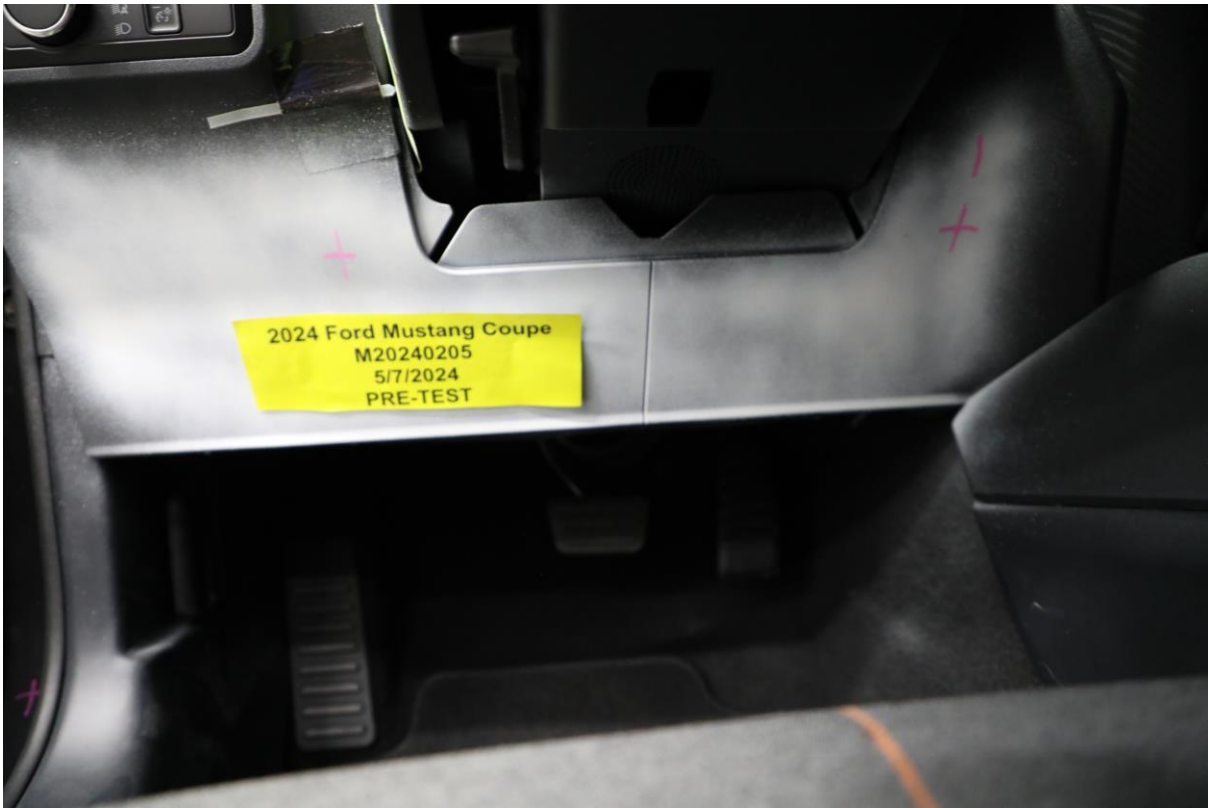
044 Pre-Test Driver's Side Knee Bolster
