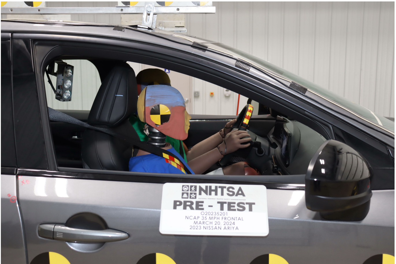
Photo No. 055 - Pre-Test Passenger Dummy Window View
