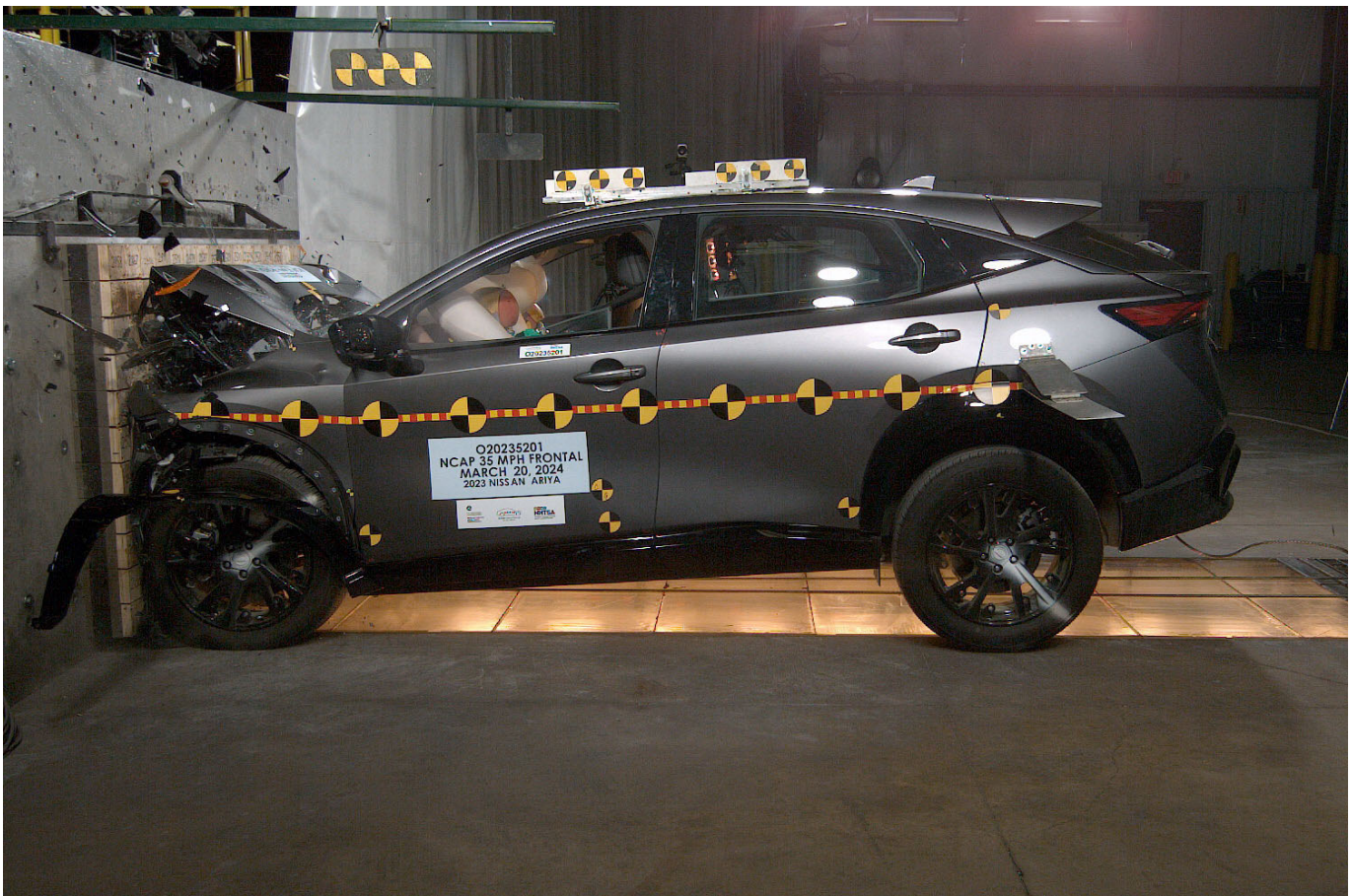
Photo No. 082 - 2023 Nissan Ariya Engage AWD 5-Door SUV Frontal Impact Event
