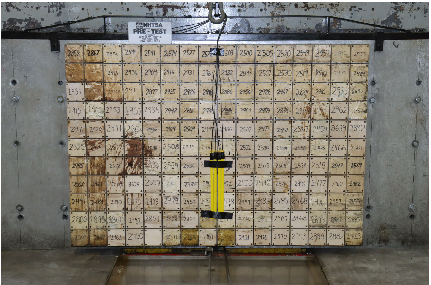
Photo No. 002 - Pre-Test Load Cell Wall
