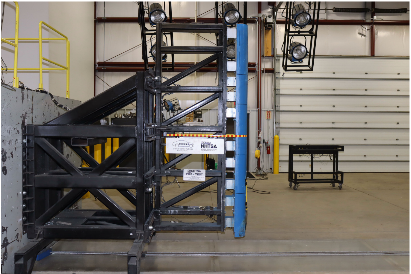
Photo No. 061 - Pre-Test Pole Barrier Side View
