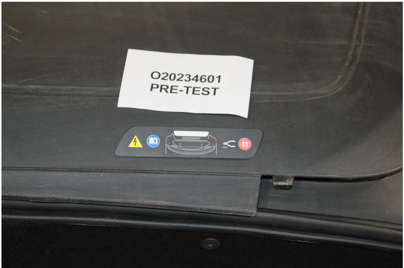
Photo No. 305-03 - First Responder Warning Label
