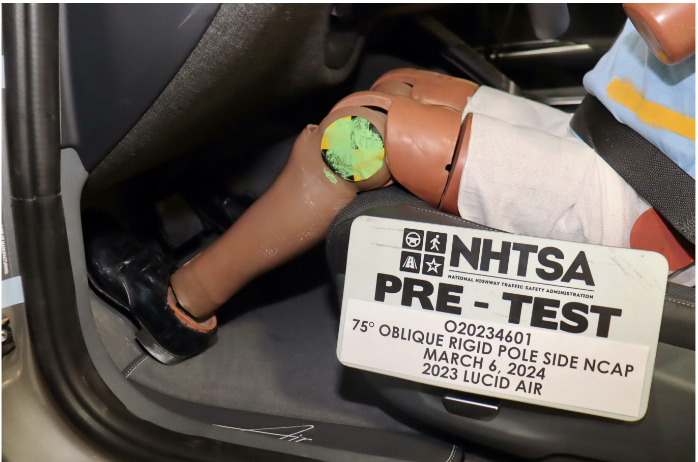
Photo No. 032 - Pre-Test Placement of Dummy's Feet
