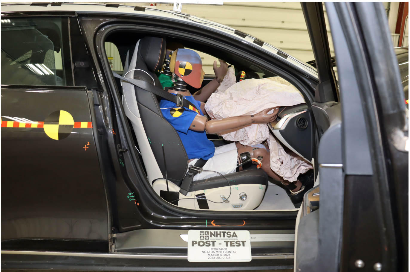
Photo No. 058 - Post-Test Passenger Dummy and Vehicle Interior View
