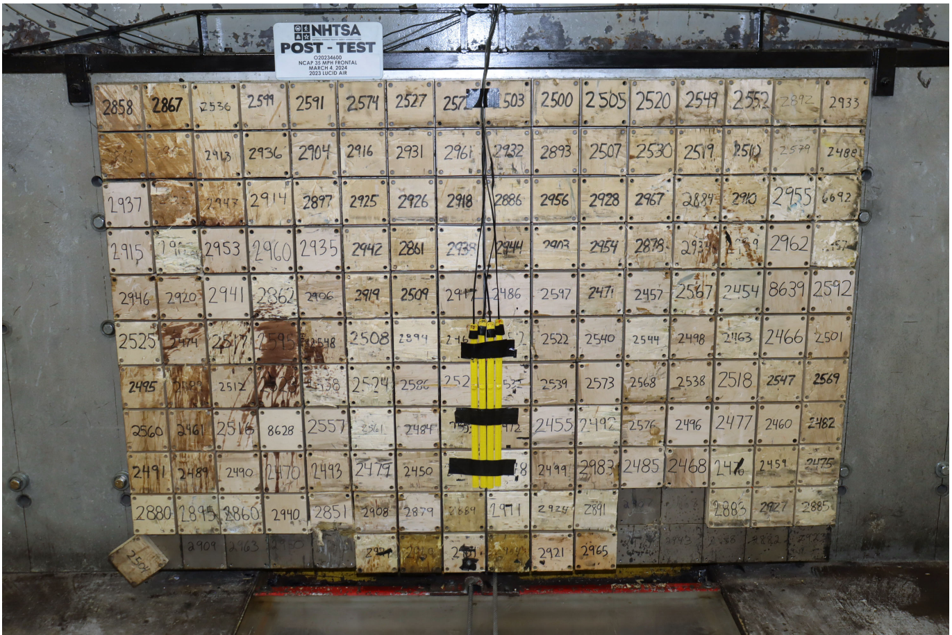
Photo No. 003 - Post-Test Load Cell Wall
