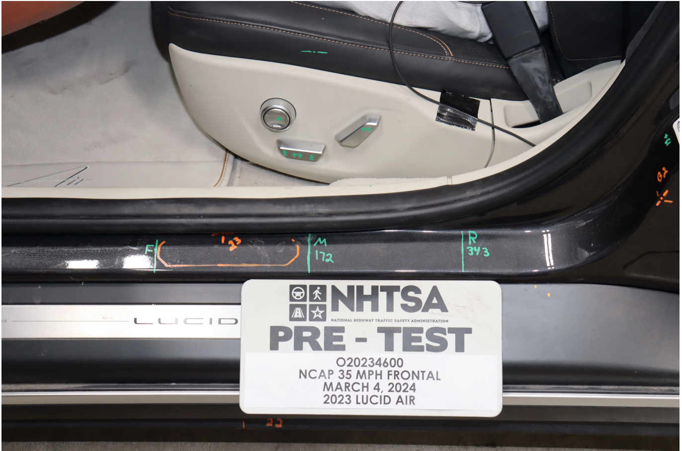
Photo No. 036 - Pre-Test Driver's Seat Fore-Aft Markings
