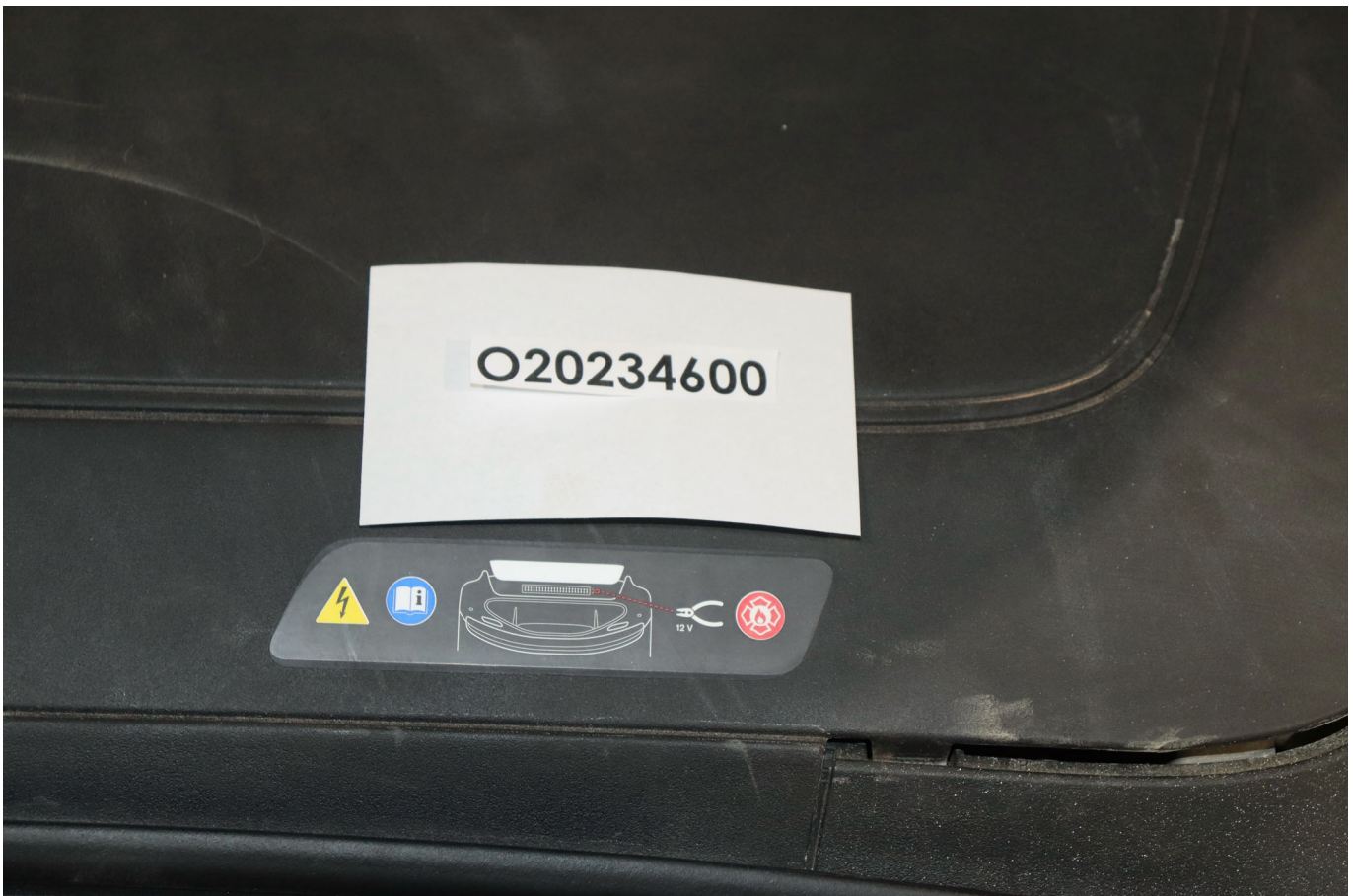
Photo No. 305-03 - First Responder Warning Label
