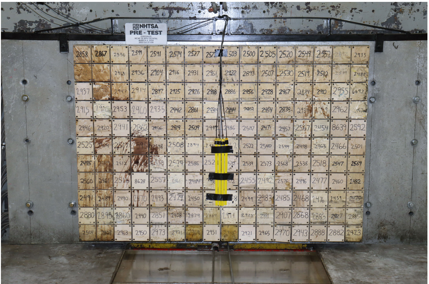
Photo No. 002 - Pre-Test Load Cell Wall
