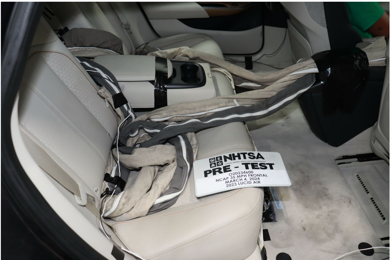
Photo No. 028 - Pre-Test Dummy Cable Routing
