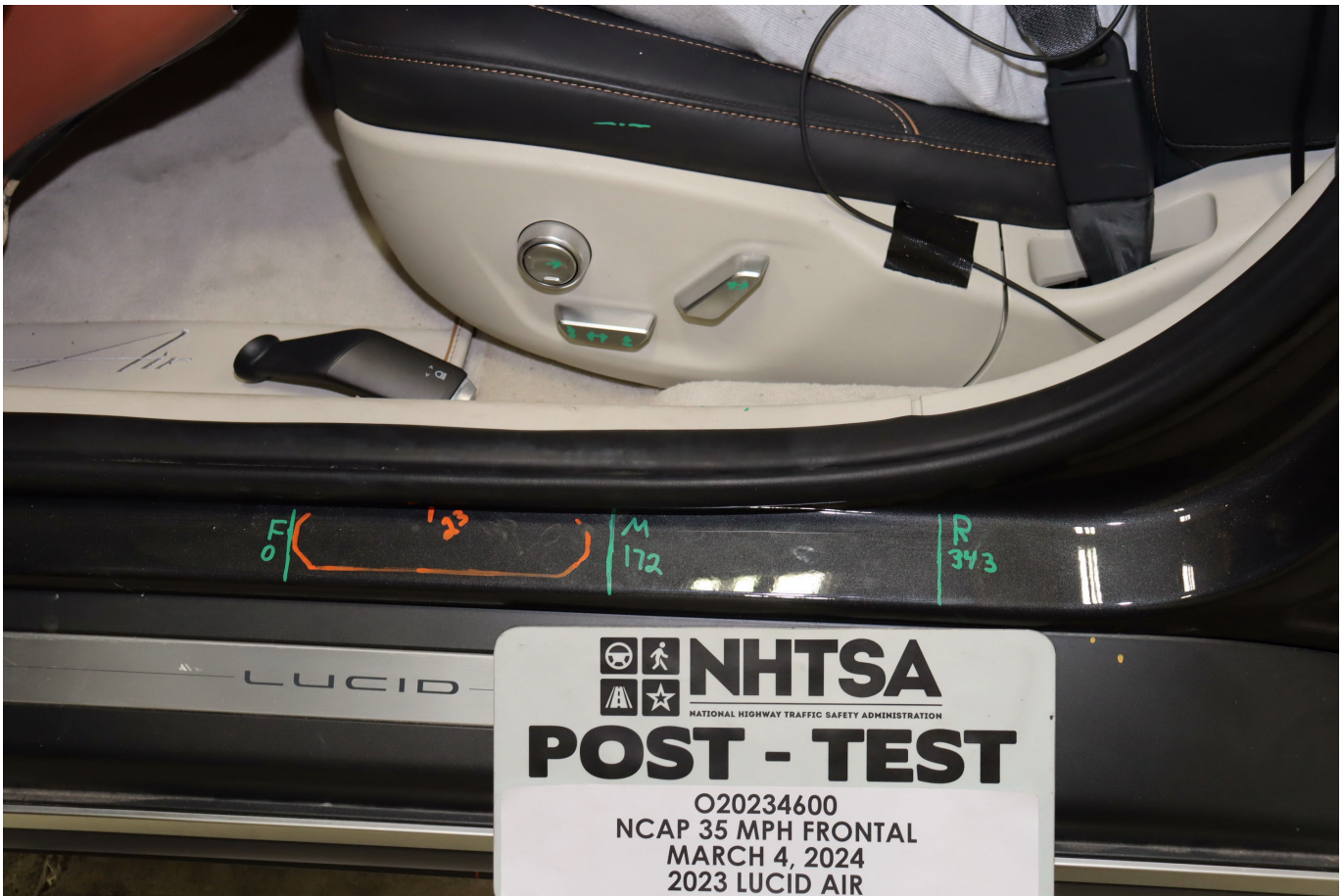
Photo No. 037 - Post-Test Driver's Seat Fore-Aft Markings
