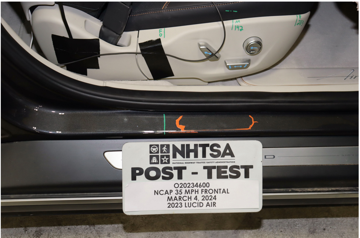
Photo No. 060 - Post-Test Passenger's Seat Fore-Aft Markings
