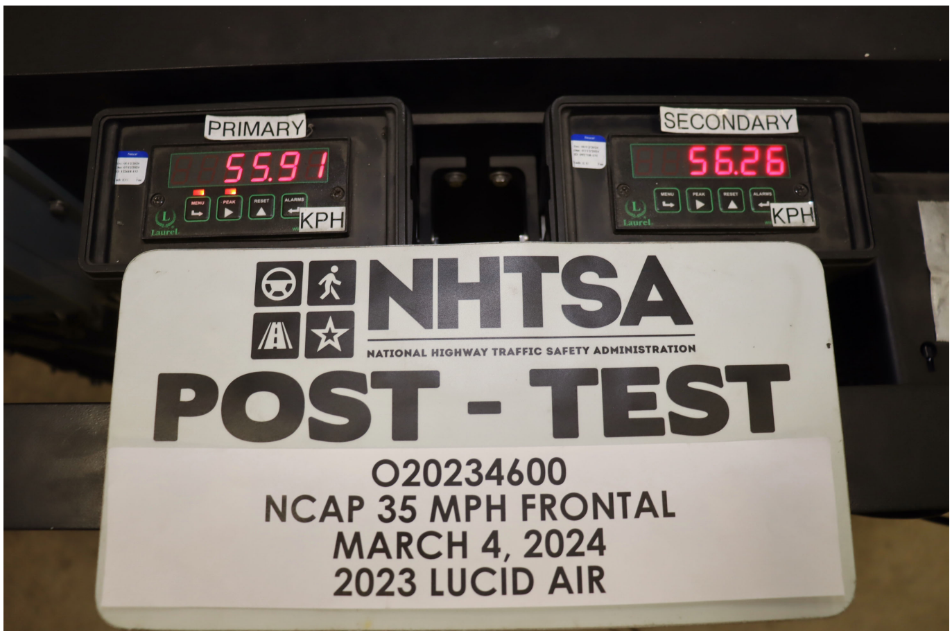
Photo No. 076 - Post-Test Speed Trap Read-Out
