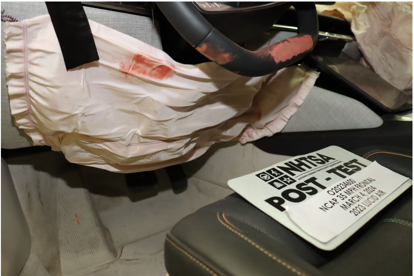
Photo No. 045 - Post-Test Driver's Side Knee Bolster
