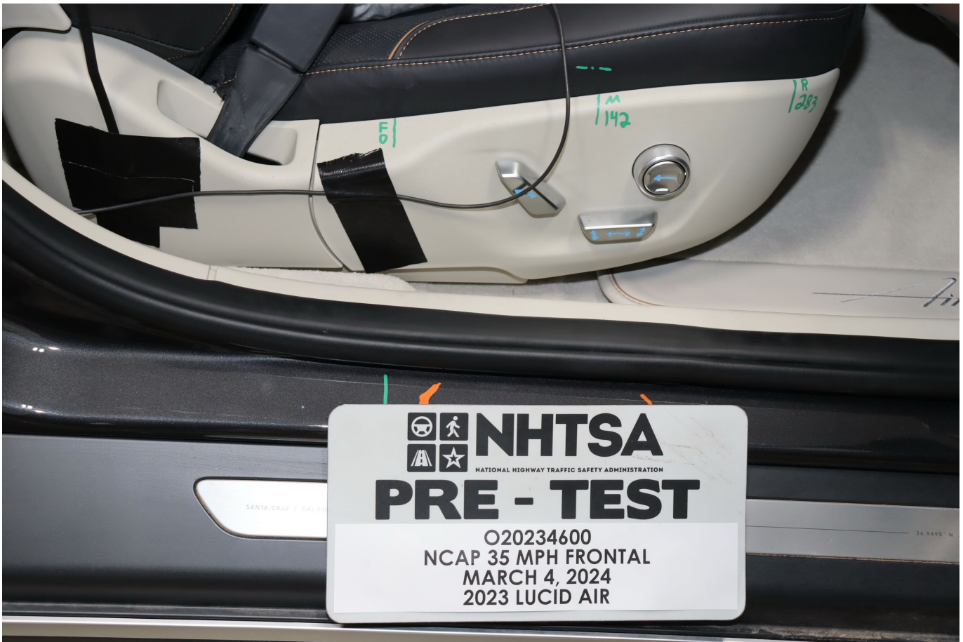
Photo No. 059 - Pre-Test Passenger's Seat Fore-Aft Markings
