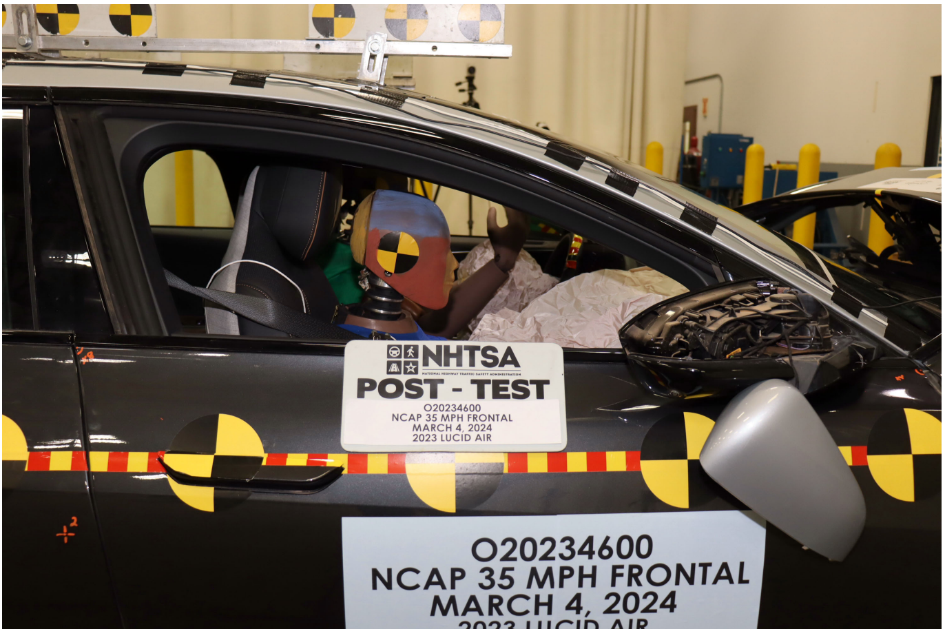
Photo No. 056 - Post-Test Passenger Dummy Window View
