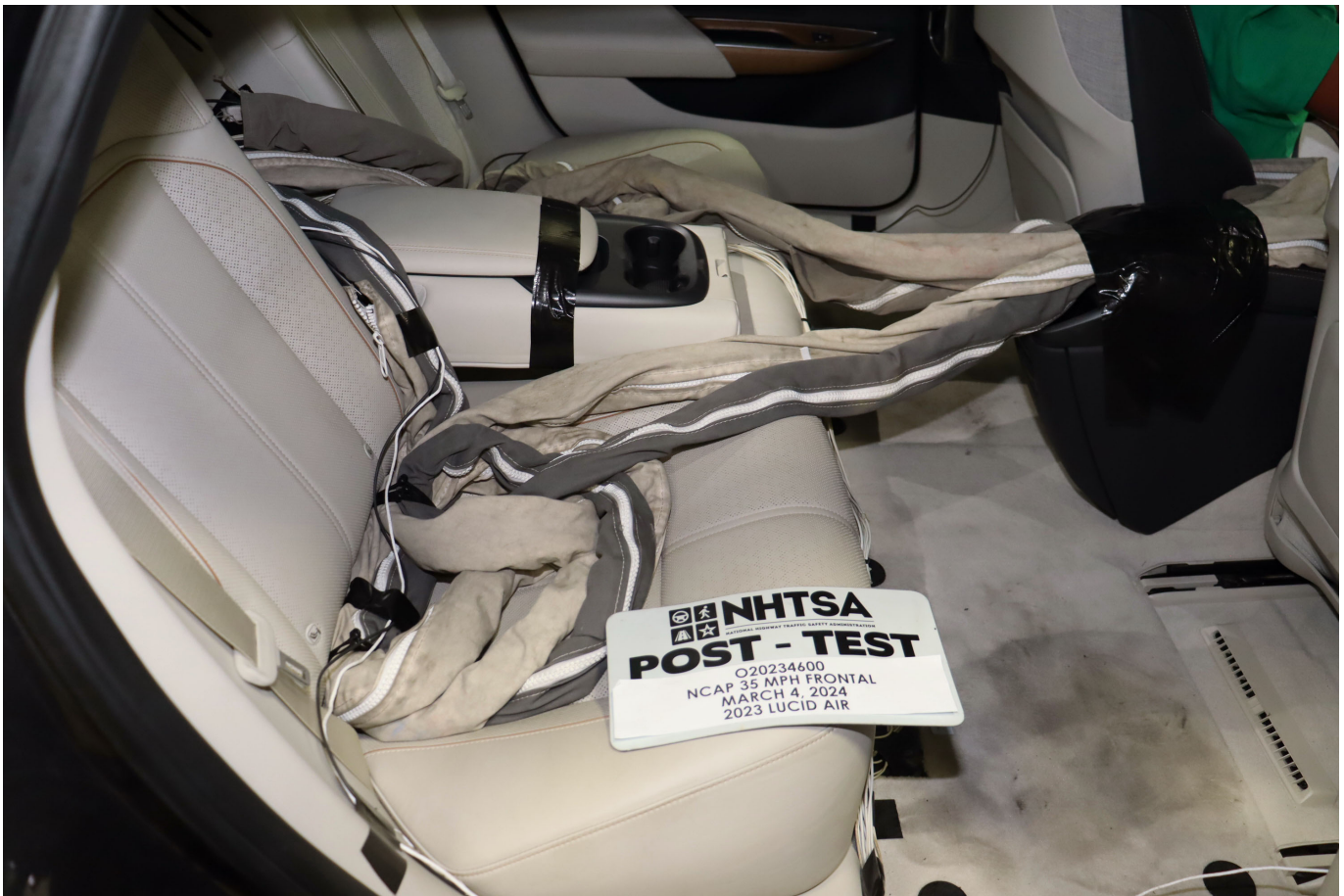
Photo No. 029 - Post-Test Dummy Cable Routing
