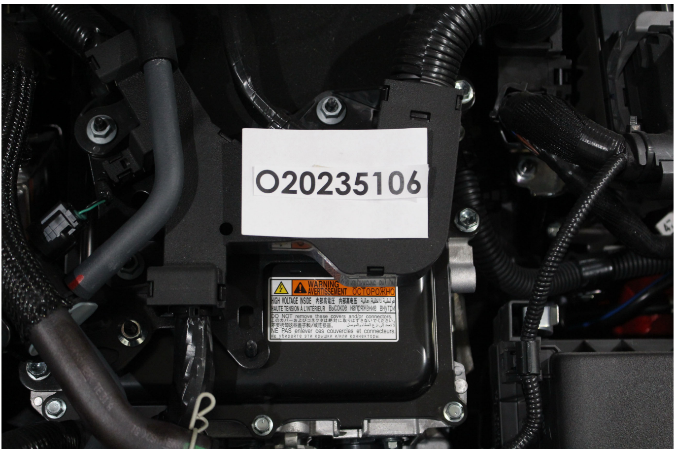
Photo No. 305-02 - Power Inverter Warning Label
