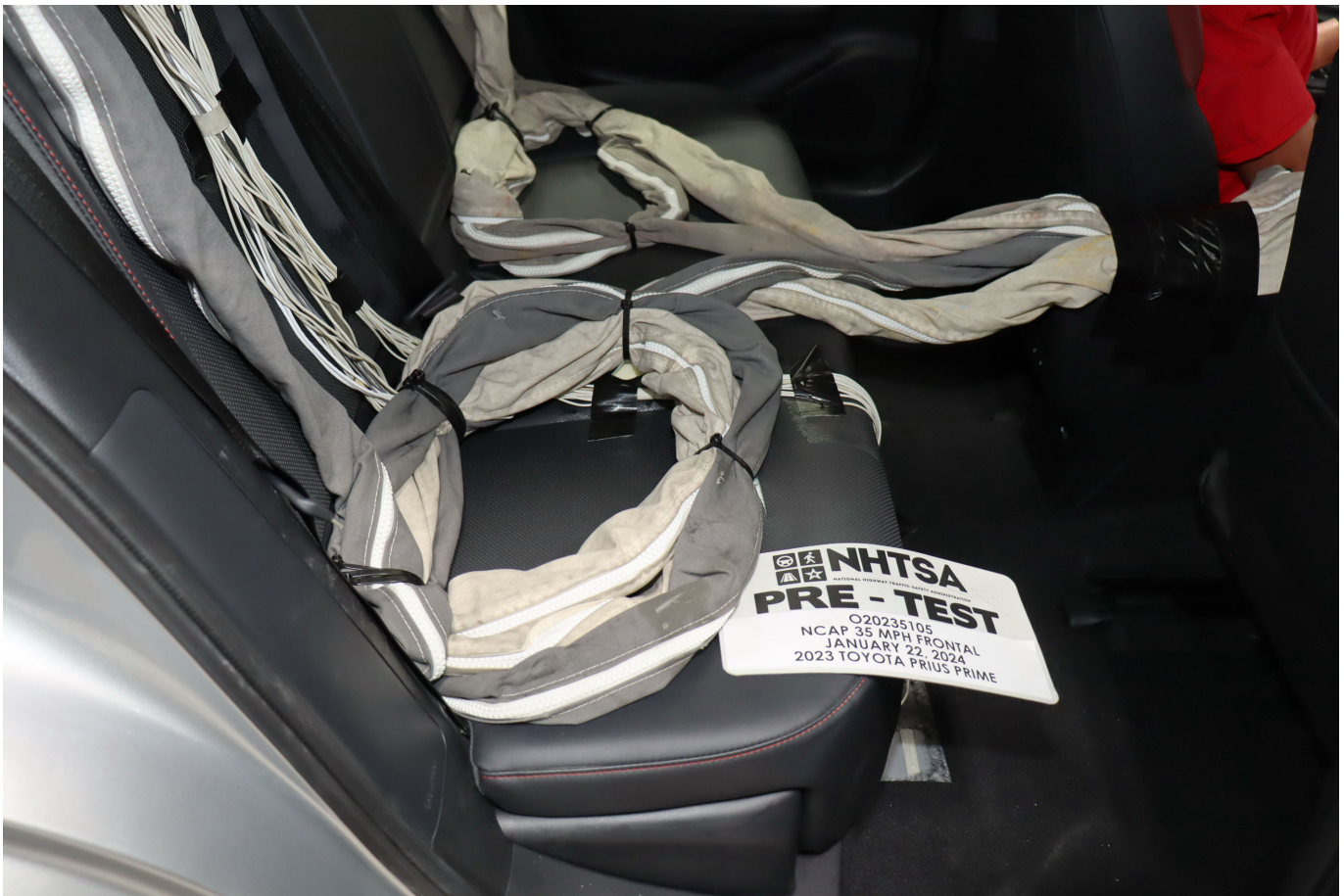
Photo No. 028 - Pre-Test Dummy Cable Routing
