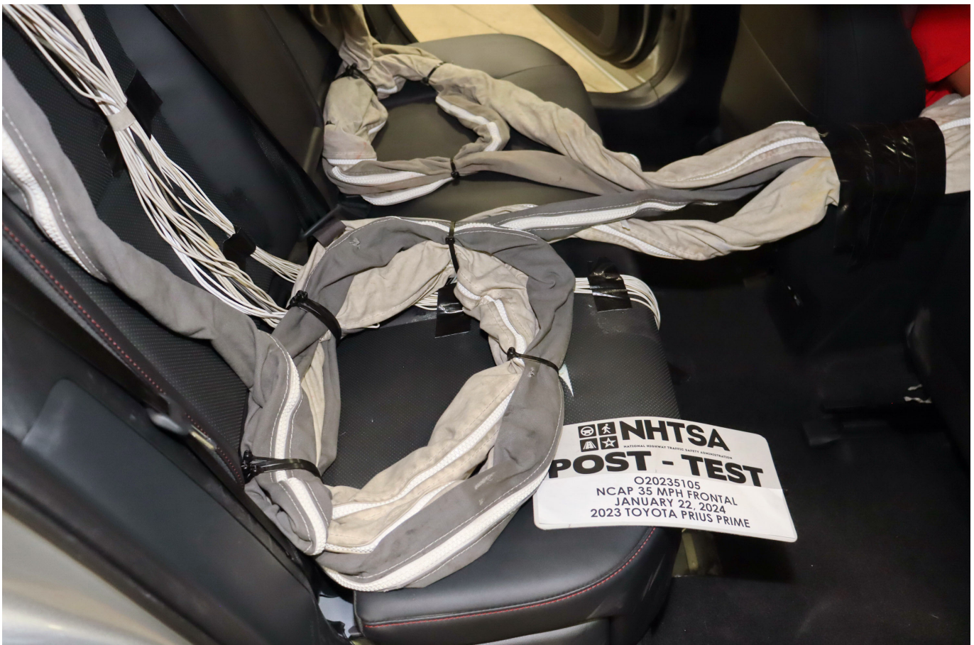
Photo No. 029 - Post-Test Dummy Cable Routing
