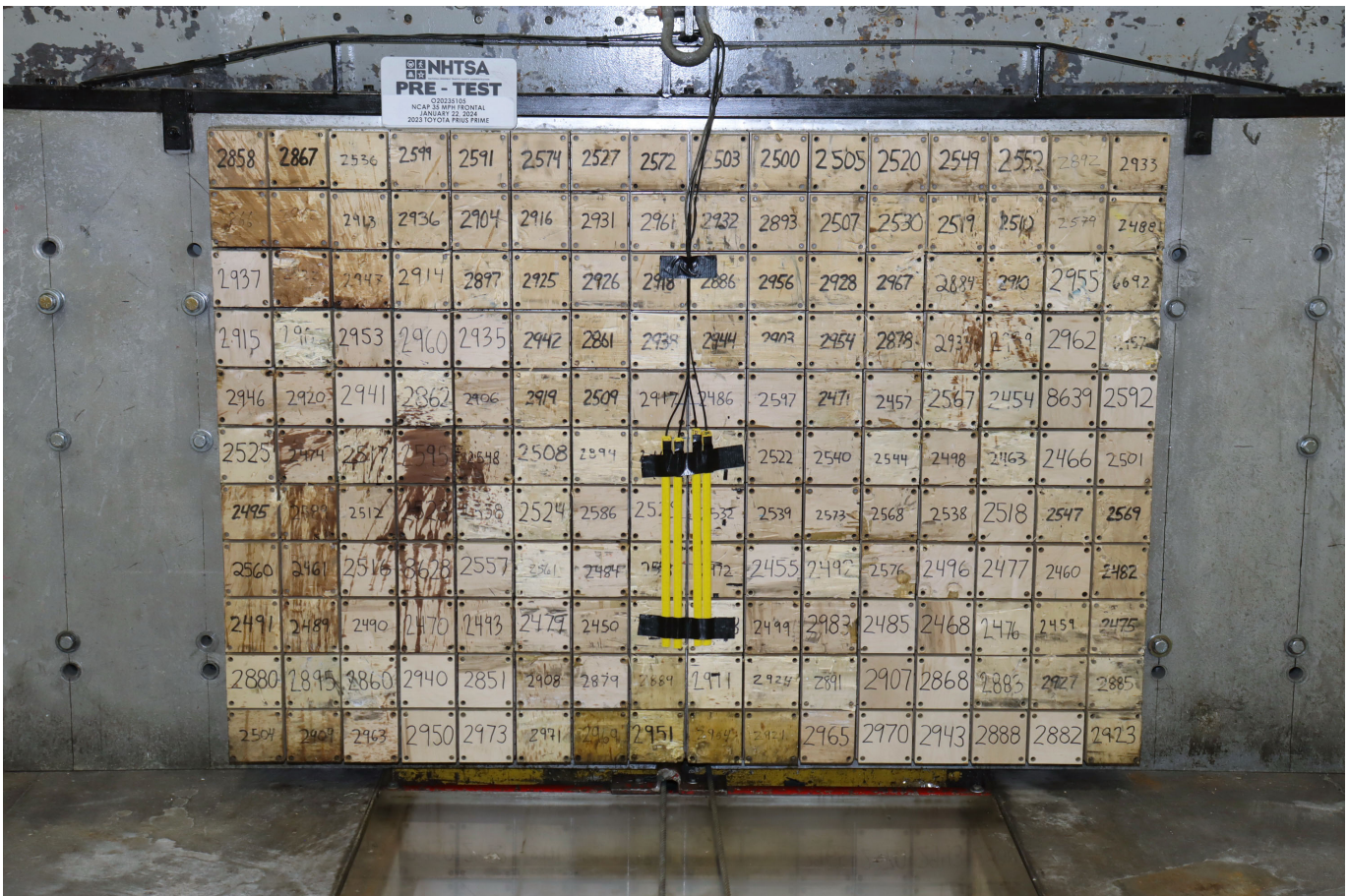
Photo No. 002 - Pre-Test Load Cell Wall
