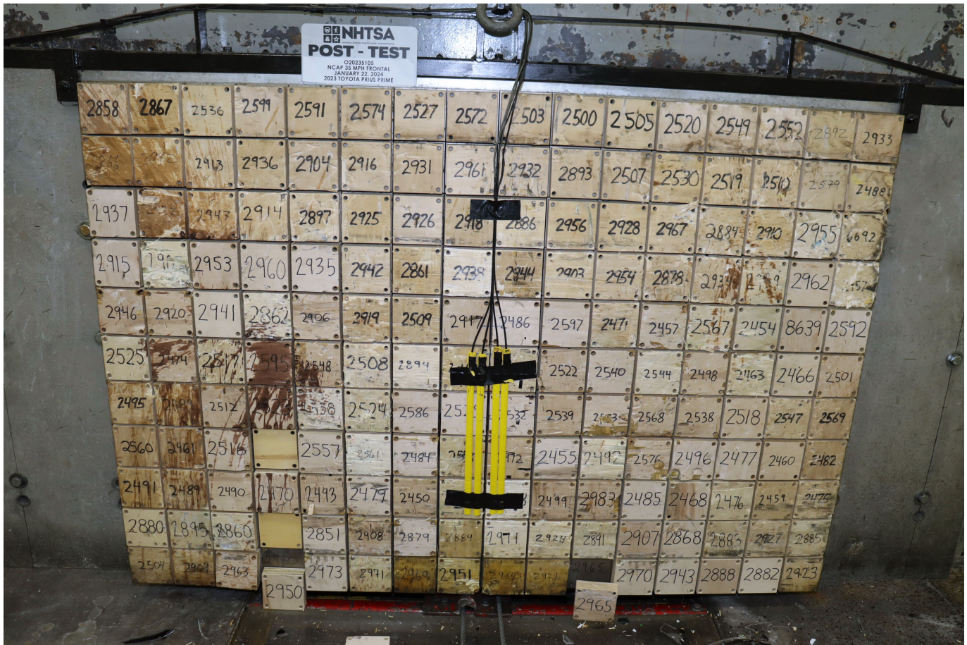
Photo No. 003 - Post-Test Load Cell Wall
