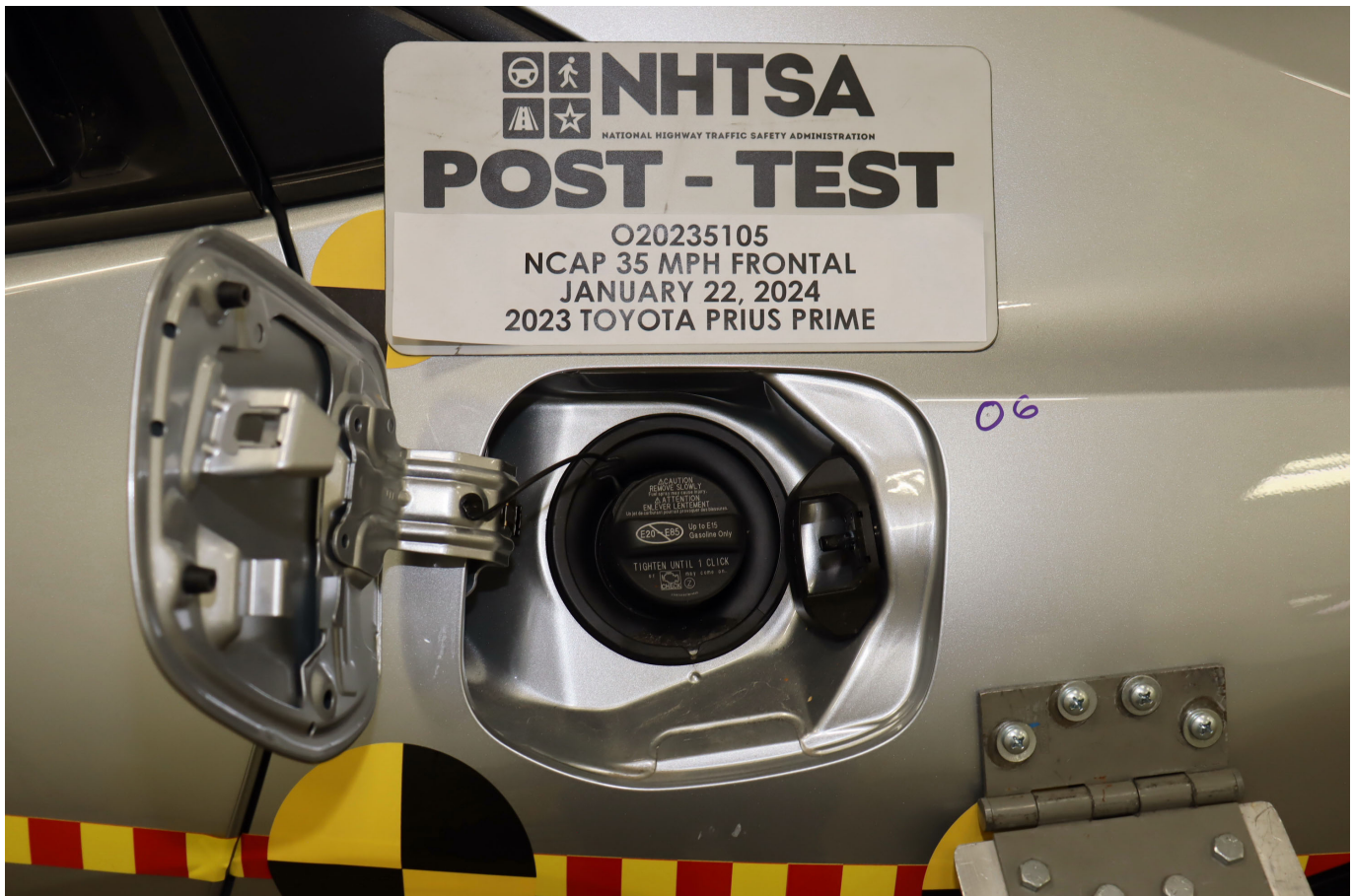
Photo No. 023 - Post-Test Fuel Filler Cap View
