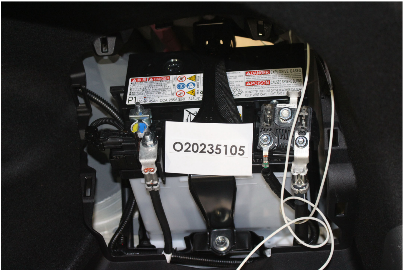
Photo No. 305-01 - Auxiliary Power Module Warning Label
