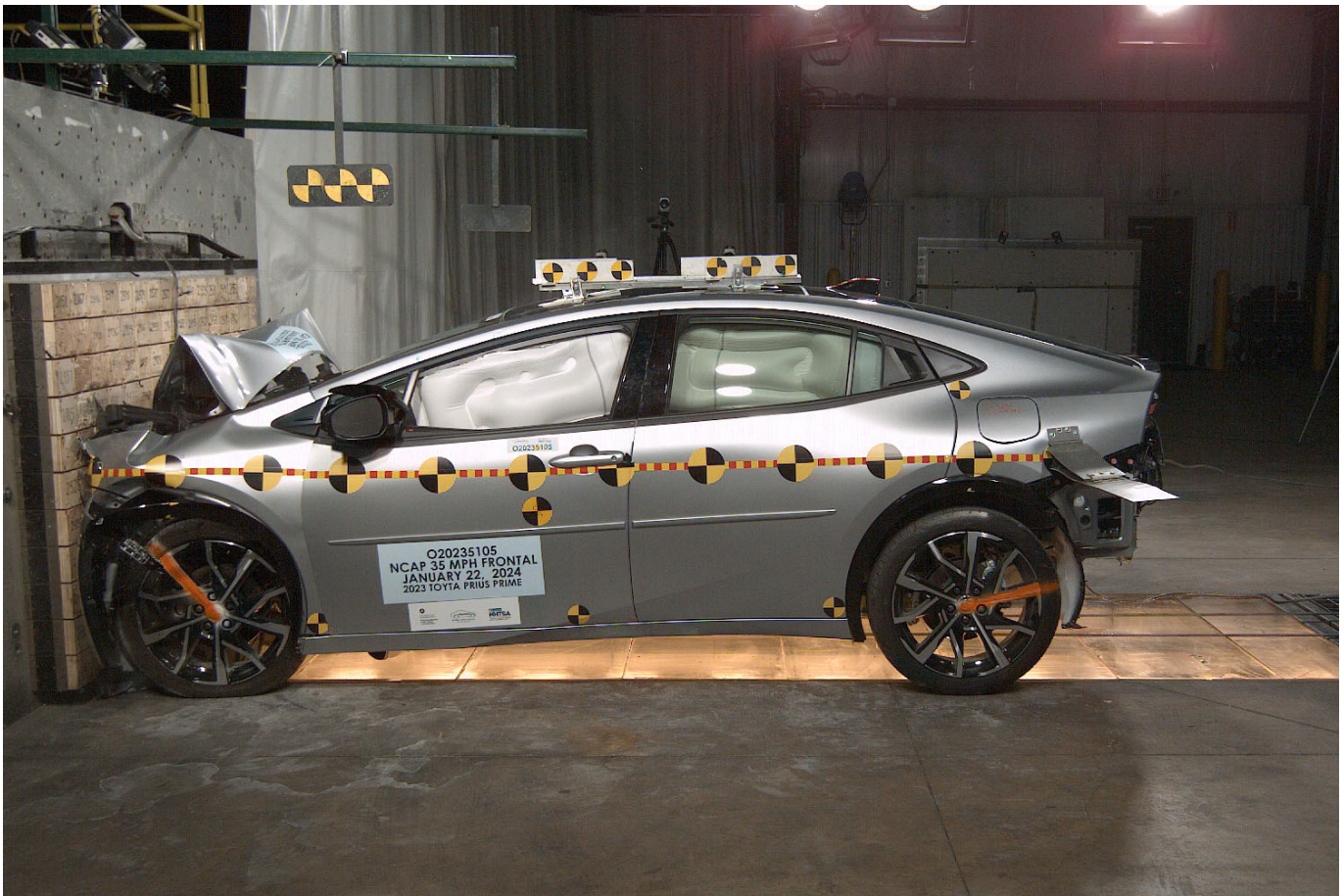
Photo No. 082 - 2023 Toyota Prius Prime XSE Premium 5-Door Hatchback Frontal Impact Event
