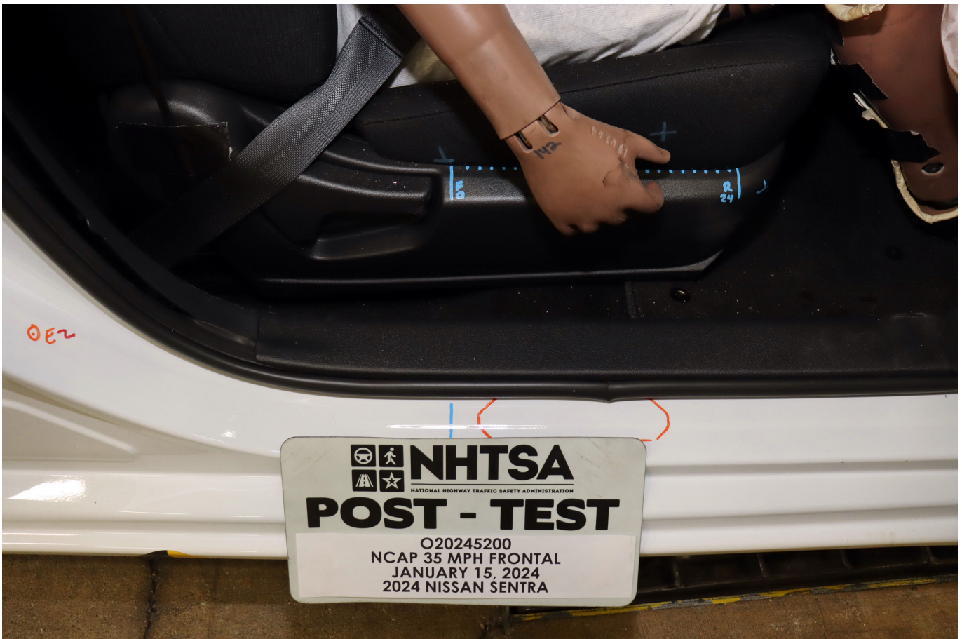
Photo No. 060 - Post-Test Passenger's Seat Fore-Aft Markings
