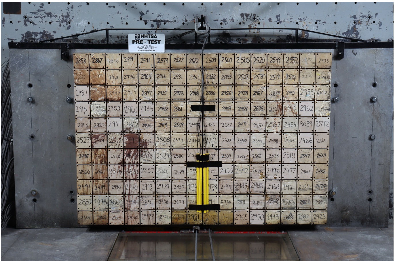
Photo No. 002 - Pre-Test Load Cell Wall
