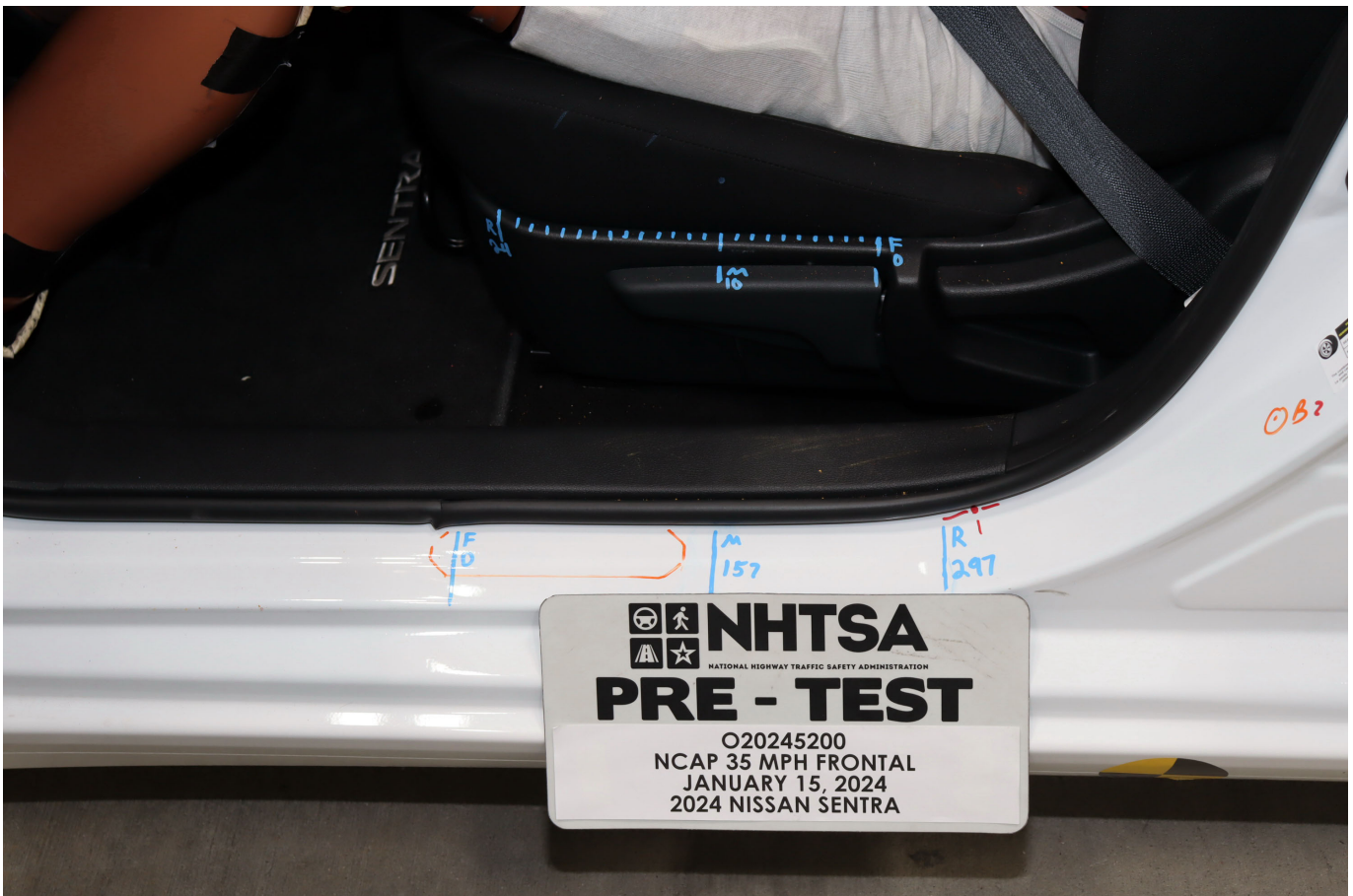
Photo No. 036 - Pre-Test Driver's Seat Fore-Aft Markings
