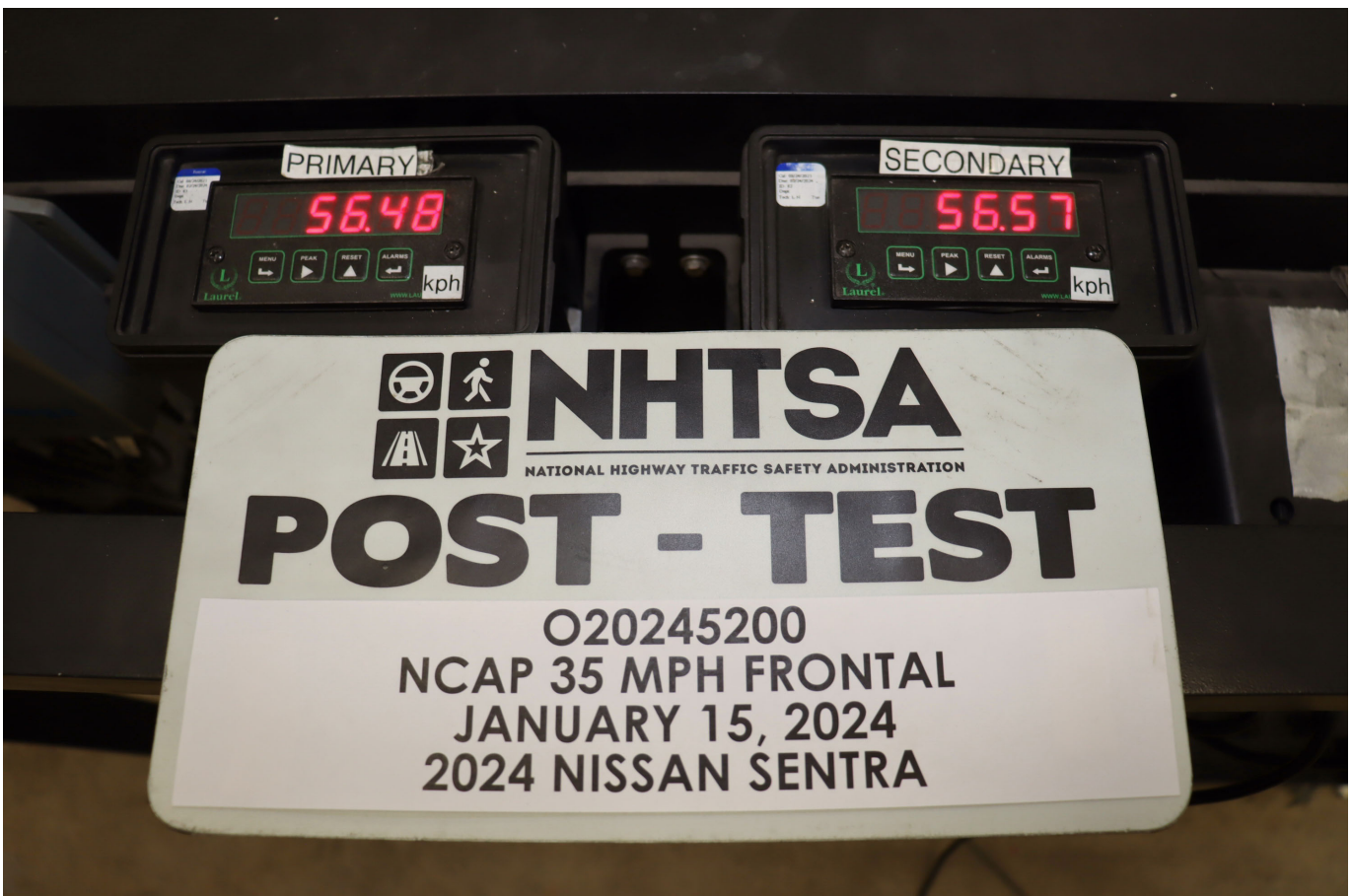
Photo No. 076 - Post-Test Speed Trap Read-Out
