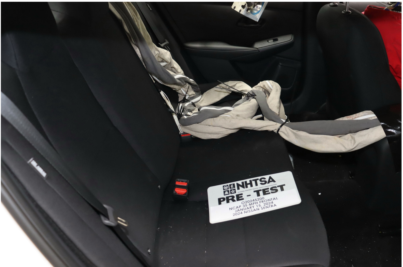
Photo No. 028 - Pre-Test Dummy Cable Routing
