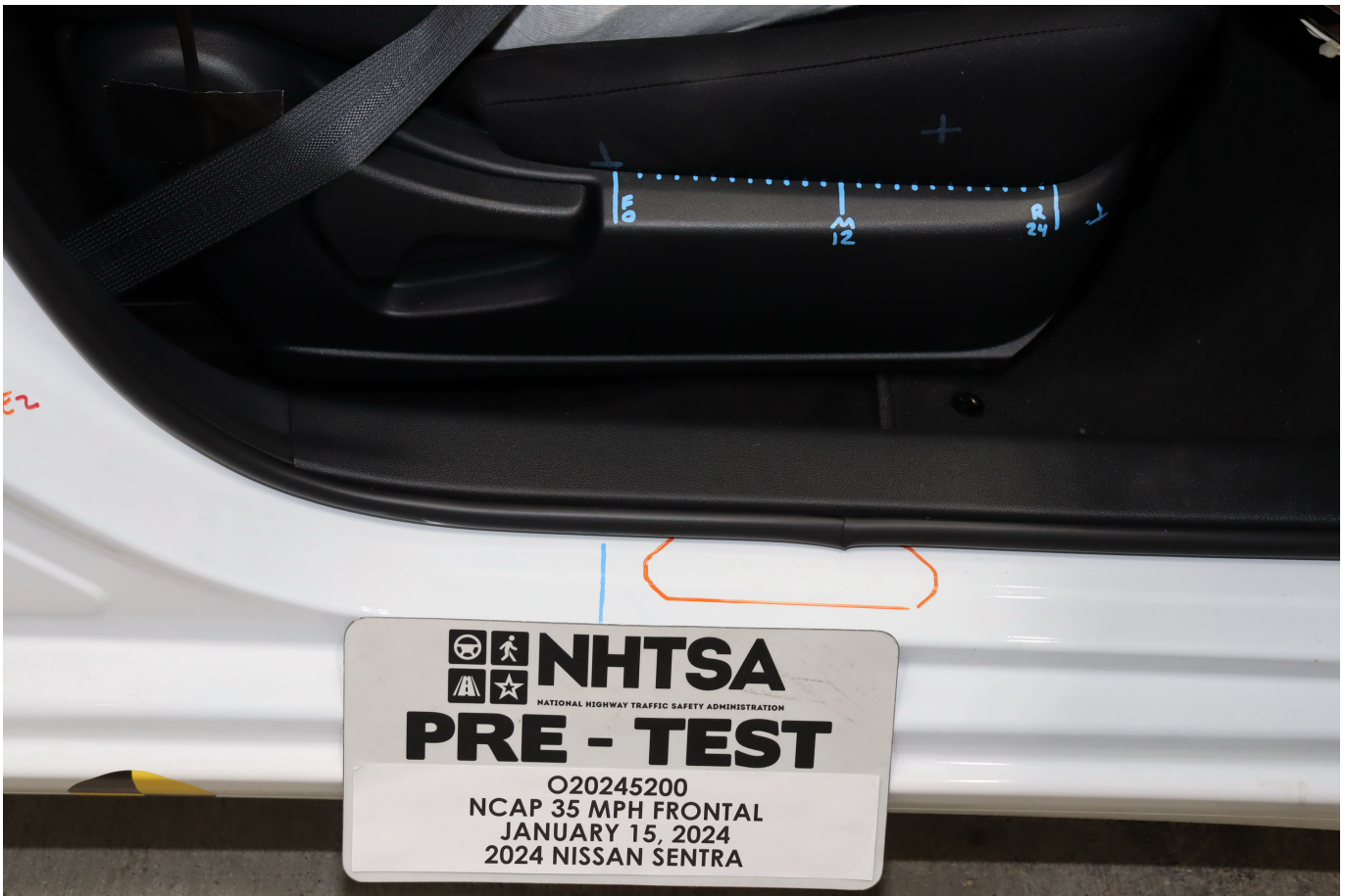
Photo No. 059 - Pre-Test Passenger's Seat Fore-Aft Markings
