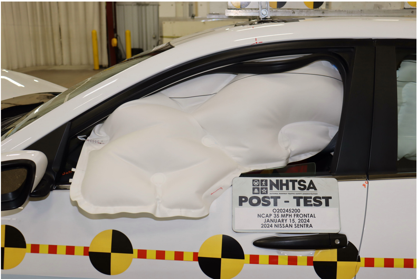
Photo No. 033 - Post-Test Driver Dummy Window View
