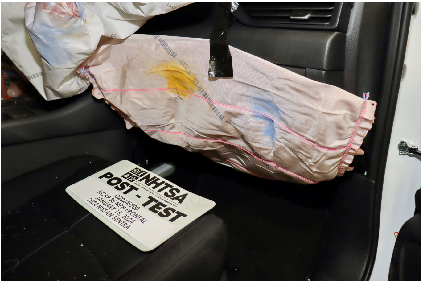
Photo No. 068 - Post-Test Passenger's Side Knee Bolster
