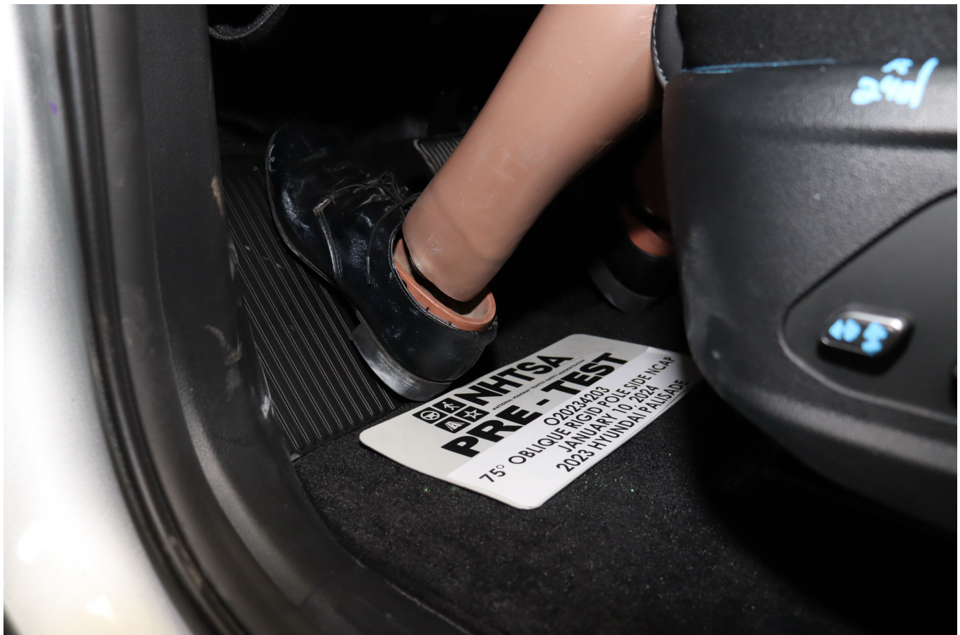
Photo No. 032 - Pre-Test Placement of Dummy's Feet
