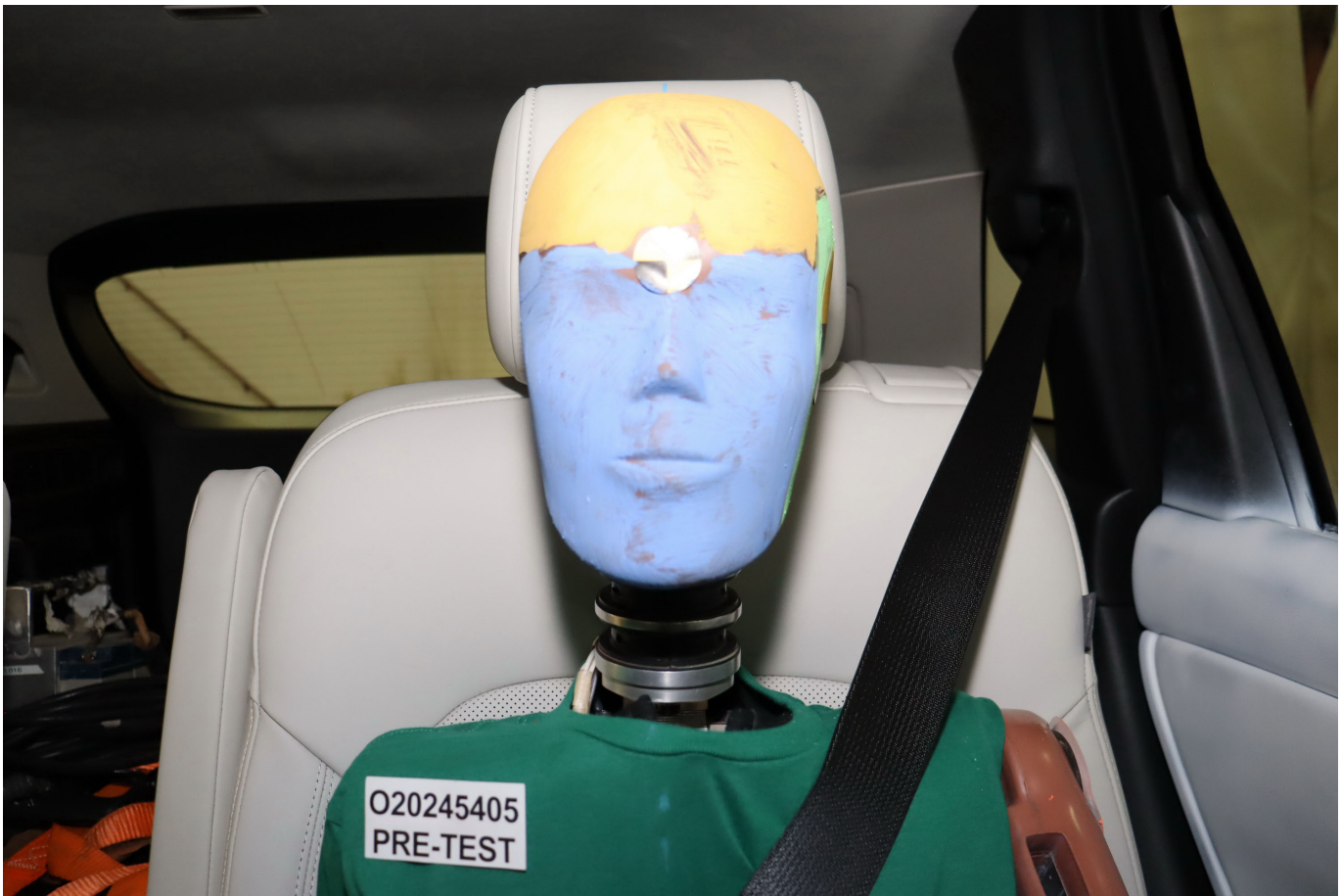
Photo No. 059 - Pre-Test Frontal View of Rear Passenger Dummy Head and Shoulders in Relation to Head Restraint
