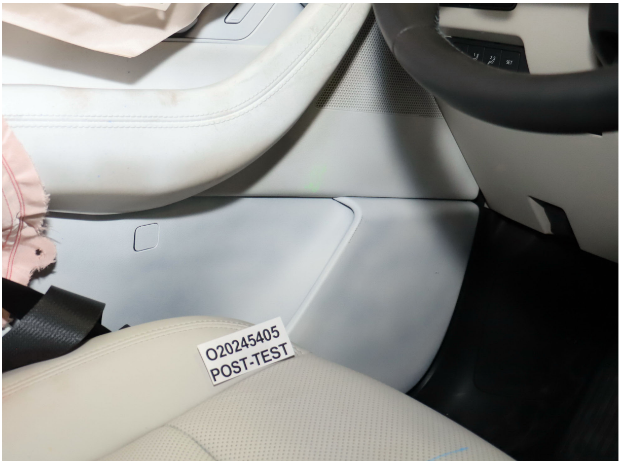
Photo No. 054 - Post-Test Driver Dummy Close-up Knee Contact View
