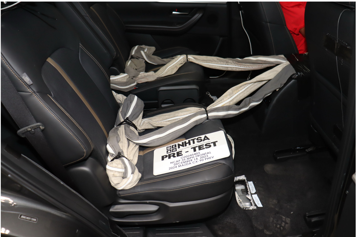
Photo No. 028 - Pre-Test Dummy Cable Routing
