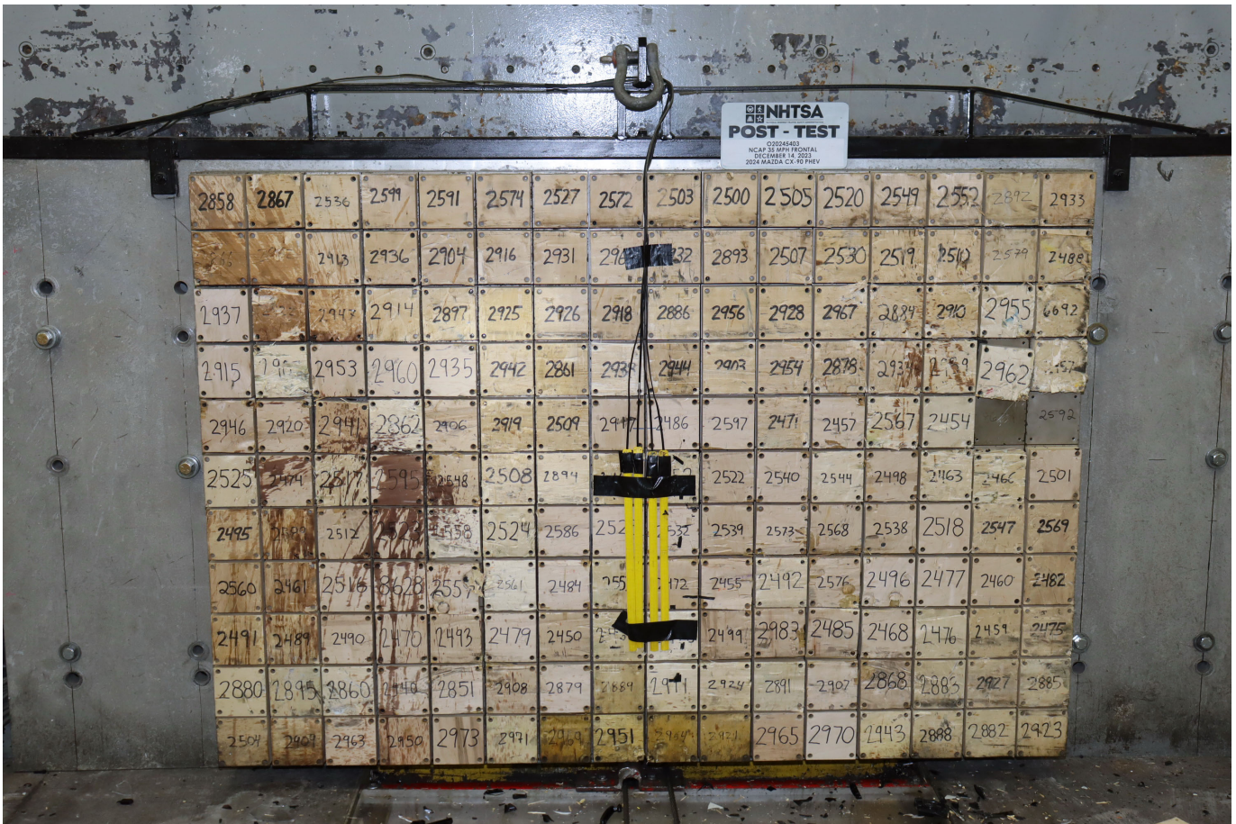
Photo No. 003 - Post-Test Load Cell Wall
