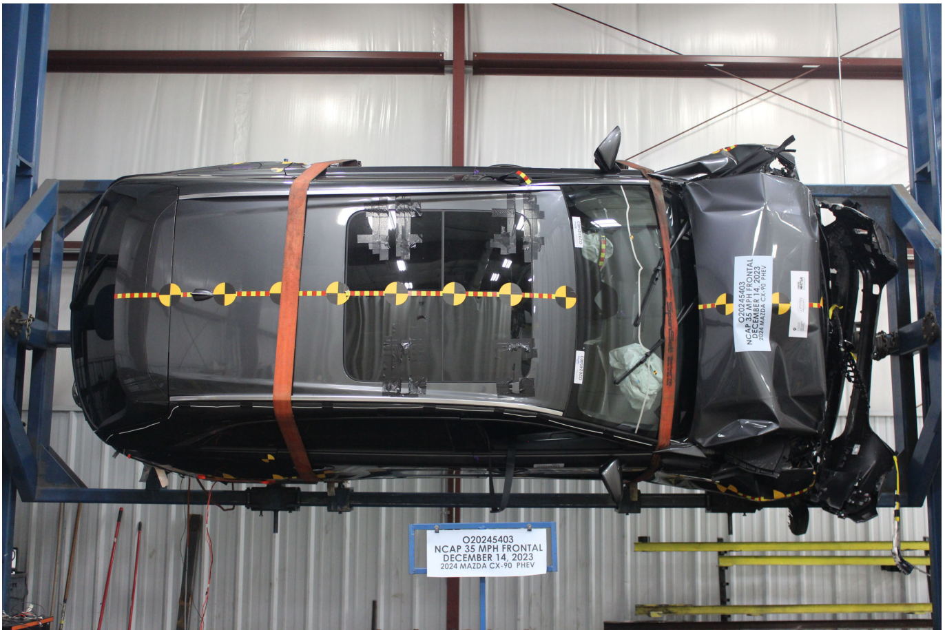
Photo No. 305-30 - FMVSS No. 305 Static Rollover at 270 Degrees
