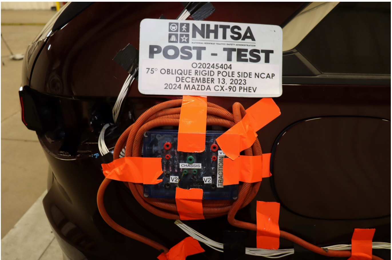
Photo No. 305-25 - Post-Impact View of Installed Test Interface Port
