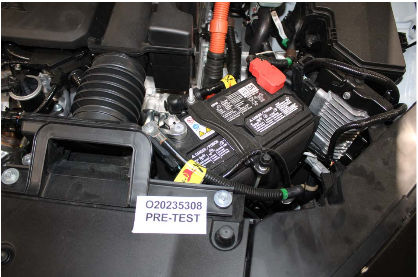
Photo No. 305-04 - First Responder Warning Location
