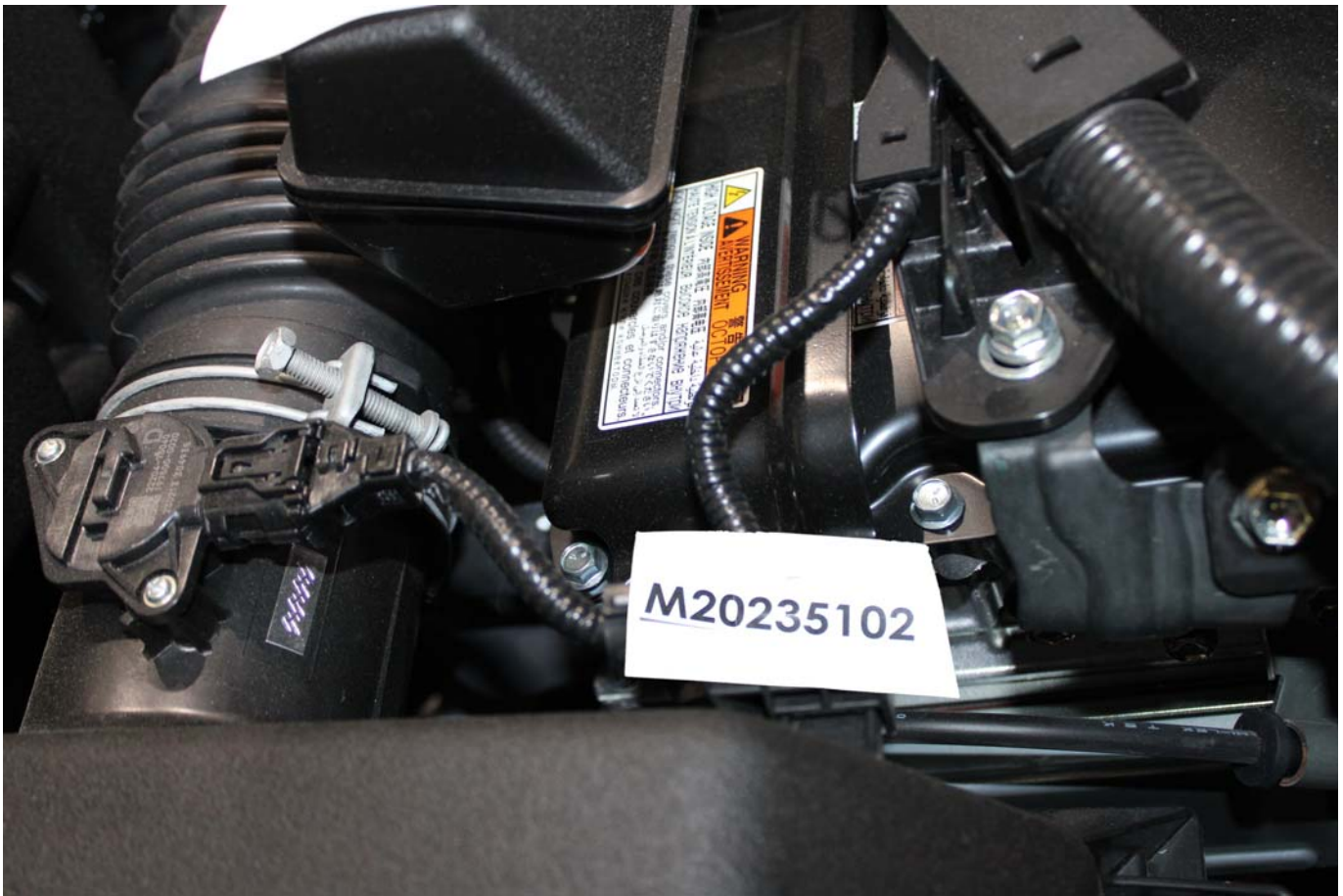
Photo No. 305-02 - Power Inverter Warning Label
