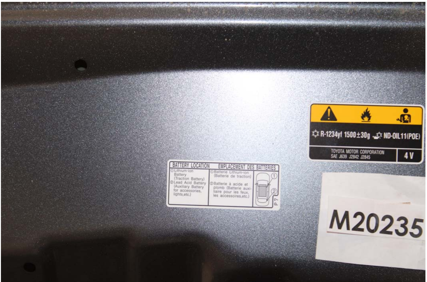
Photo No. 305-03 - First Responder Warning Label
