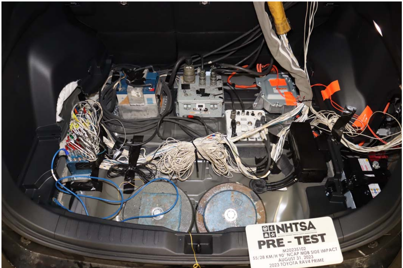
Photo No. 094 - Pre-Test Ballast View
