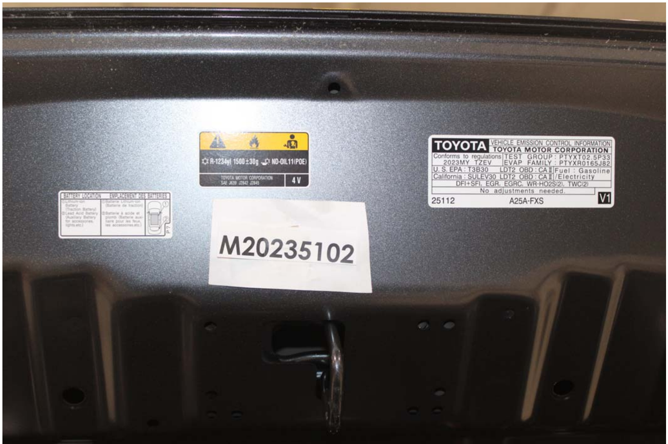
Photo No. 305-04 - First Responder Warning Location
