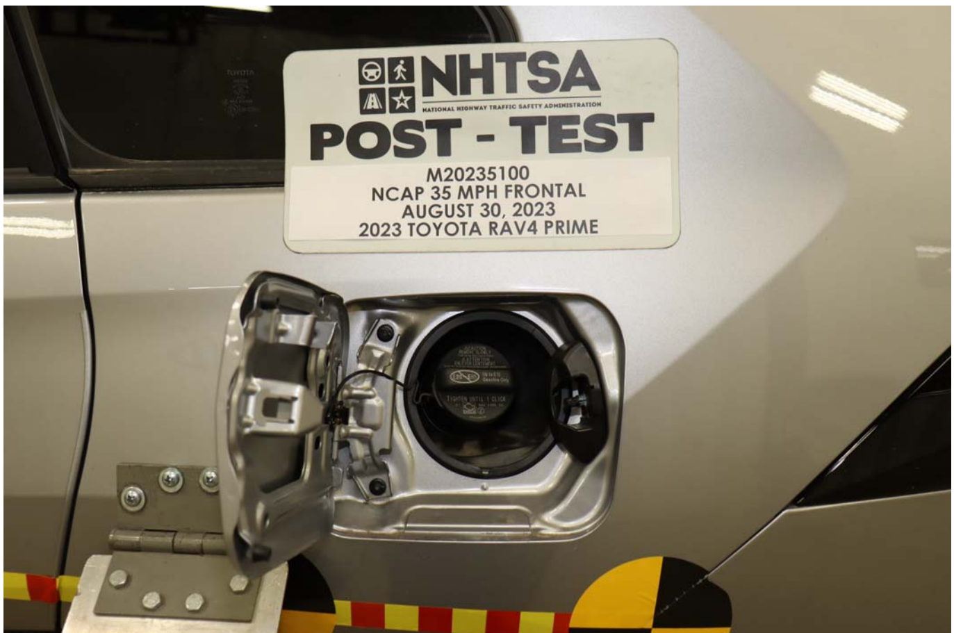
Photo No. 023 - Post-Test Fuel Filler Cap View
