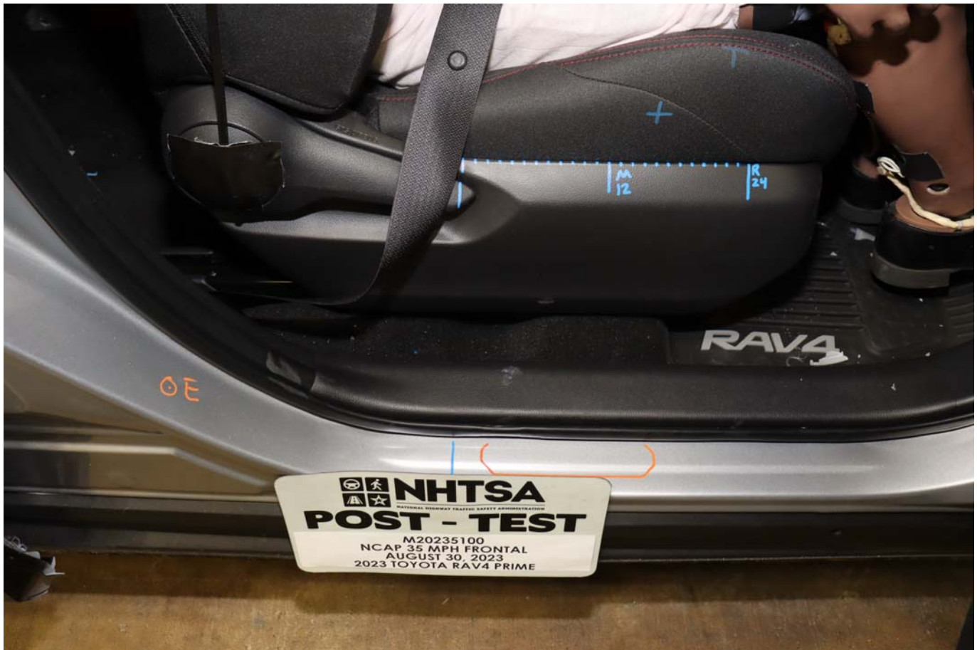
Photo No. 060 - Post-Test Passenger's Seat Fore-Aft Markings
