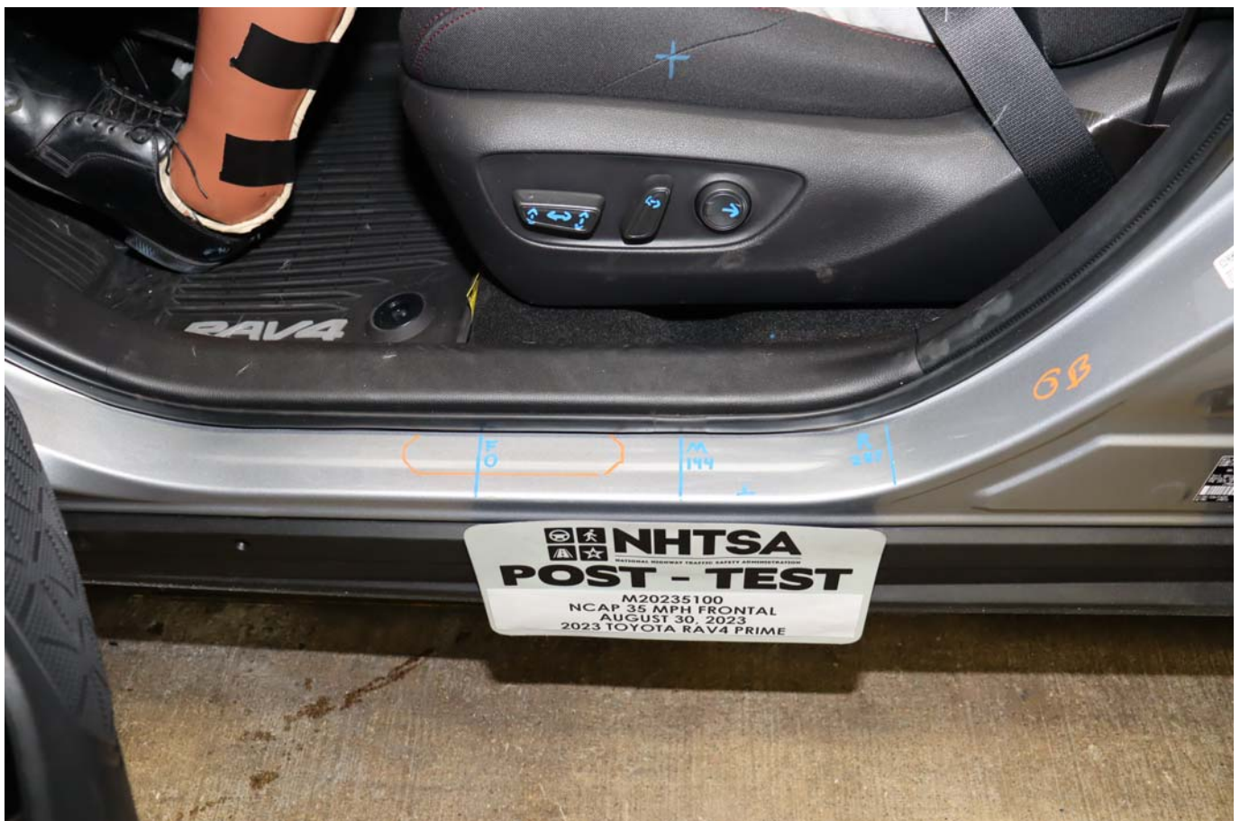
Photo No. 037 - Post-Test Driver's Seat Fore-Aft Markings
