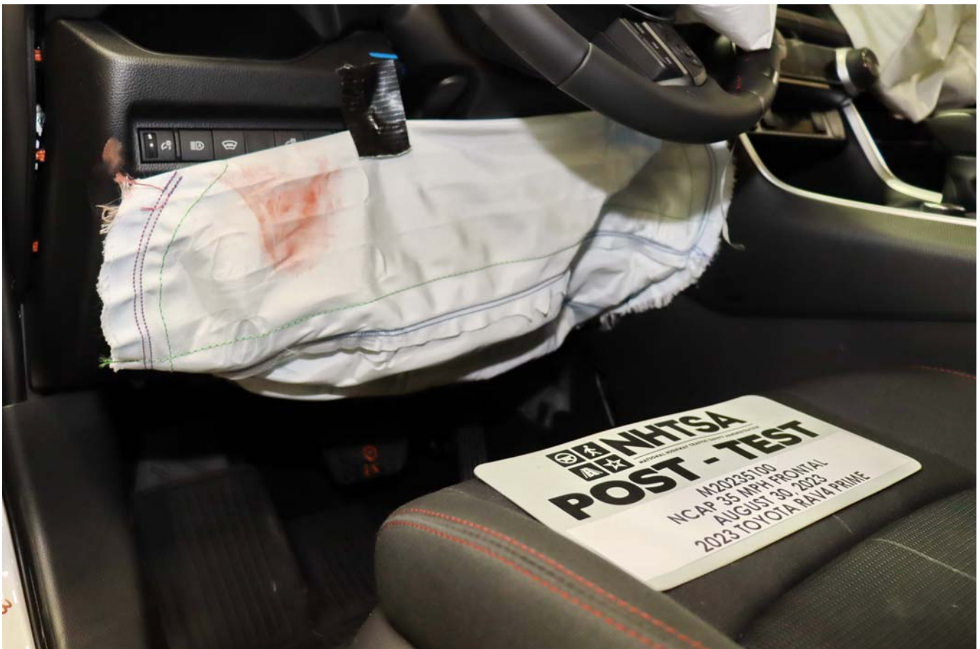
Photo No. 045 - Post-Test Driver's Side Knee Bolster
