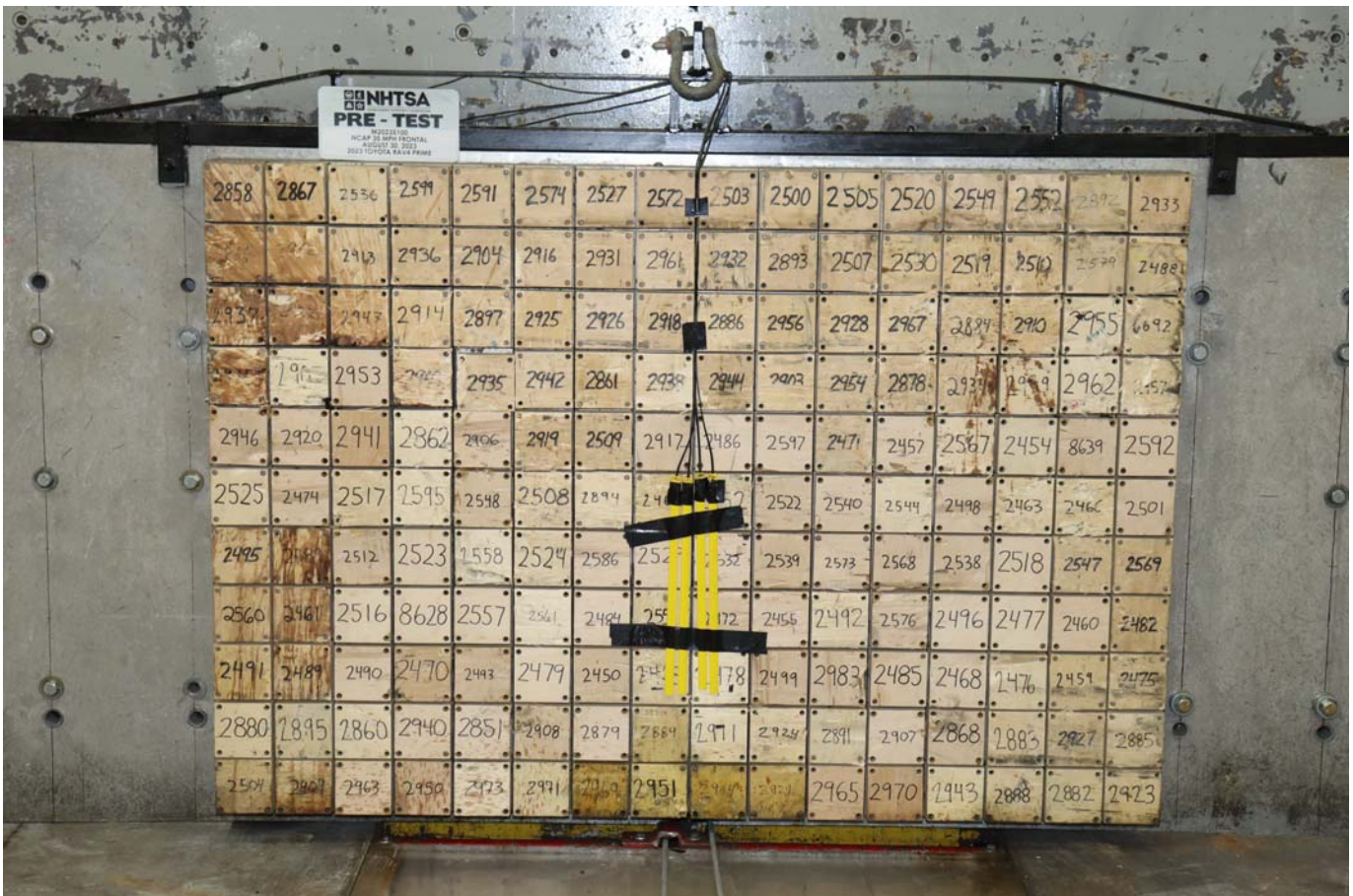
Photo No. 002 - Pre-Test Load Cell Wall
