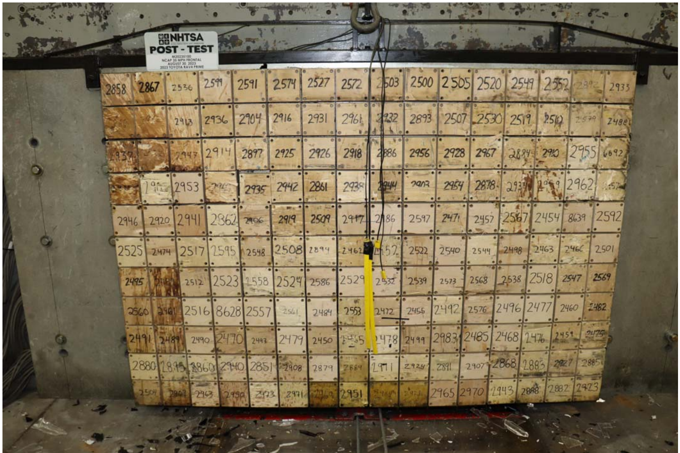
Photo No. 003 - Post-Test Load Cell Wall
