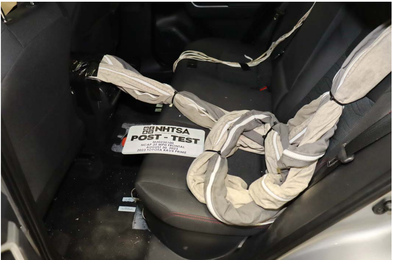
Photo No. 029 - Post-Test Dummy Cable Routing
