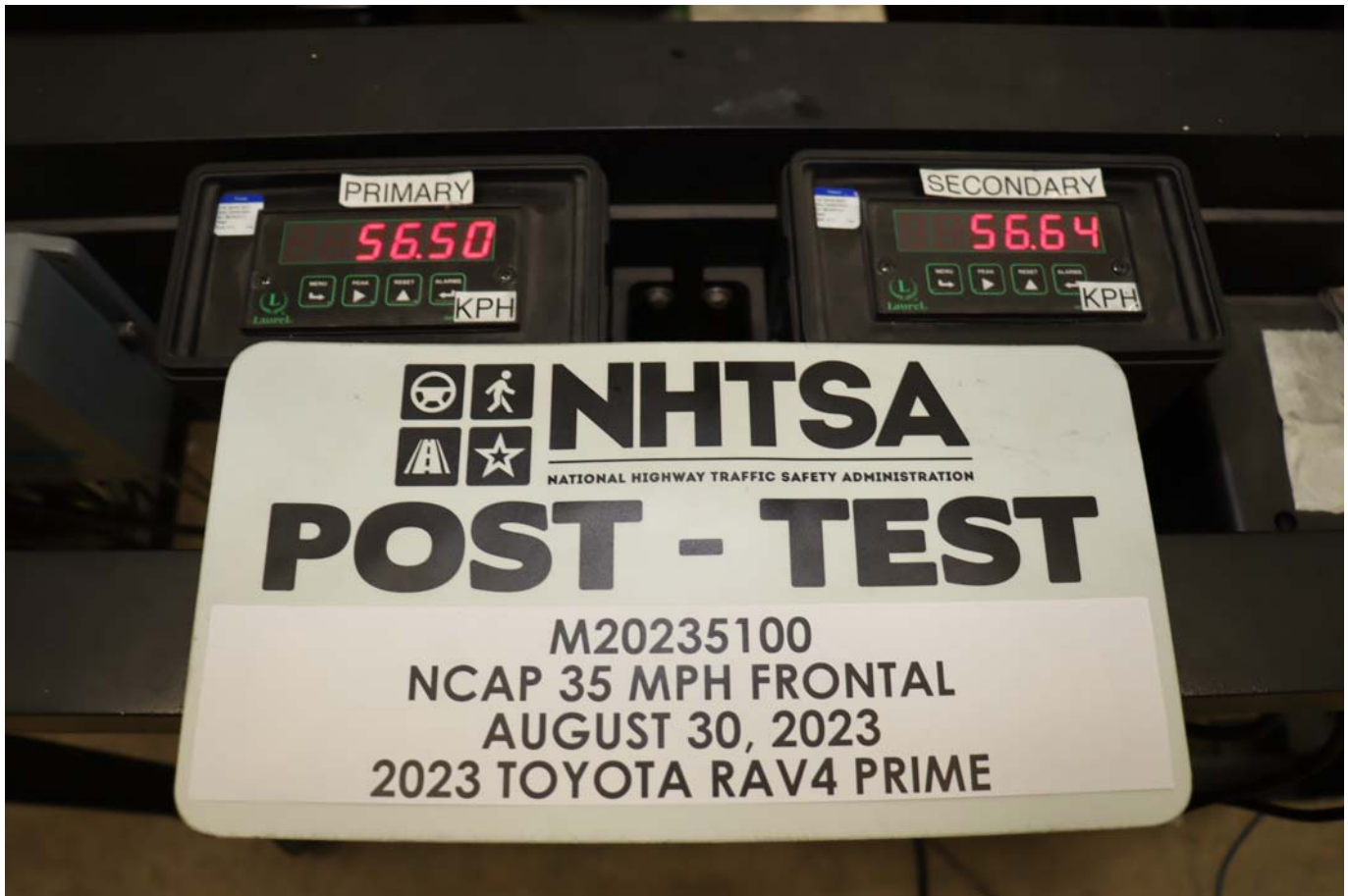
Photo No. 076 - Post-Test Speed Trap Read-Out
