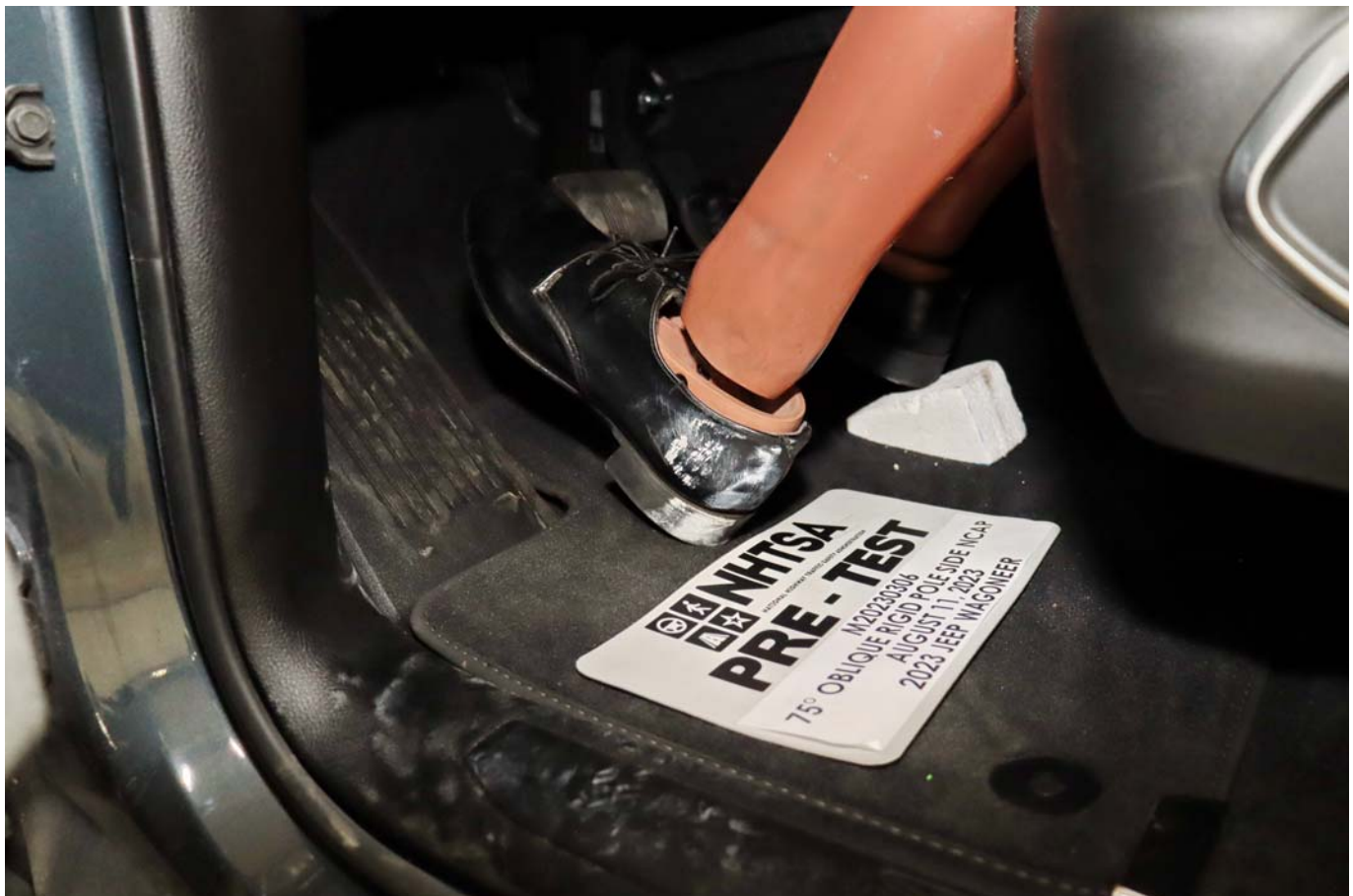
Photo No. 032 - Pre-Test Placement of Dummy's Feet
