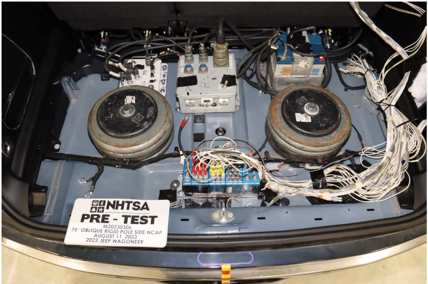
Photo No. 063 - Pre-Test Ballast View
