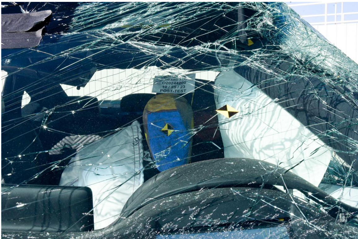
FIGURE 22. Post-Test Front Close-Up View of Dummy
