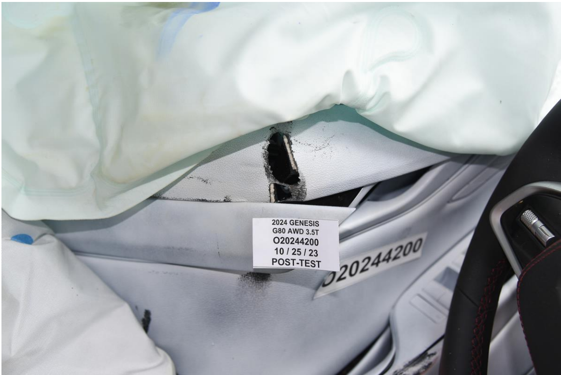
FIGURE 73. Post-Test View of Shattered Vehicle Inner Door Panel
