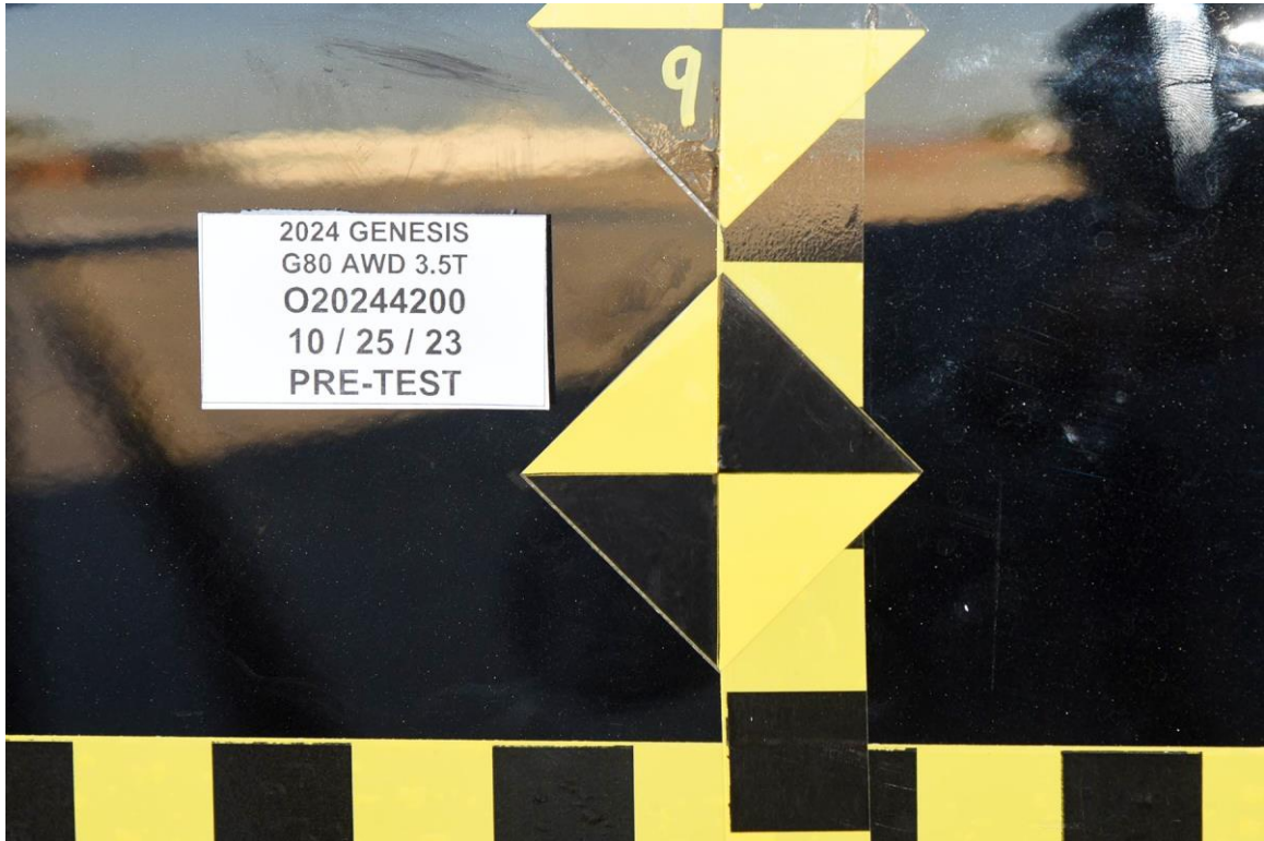
FIGURE 19. Pre-Test Close-Up View of Impact Point Target
