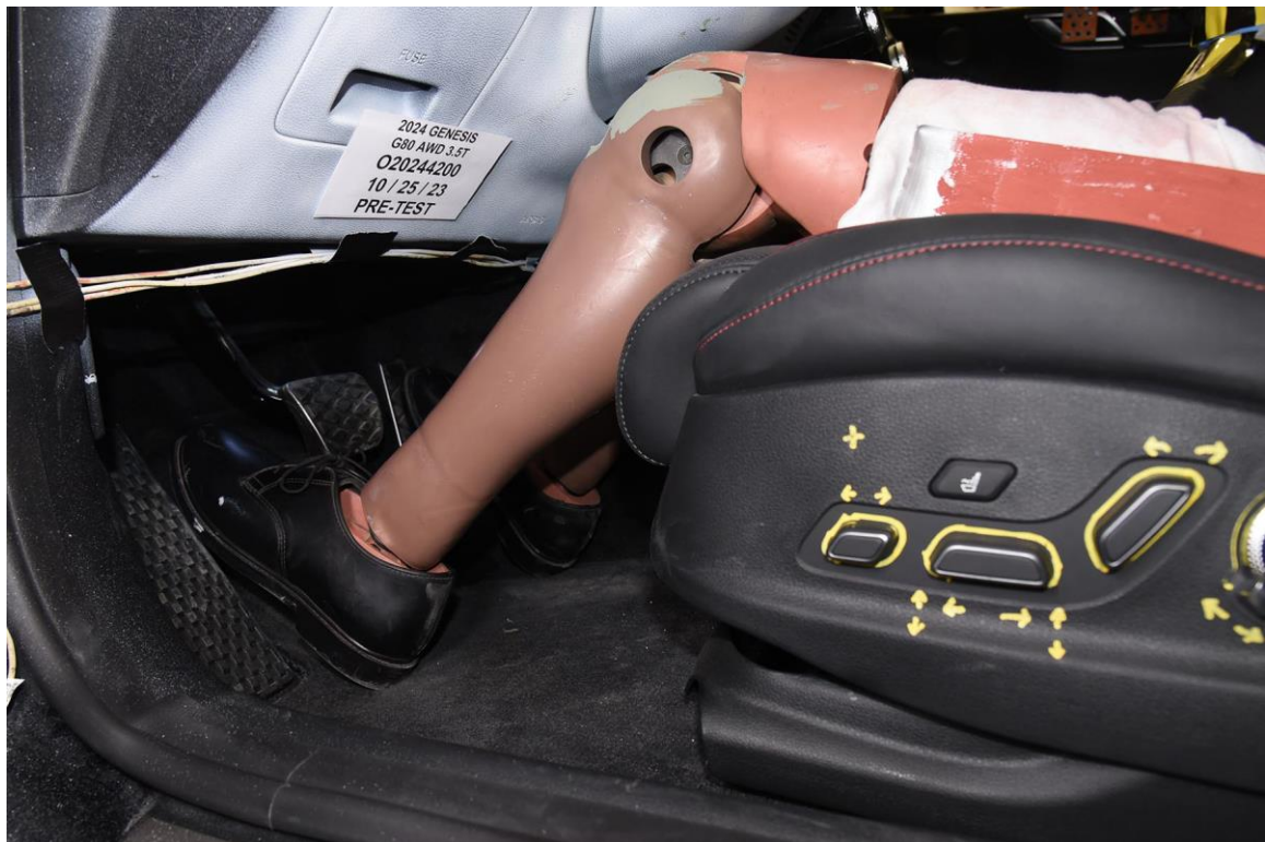
FIGURE 32. Pre-Test Placement of Dummy's Feet
