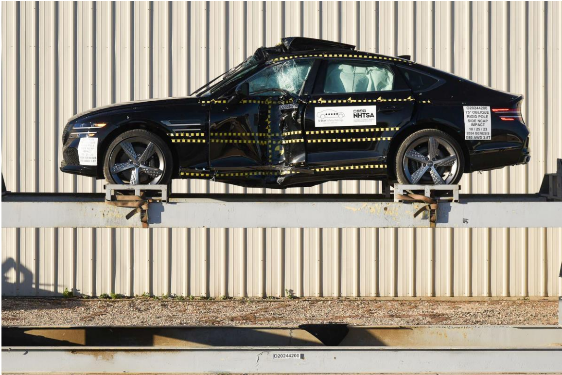
FIGURE 69. FMVSS No. 301 Static Rollover 360 Degrees
