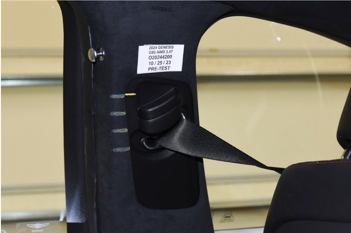
FIGURE 33. Pre-Test View of Belt Anchorage for Dummy
