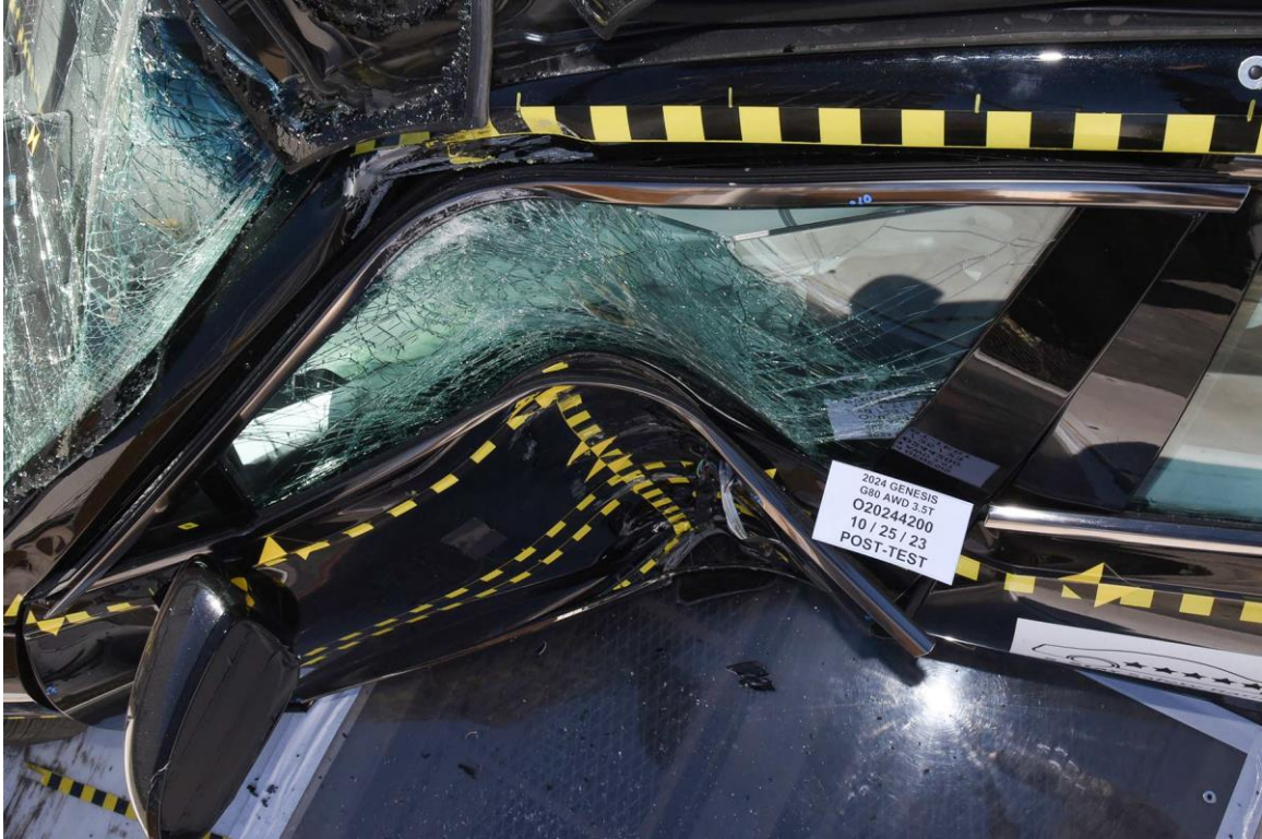
FIGURE 41. Post-Test Dummy and Door Clearance View
