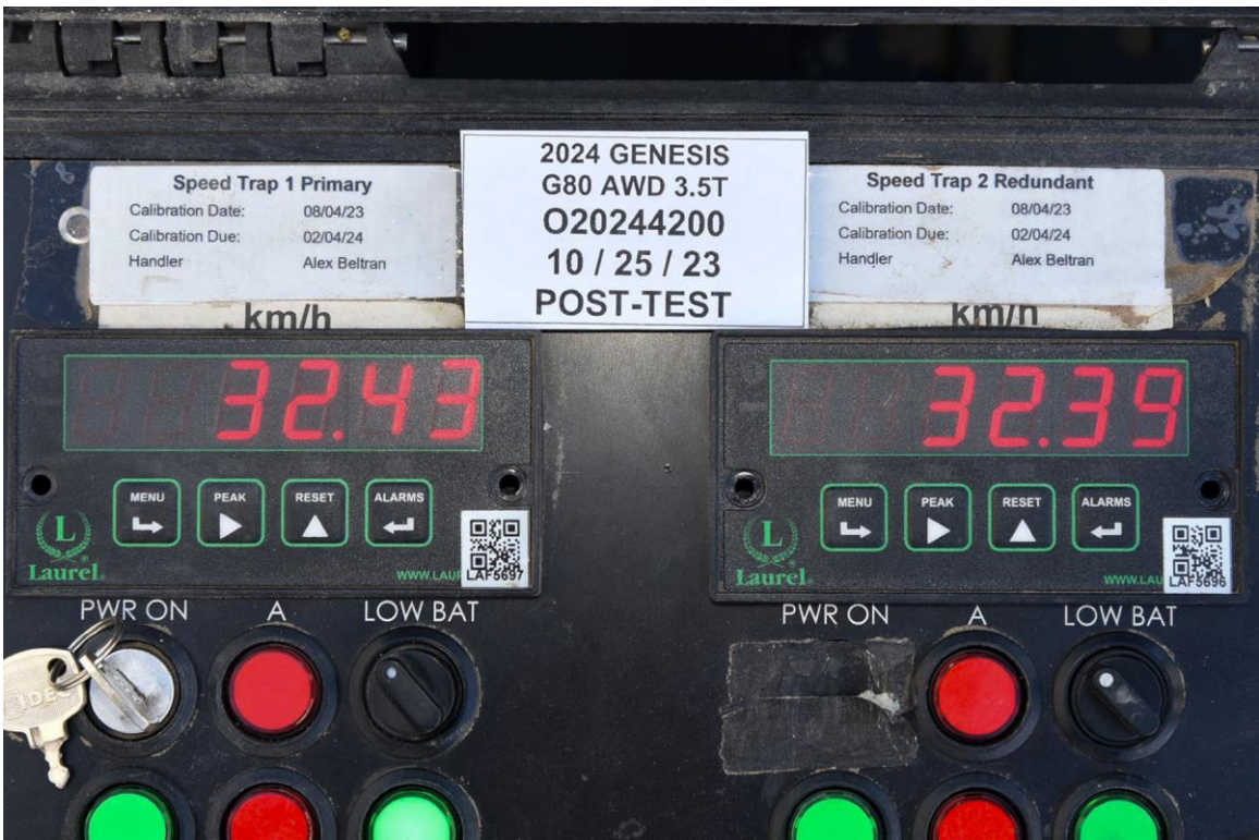
FIGURE 64. Post-Test Primary and Redundant Speed Trap Read-Out
