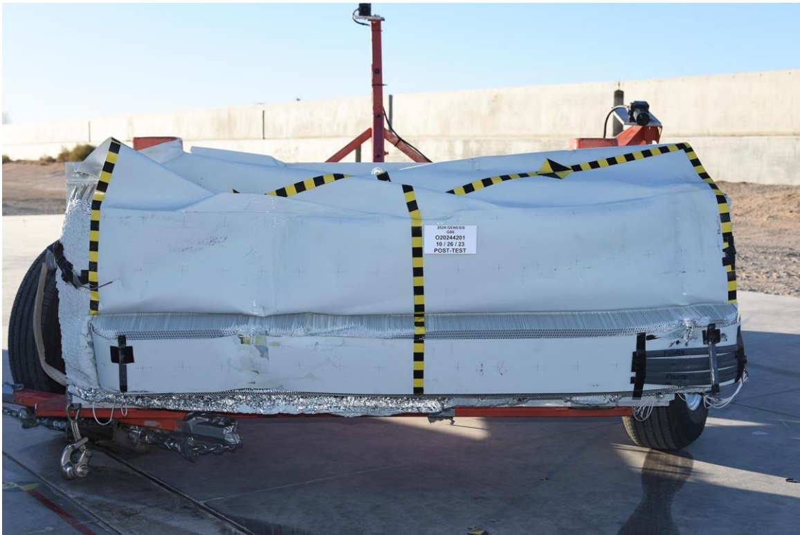
FIGURE 85. Post-Test Front View of MDB Impactor Face
