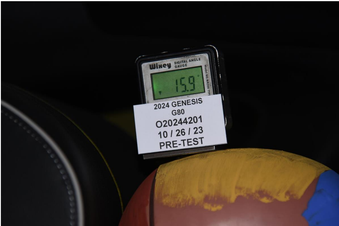
FIGURE 63. Pre-Test View of Rear Passenger Dummy's Head Showing Dummy's Head is Level
