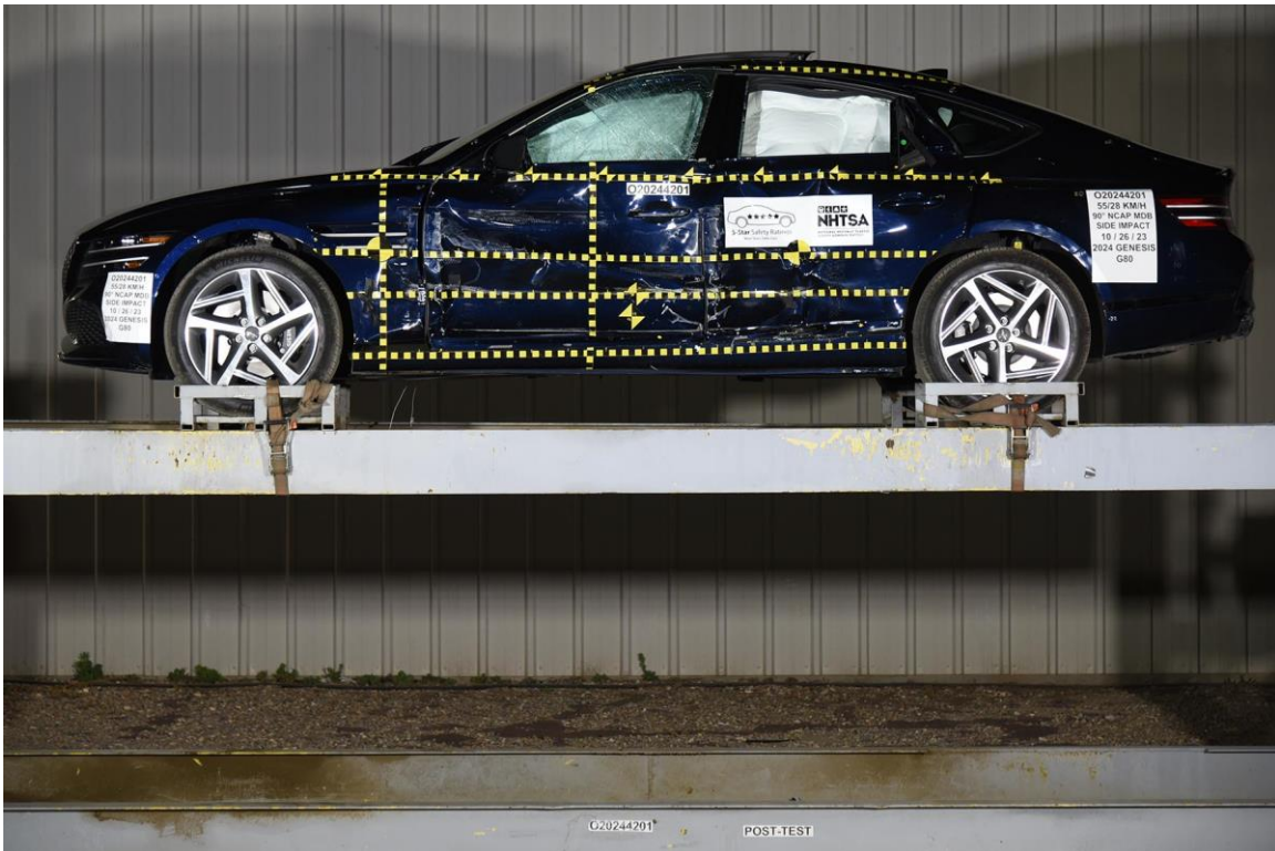
FIGURE 96. FMVSS No. 301 Static Rollover 0 Degrees
