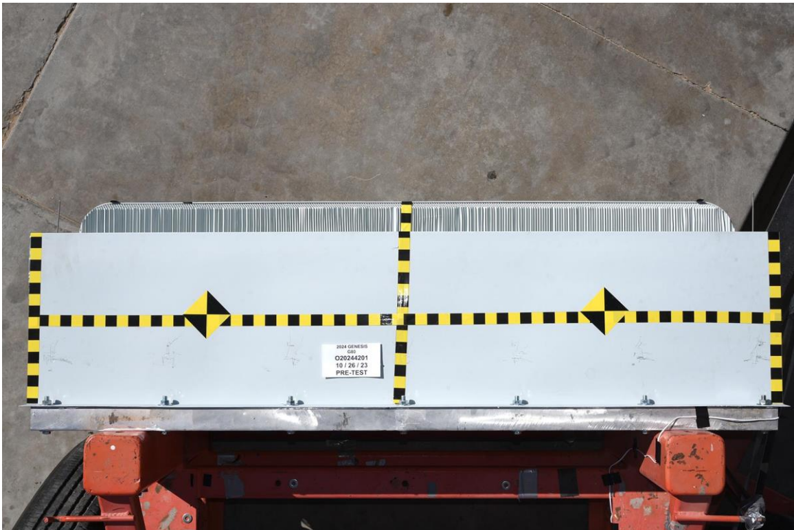
FIGURE 86. Pre-Test Top View of MDB Impactor Face
