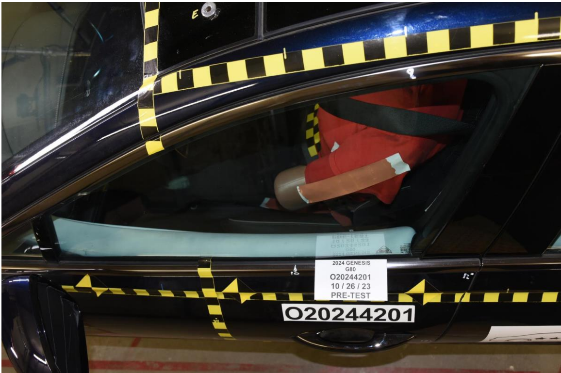
FIGURE 42. Pre-Test Driver Dummy and Door Clearance View
