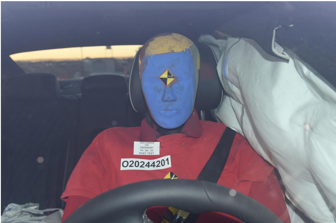
FIGURE 26. Post-Test Front Close-Up View of Driver Dummy
