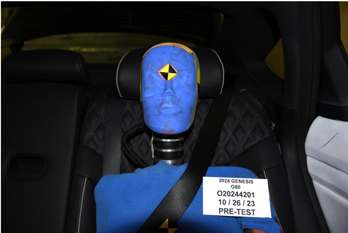
FIGURE 59. Pre-Test Frontal View of Rear Passenger Dummy Head and Shoulders in Relation to Head Restraint
