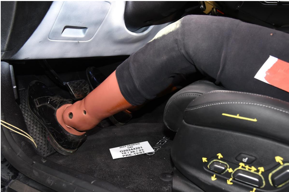
FIGURE 34. Pre-Test Placement of Driver Dummy's Feet
