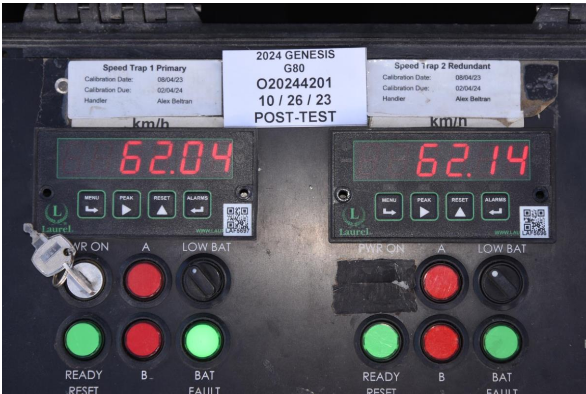
FIGURE 95. Post-Test Primary and Redundant Speed Trap Read-Out
