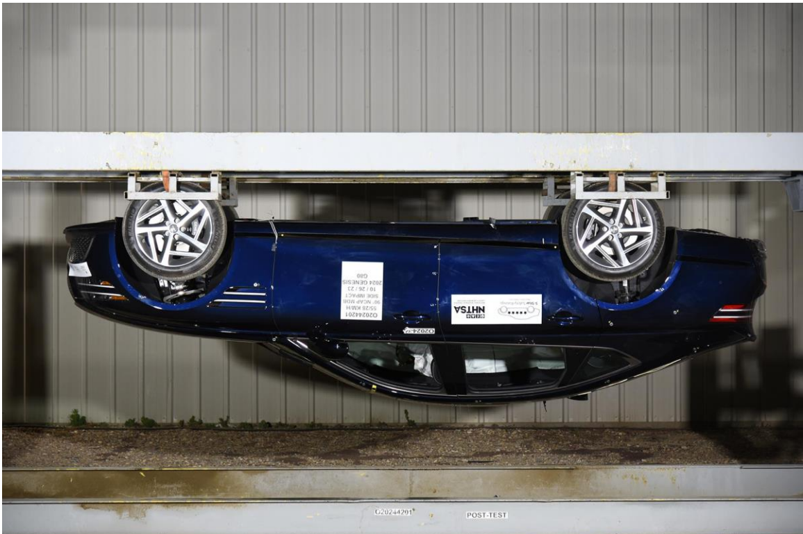
FIGURE 98. FMVSS No. 301 Static Rollover 180 Degrees
