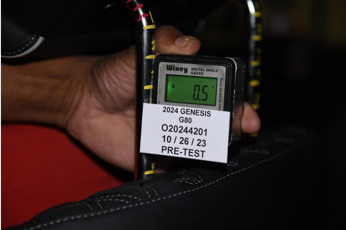
FIGURE 41. Pre-Test Close-Up View of Driver Seat Back or Head Restraint
