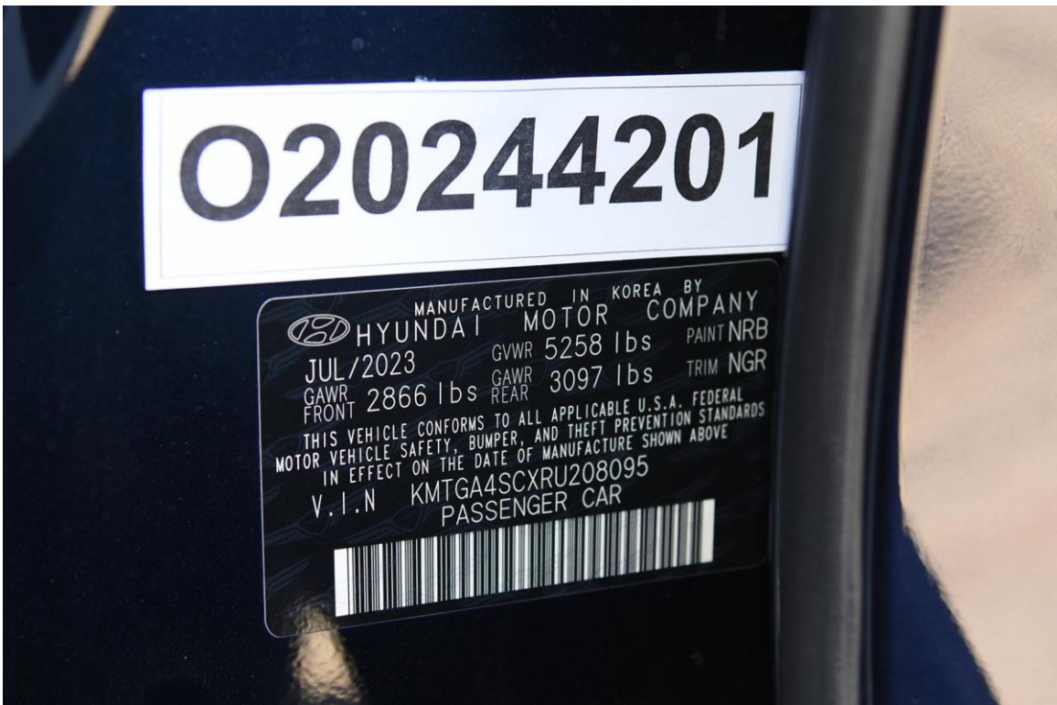
FIGURE 92. Close-Up View of Vehicle's Certification Label
