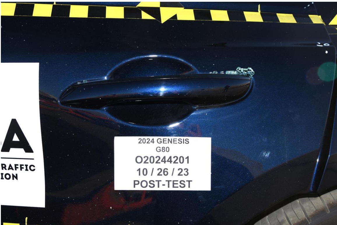
FIGURE 24. Post-Test Left Rear Door Latch Close-Up
