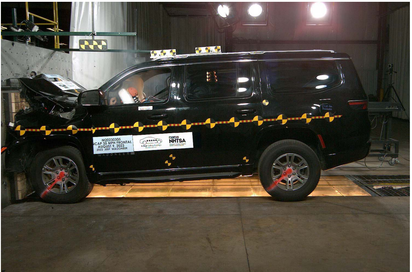
Photo No. 082 - 2023 Jeep Wagoneer 4x4 5-Door SUV Frontal Impact Event
