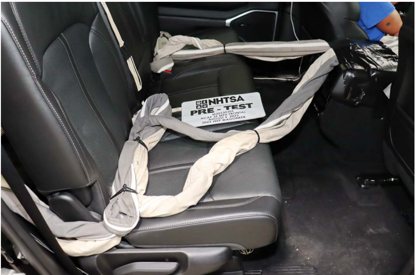
Photo No. 028 - Pre-Test Dummy Cable Routing
