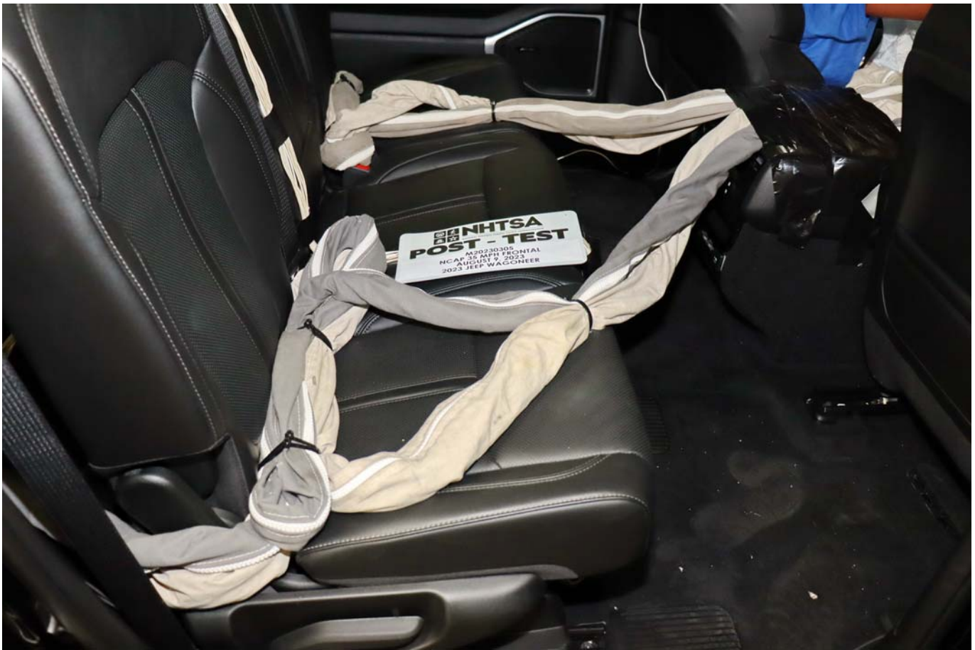
Photo No. 029 - Post-Test Dummy Cable Routing
