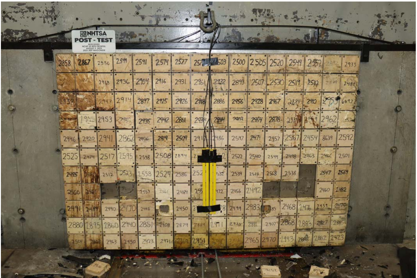
Photo No. 003 - Post-Test Load Cell Wall
