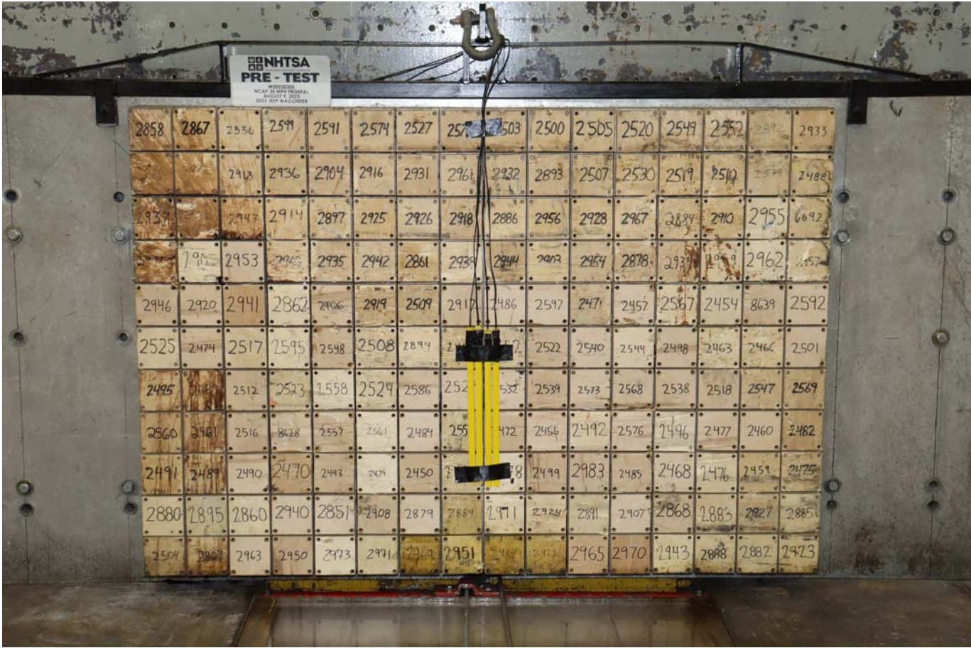
Photo No. 002 - Pre-Test Load Cell Wall
