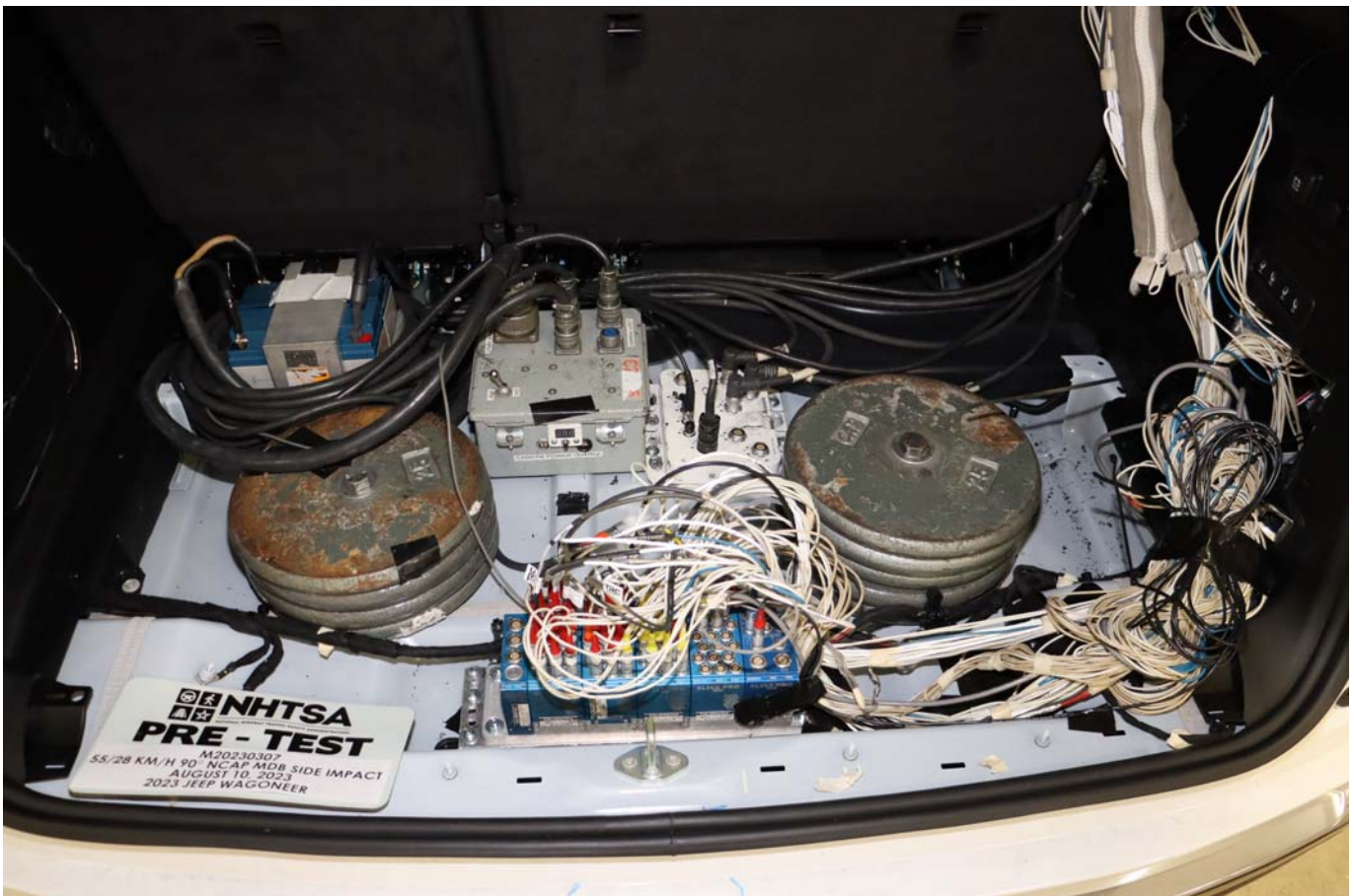
Photo No. 094 - Pre-Test Ballast View
