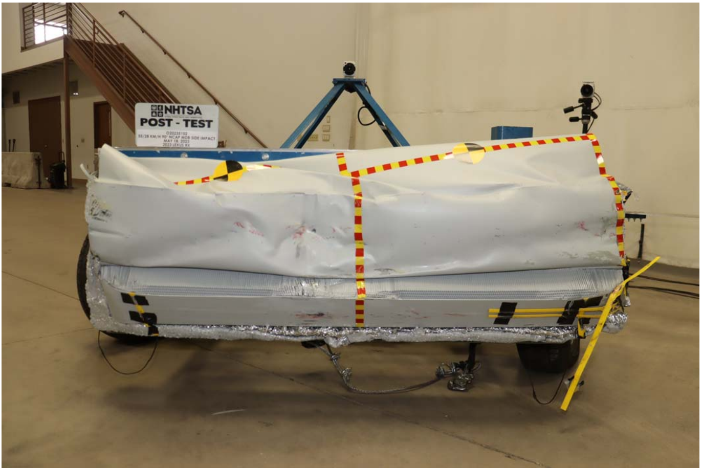
Photo No. 085 - Post-Test Front View of MDB Impactor Face
