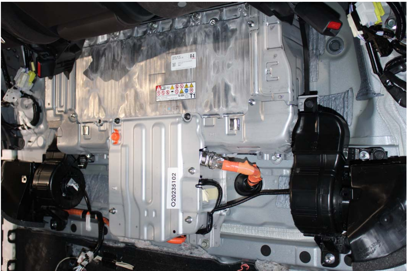
Photo No. 305-09 - Pre-Impact View of Propulsion Battery
