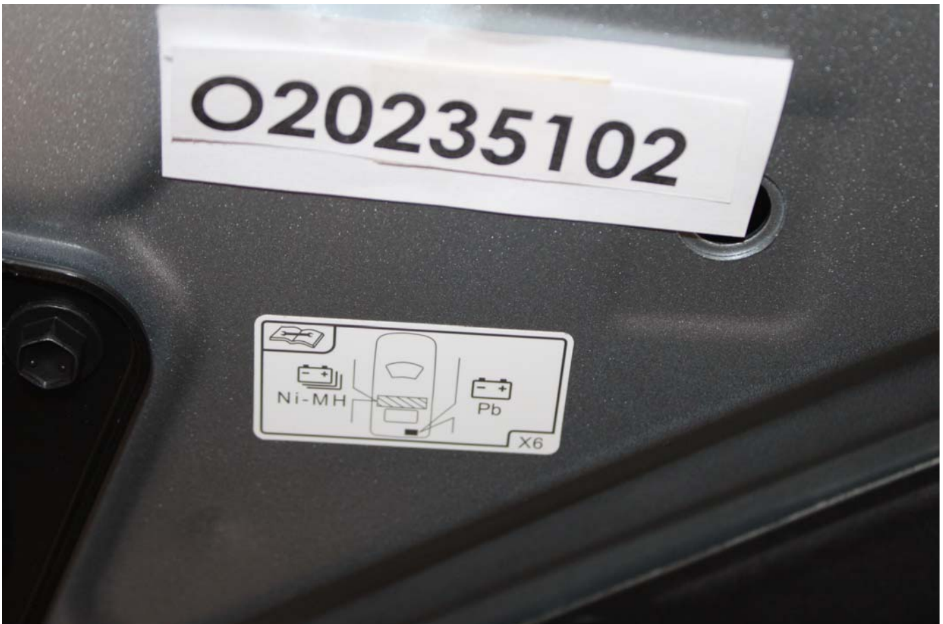
Photo No. 305-03 - First Responder Warning Label
