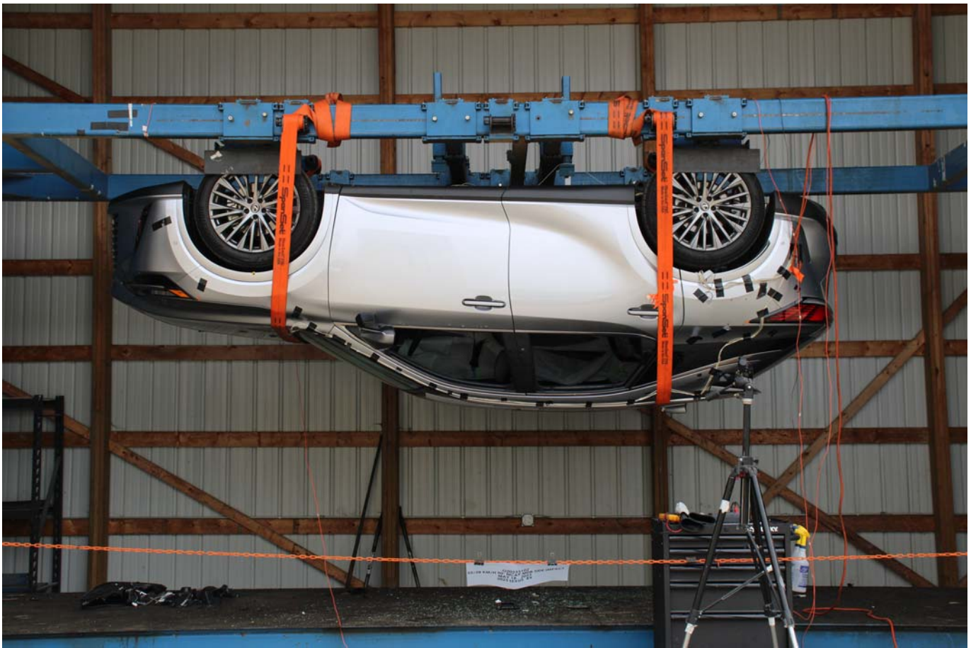
Photo No. 098 - FMVSS Photo No. 301 Static Rollover 180 Degrees
