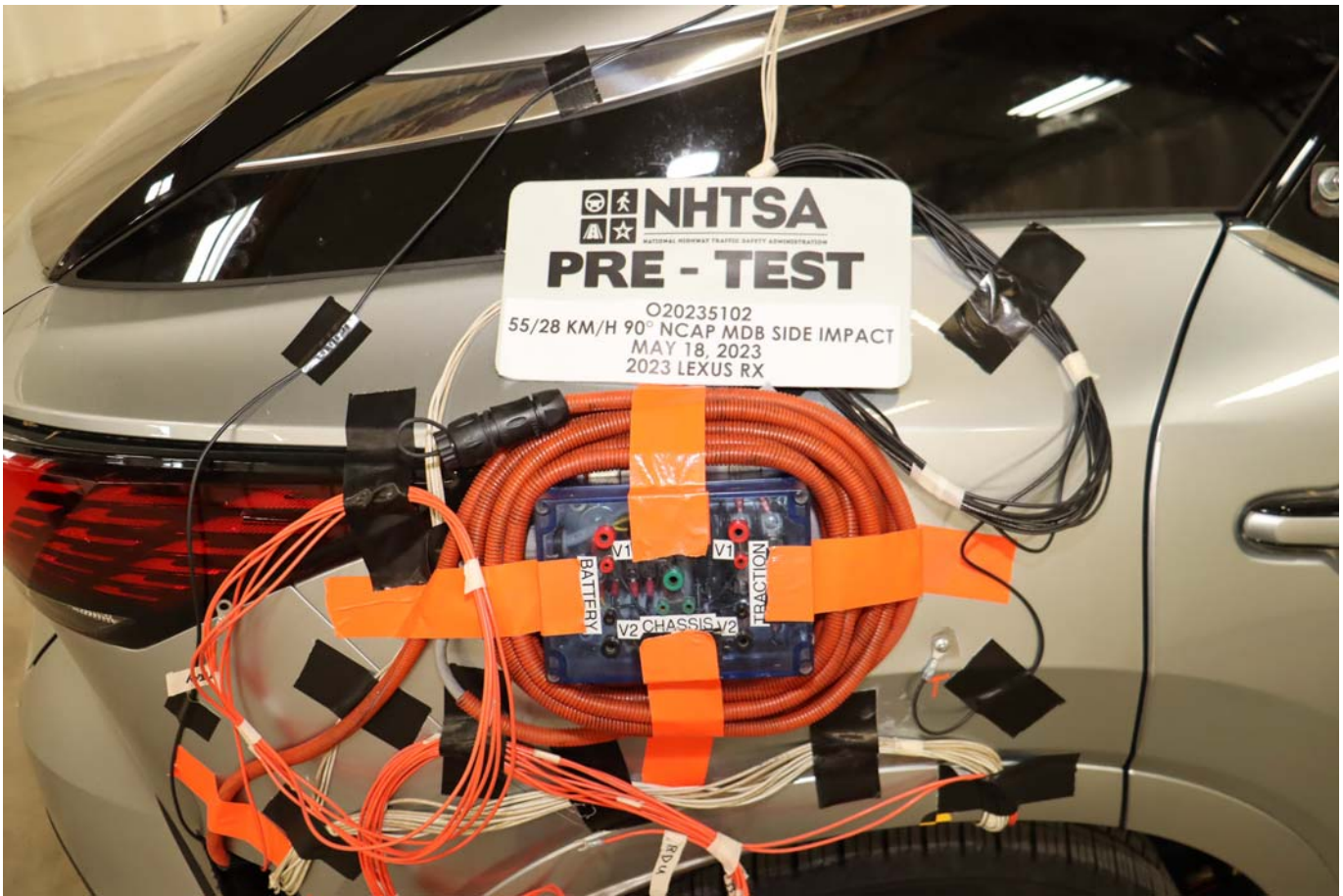
Photo No. 305-24 - Pre-Impact View of Installed Test Interface Port
