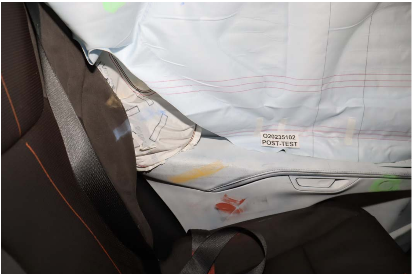
Photo No. 078 - Post-Test Rear Passenger Dummy Close-up Torso Contact with Side Airbag View
